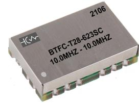
The BTFC module outputs a 1PPS signal and a digitally synthesized 3.3V LVCMOS clock output at frequencies from 152Hz to 80 MHz. In addition, the module can generate up to 2 additional clean clock outputs at a variety of frequencies from 160MHz to <1KHz. The generated frequency outputs are both phase and frequency locked to the incoming 1PPS reference signal.
