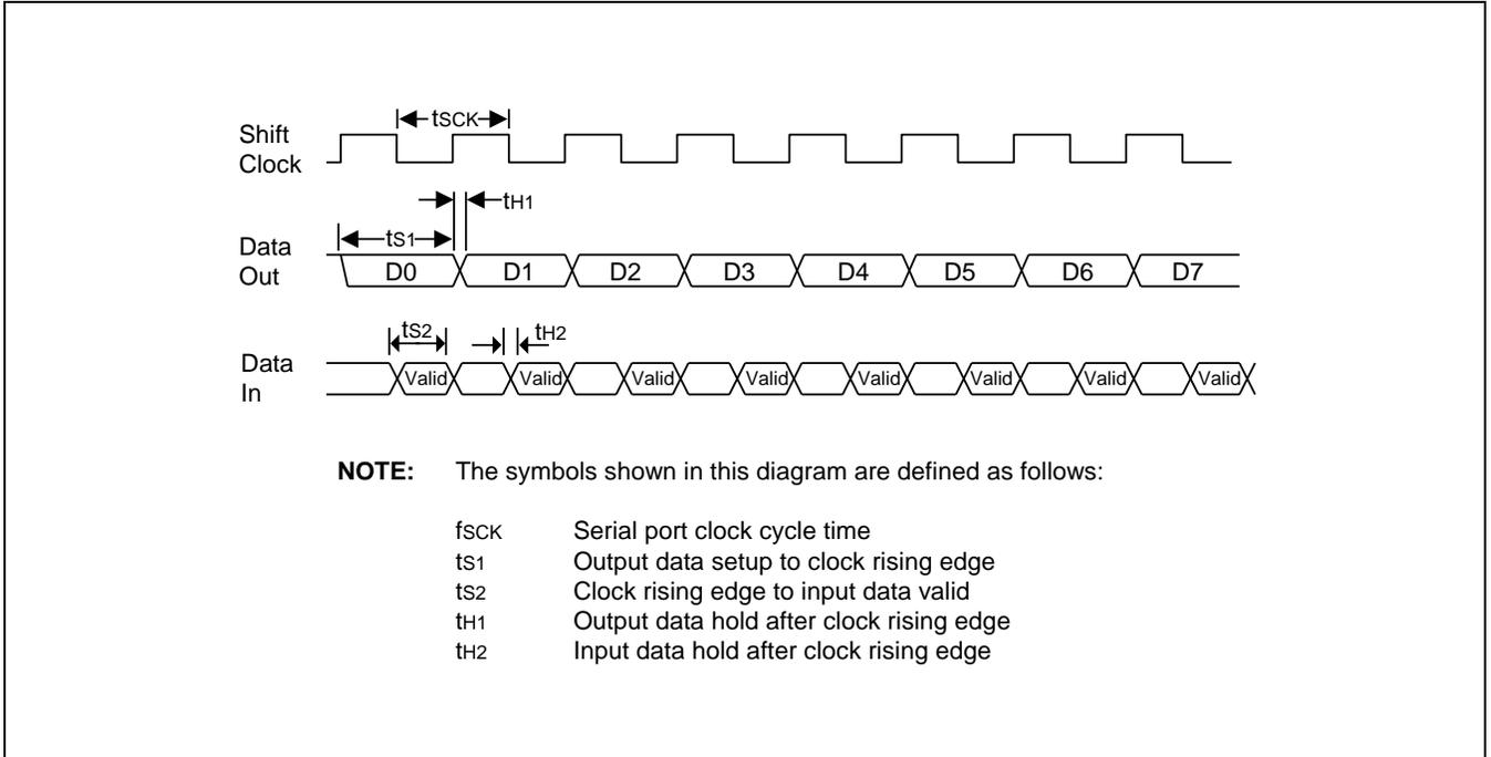
Figure 22-8 Timing Waveform for the UART Module
