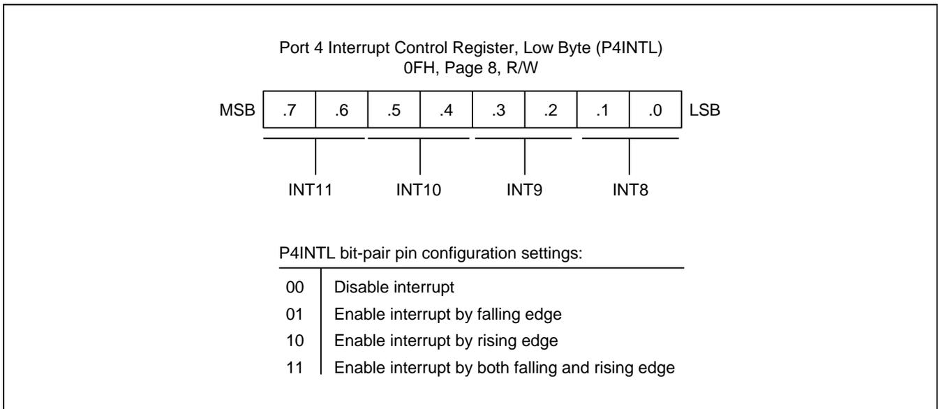
**Figure 9-21 Port 4 Low-Byte Interrupt Control Register (P4INTL)**
