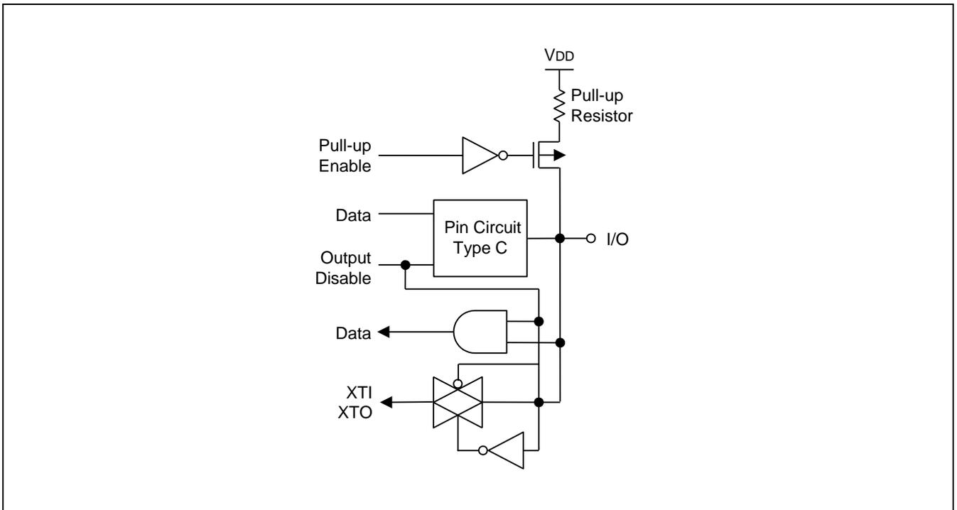
**Figure 1-7 Pin Circuit Type D-2 (P5.6 – P5.7)**
