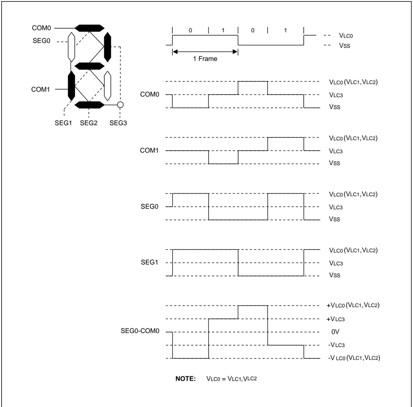
Figure 15-11 LCD Signal Waveforms (1/2 Duty, 1/2 Bias)
