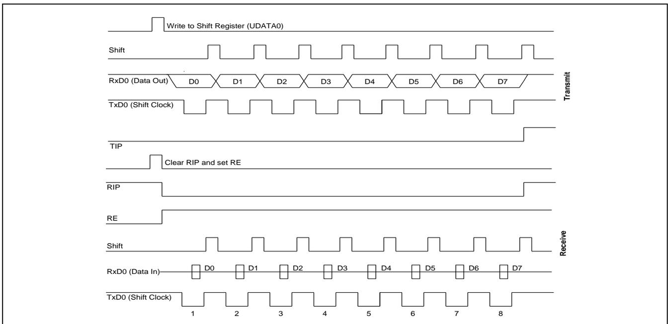
Figure 18-6 Timing Diagram for Serial Port Mode 0 Operation
