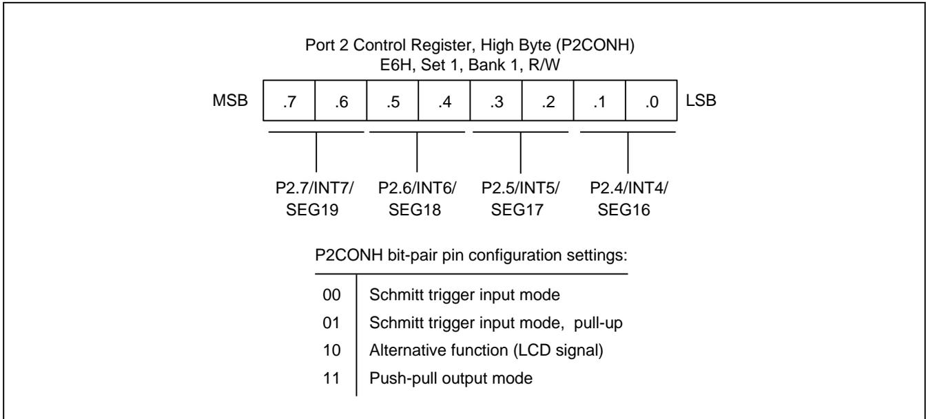
**Figure 9-8 Port 2 High-Byte Control Register (P2CONH)**
