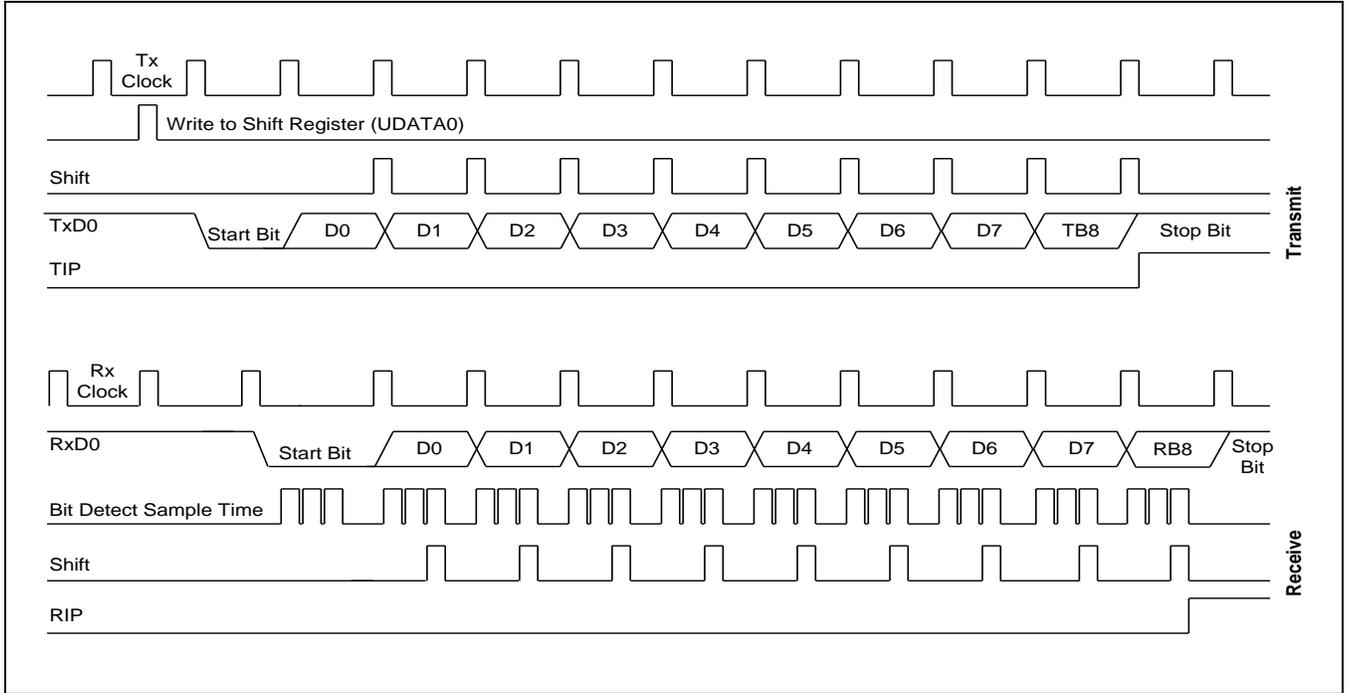
**Figure 18-8 Timing Diagram for Serial Port Mode 2 Operation**
