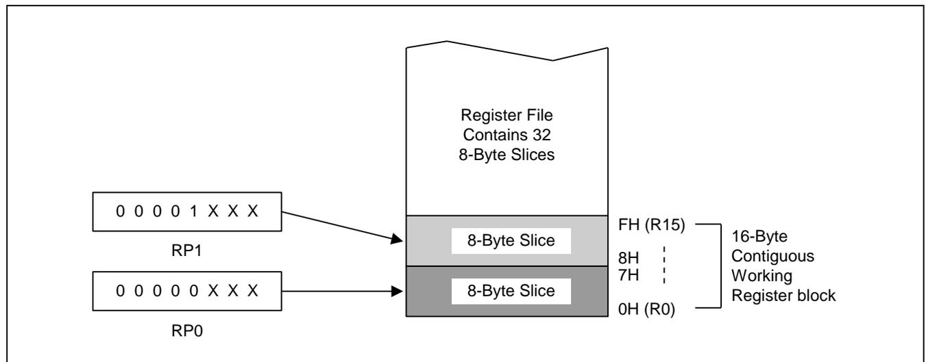
Figure 2-7 Contiguous 16 byte Working Register Block
