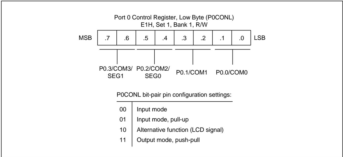
**Figure 9-3 Port 0 Low-Byte Control Register (P0CONL)**
