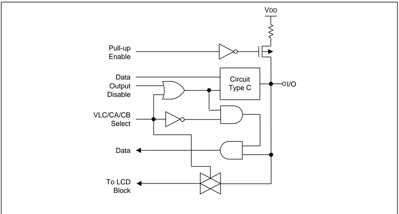
**Figure 1-9 Pin Circuit Type F-17 (P5.0 - P5.5)**
