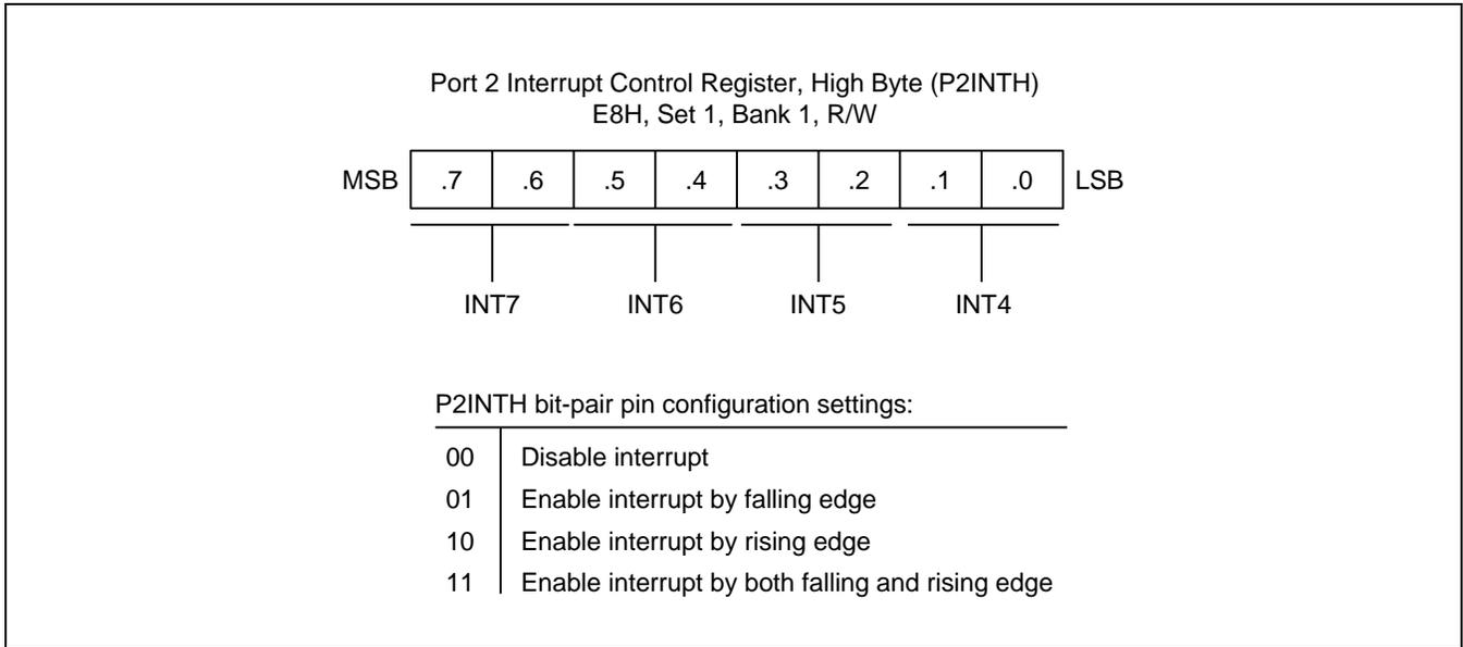
**Figure 9-10 Port 2 High-Byte Interrupt Control Register (P2INTH)**
