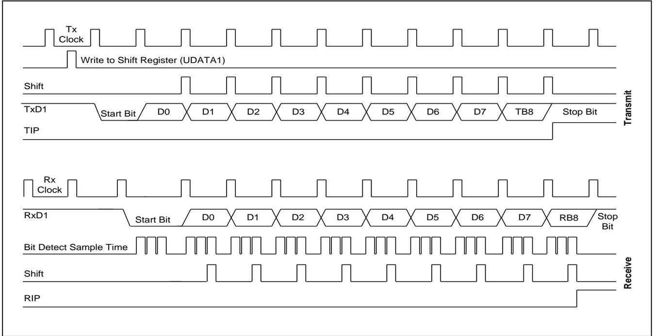
**Figure 19-8 Timing Diagram for Serial Port Mode 2 Operation**
