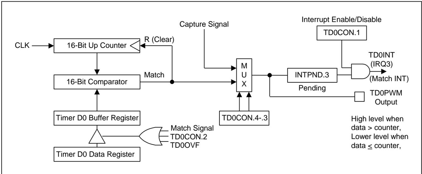
Figure 13-3 Simplified Timer D0 Function Diagram: PWM Mode
