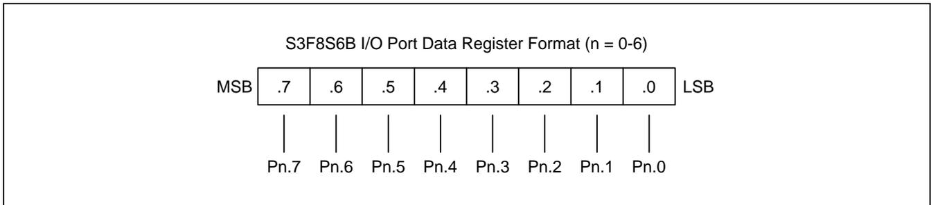
**Figure 9-1 S3F8S6B I/O Port Data Register Format**
