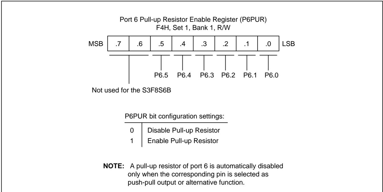
**Figure 9-27 Port 6 Pull-up Resistor Enable Register (P6PUR)**
