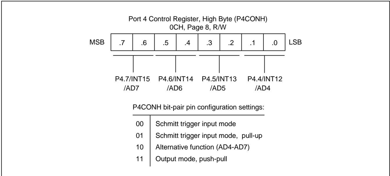
**Figure 9-18 Port 4 High-Byte Control Register (P4CONH)**
