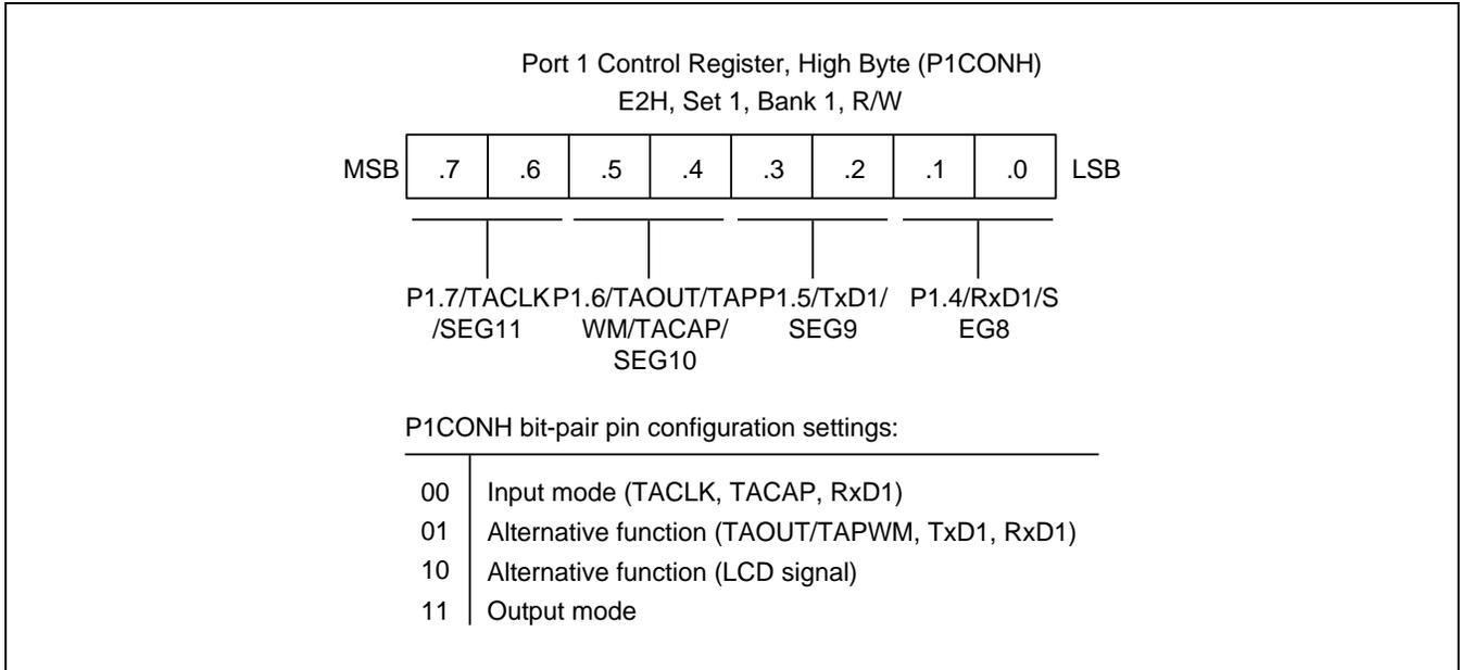
**Figure 9-4 Port 1 High-Byte Control Register (P1CONH)**
