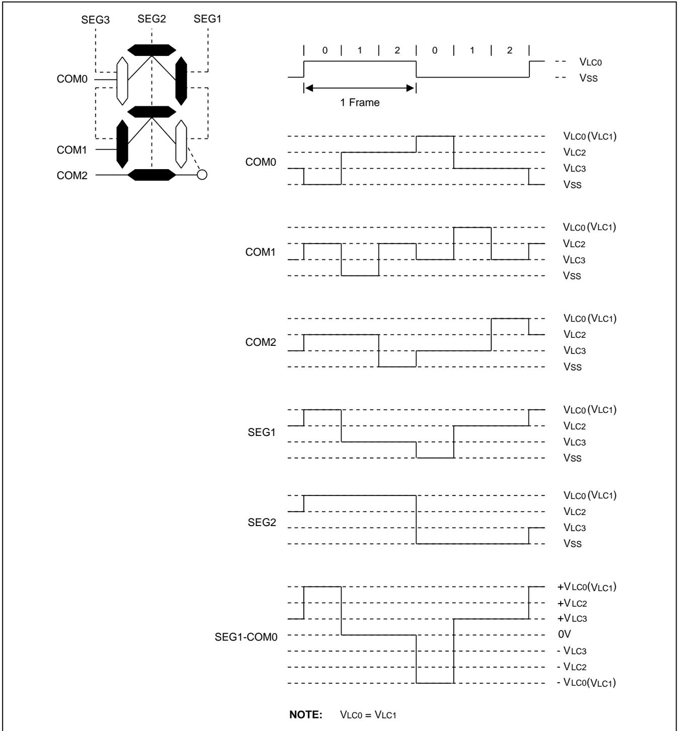
Figure 15-12 LCD Signal Waveforms (1/3 Duty, 1/3 Bias)
