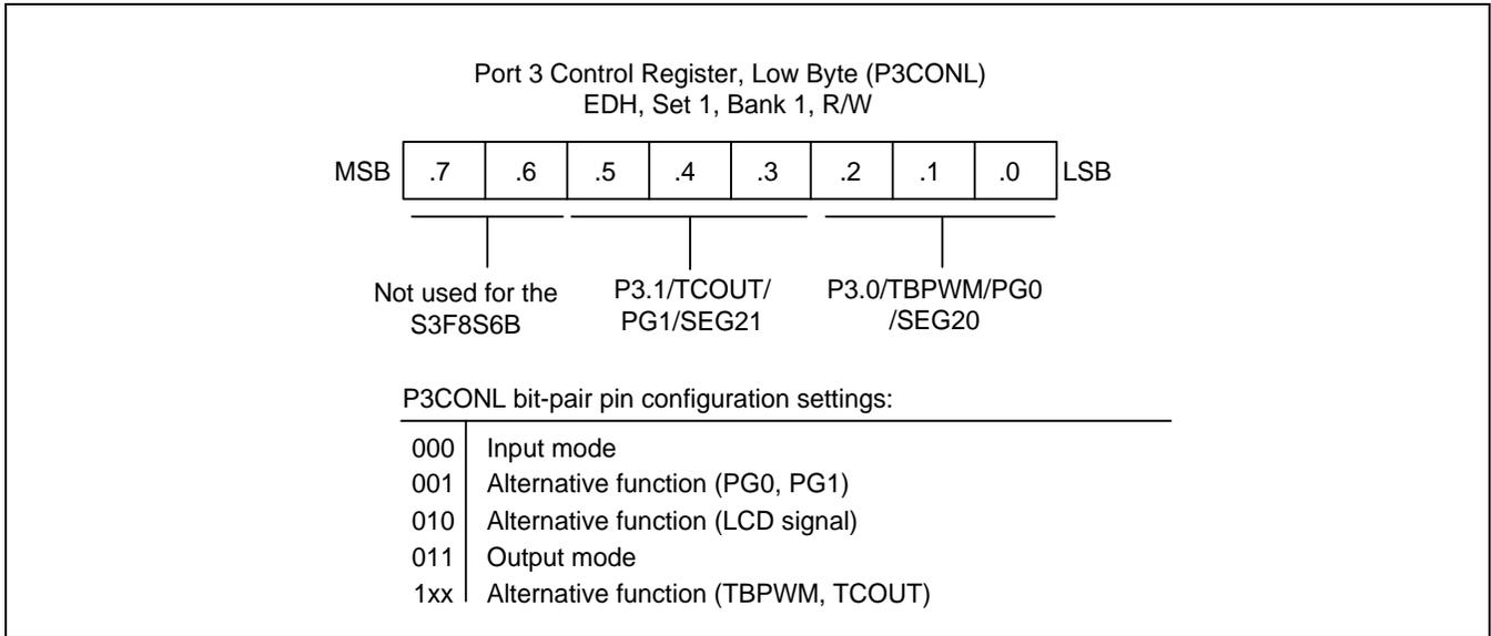
**Figure 9-15 Port 3 Low-Byte Control Register (P3CONL)**
