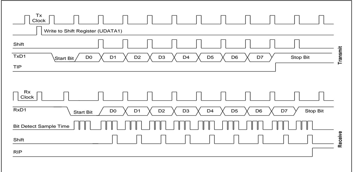
**Figure 19-7 Timing Diagram for Serial Port Mode 1 Operation**
