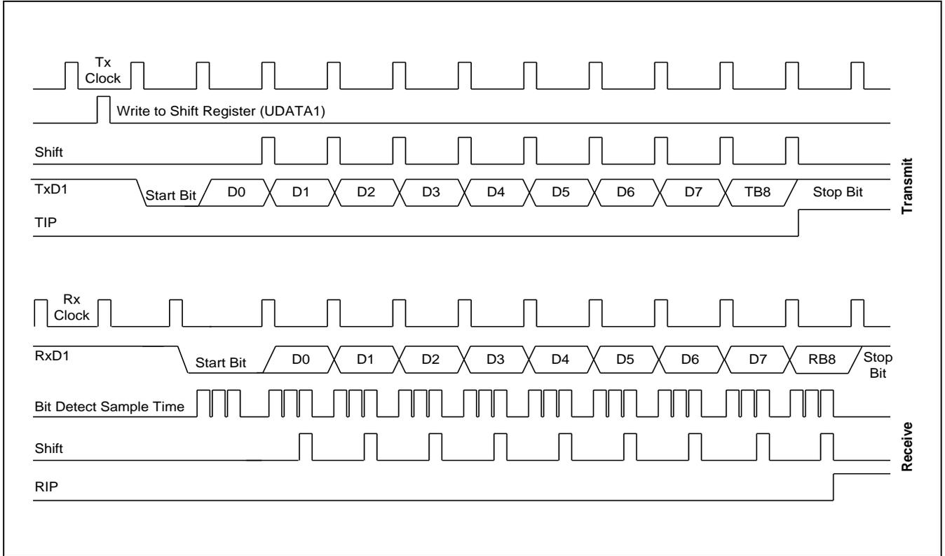
**Figure 19-9 Timing Diagram for Serial Port Mode 3 Operation**
