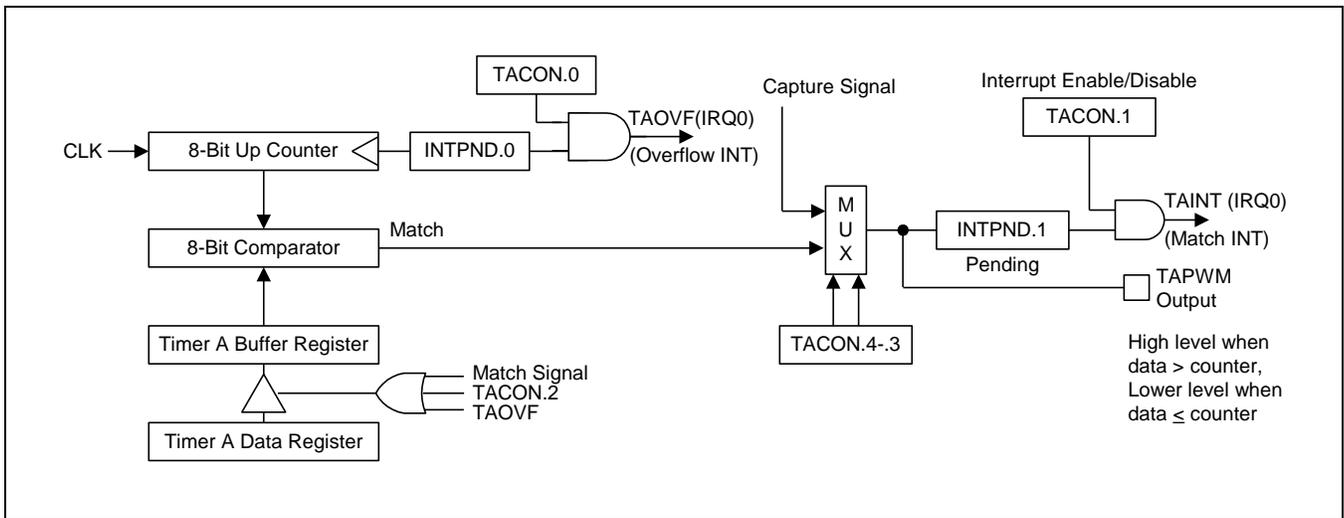
Figure 11-3 Simplified Timer A Function Diagram: PWM Mode
