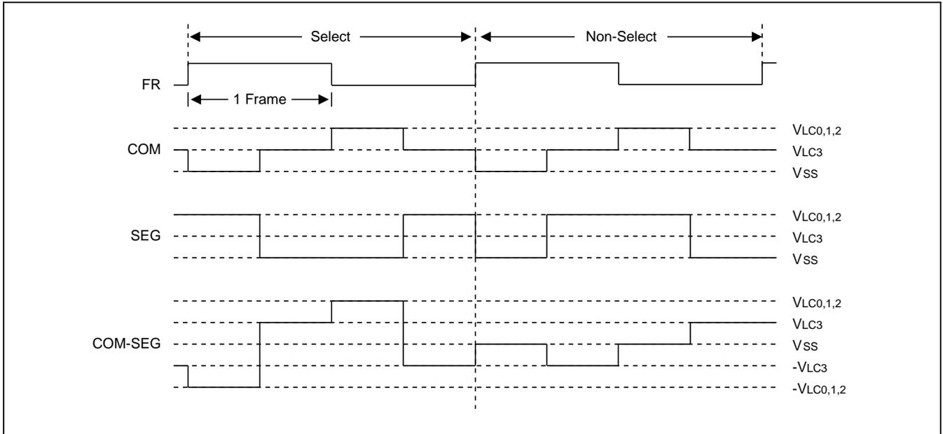
**Figure 15-9 Select/No-Select Signal in 1/2 Duty, 1/2 Bias Display Mode**
