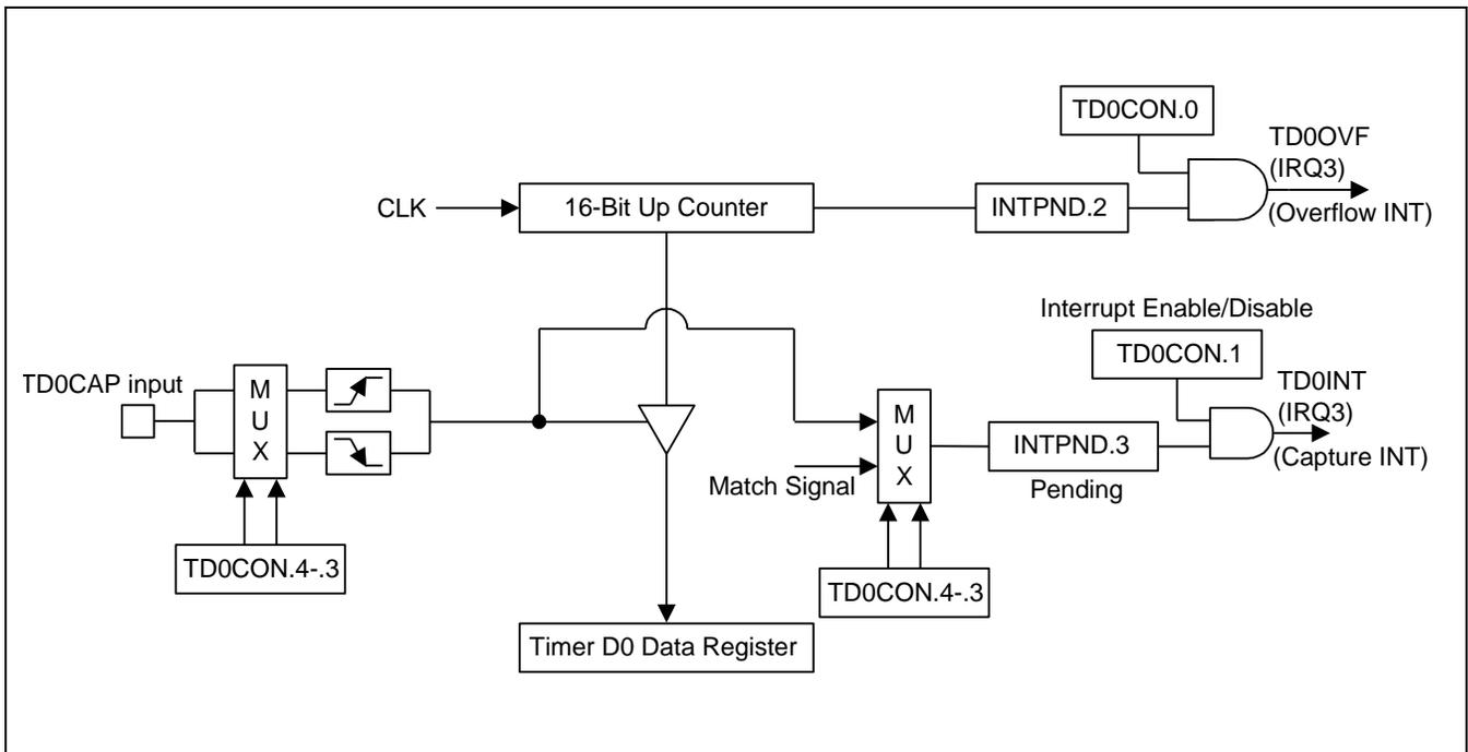
Figure 13-4 Simplified Timer D0 Function Diagram: Capture Mode
