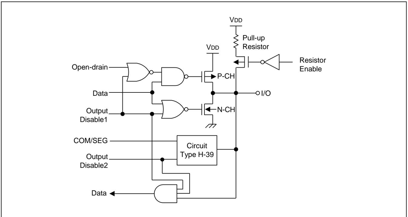
Figure 1-13 Pin Circuit Type H-42 (P1, P3, P6)
