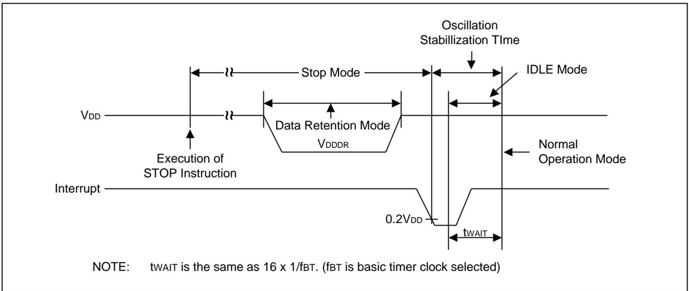
**Figure 22-4 Stop Mode Release Timing Initiated by Interrupts**
