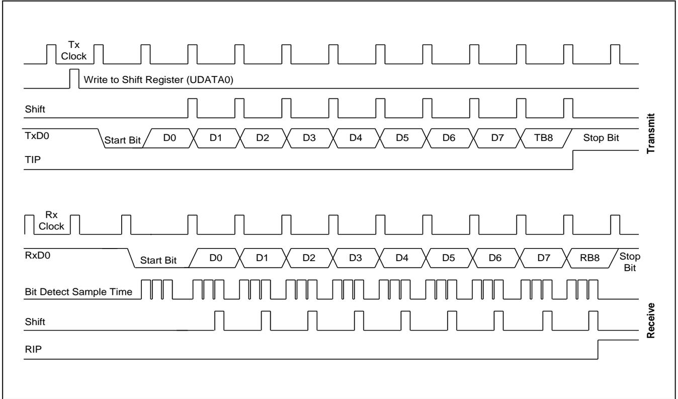
**Figure 18-9 Timing Diagram for Serial Port Mode 3 Operation**
