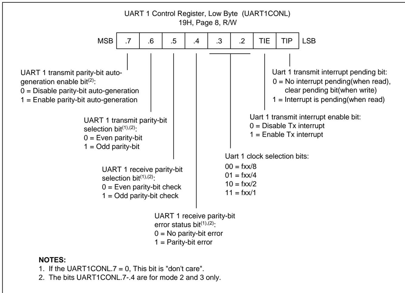
Figure 19-2 UART 1 Low Byte Control Register (UART1CONL)
