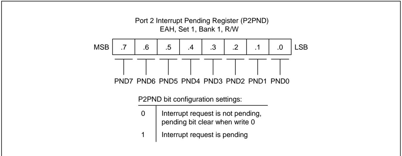
**Figure 9-12 Port 2 Interrupt Pending Register (P2PND)**
