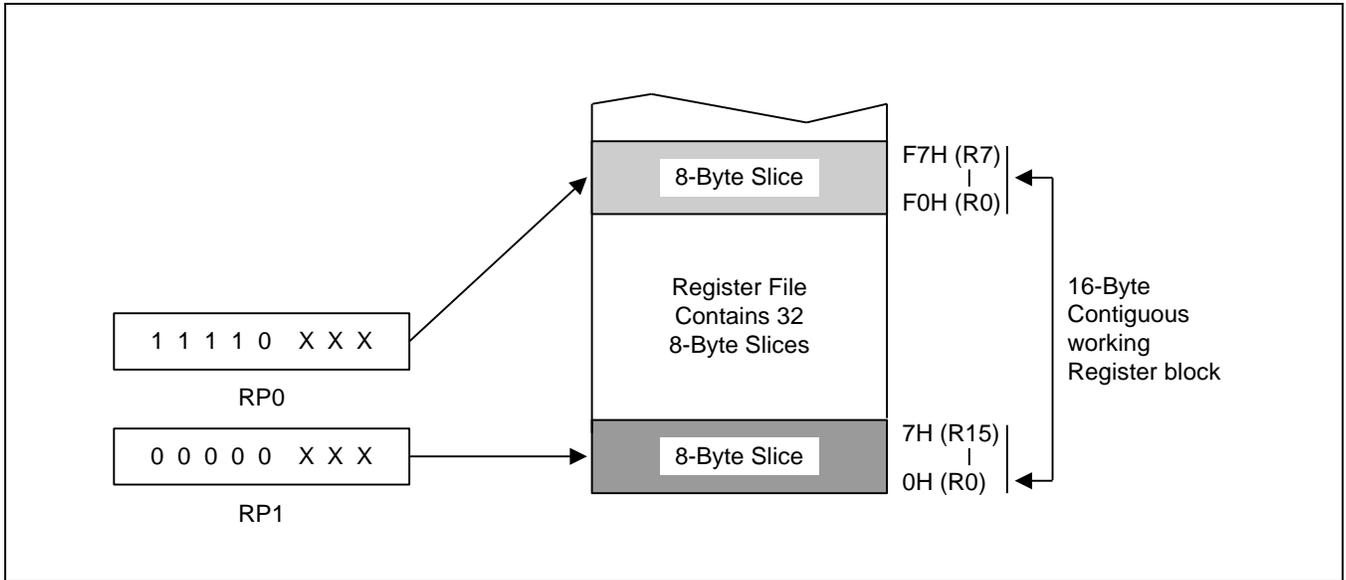
Figure 2-8 Non-Contiguous 16 byte Working Register Block
