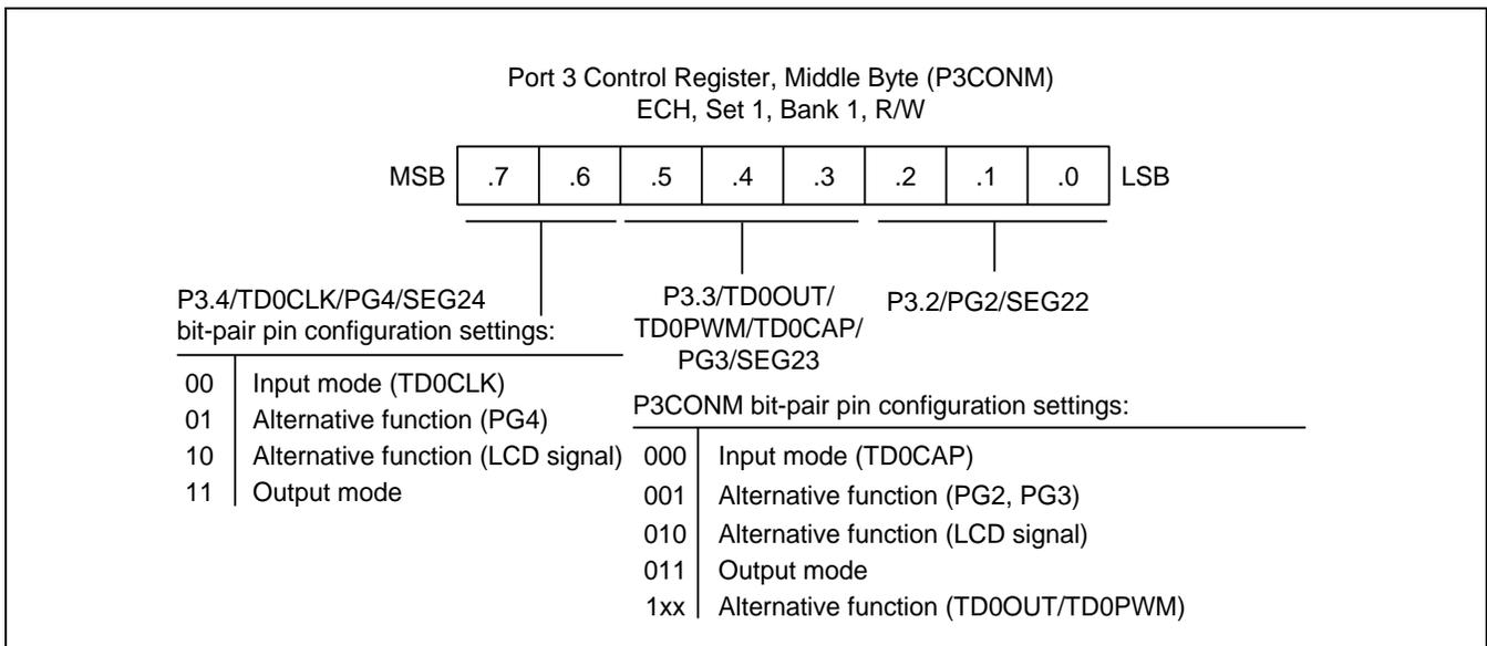
**Figure 9-14 Port 3 Middle-Byte Control Register (P3CONM)**
