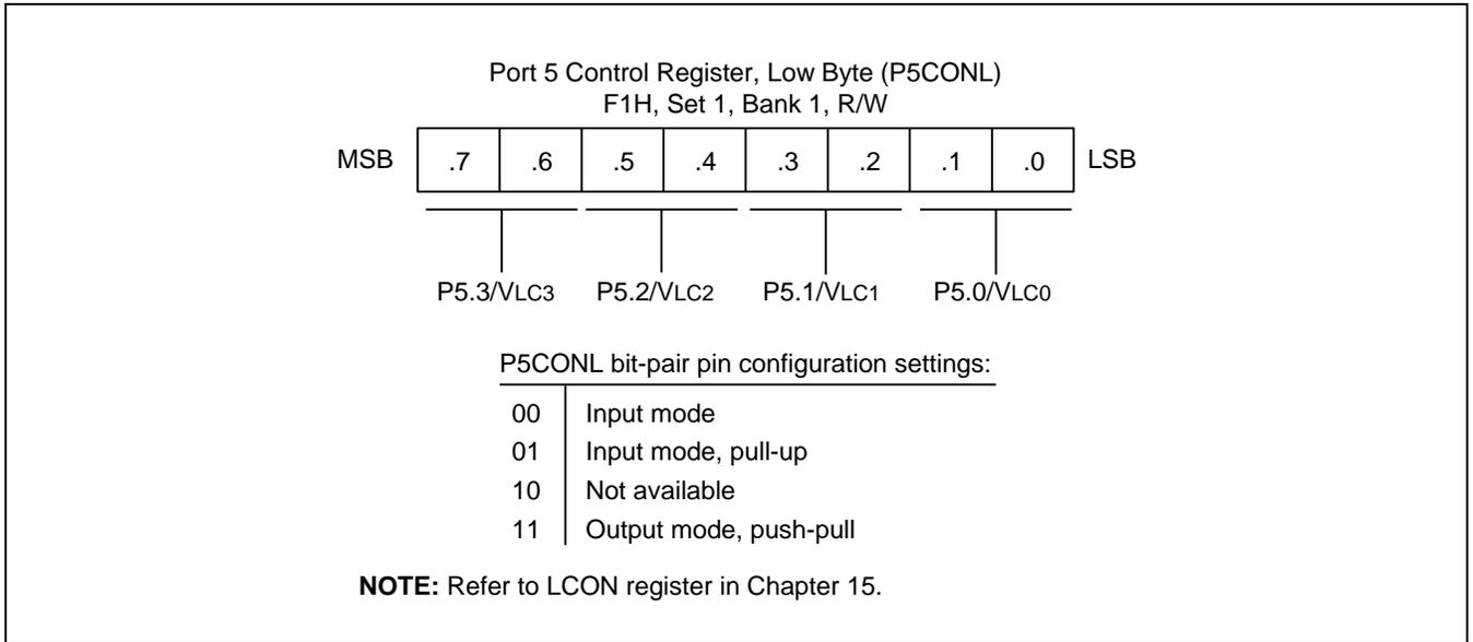
**Figure 9-24 Port 5 Low-Byte Control Register (P5CONL)**
