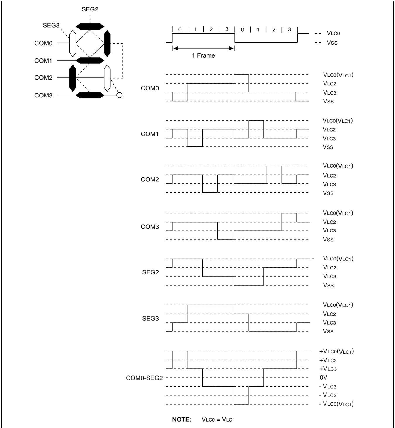
Figure 15-13 LCD Signal Waveforms (1/4 Duty, 1/3 Bias)
