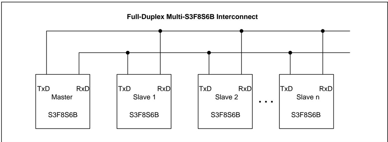
**Figure 18-10 Connection Example for Multiprocessor Serial Data Communications**
