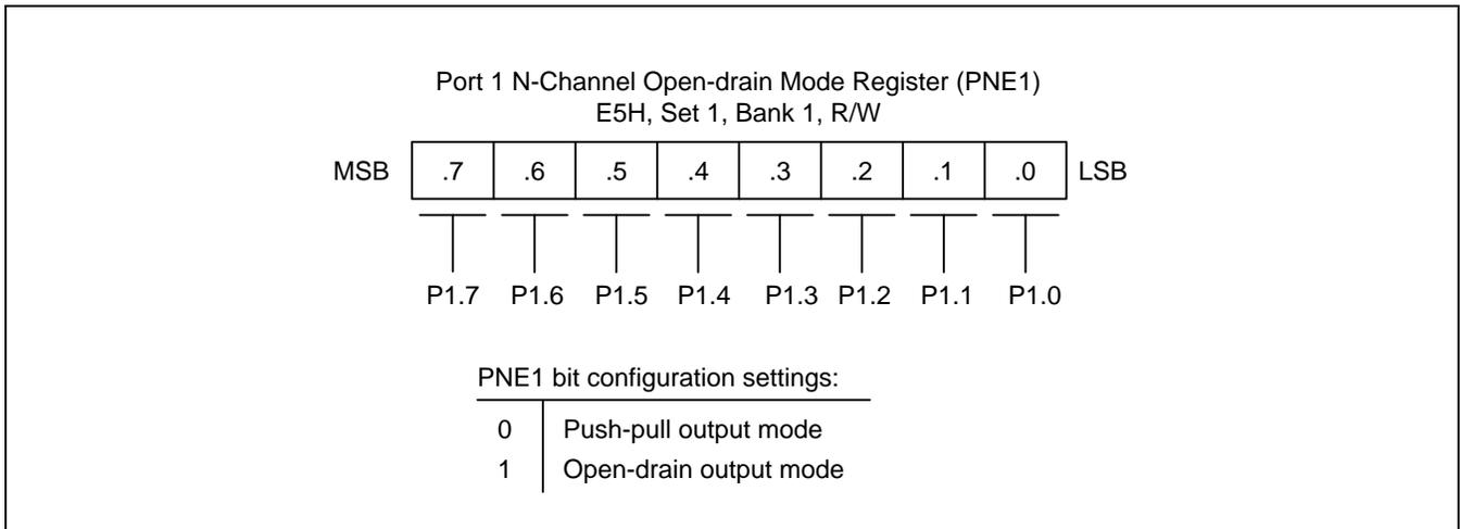
**Figure 9-7 Port 1 N-Channel Open-drain Mode Register (PNE1)**
