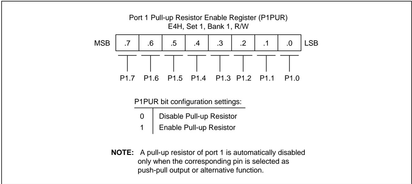
**Figure 9-6 Port 1 Pull-up Resistor Enable Register (P1PUR)**
