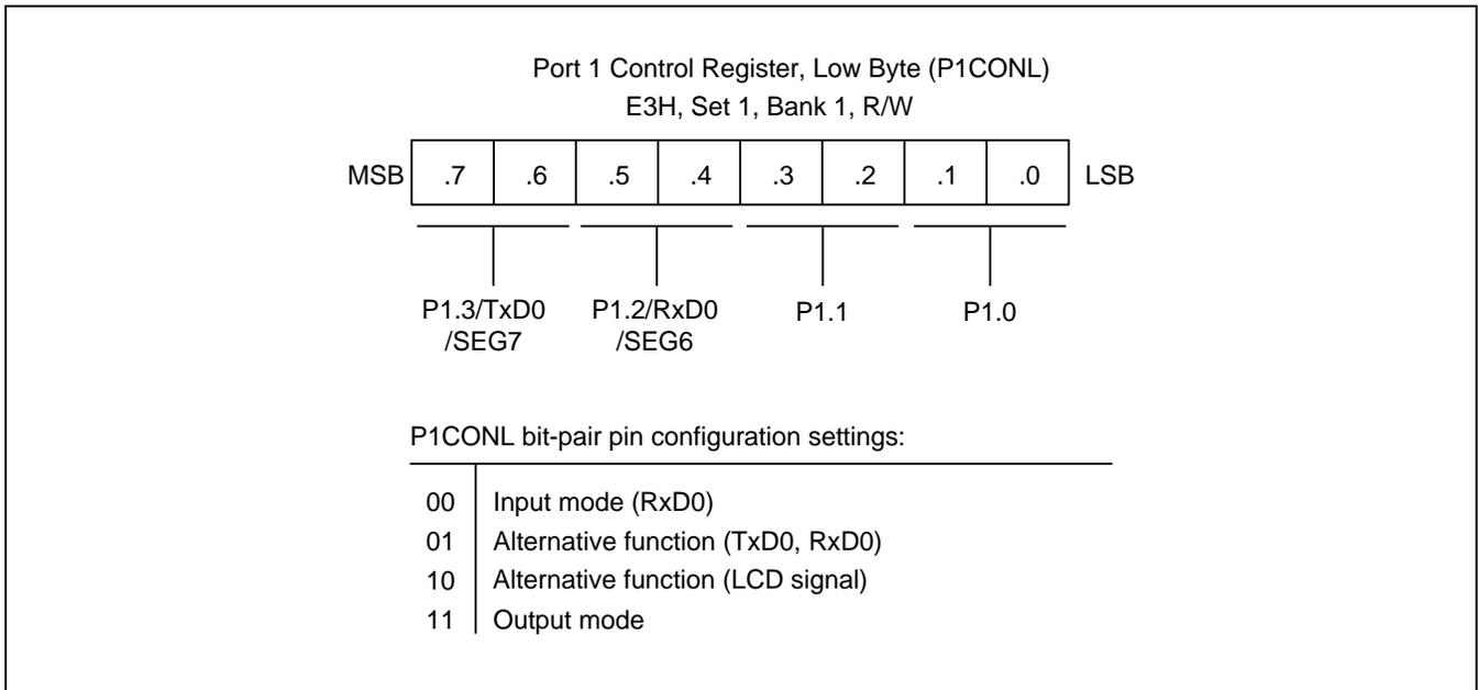
**Figure 9-5 Port 1 Low-Byte Control Register (P1CONL)**
