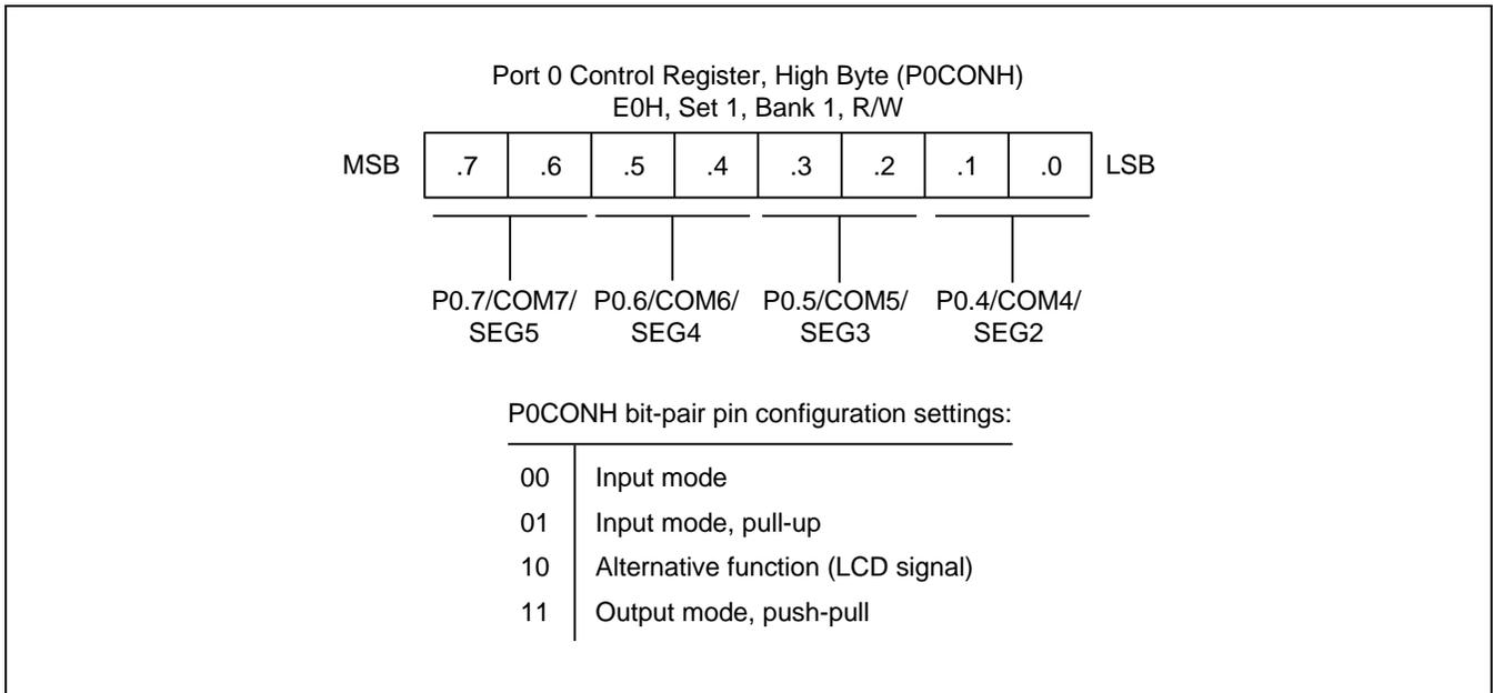
**Figure 9-2 Port 0 High-Byte Control Register (P0CONH)**
