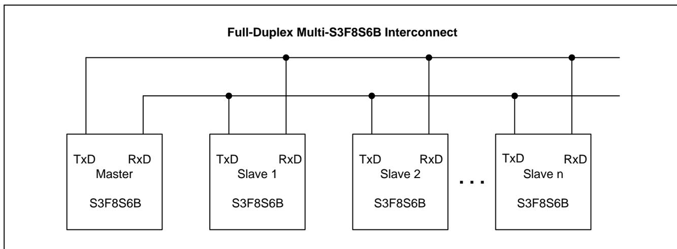
**Figure 19-10 Connection Example for Multiprocessor Serial Data Communications**
