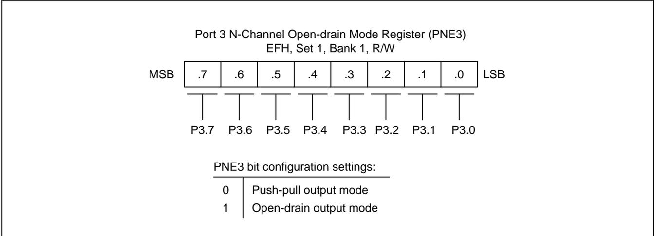
**Figure 9-17 Port 3 N-Channel Open-Drain Mode Register (PNE3)**
