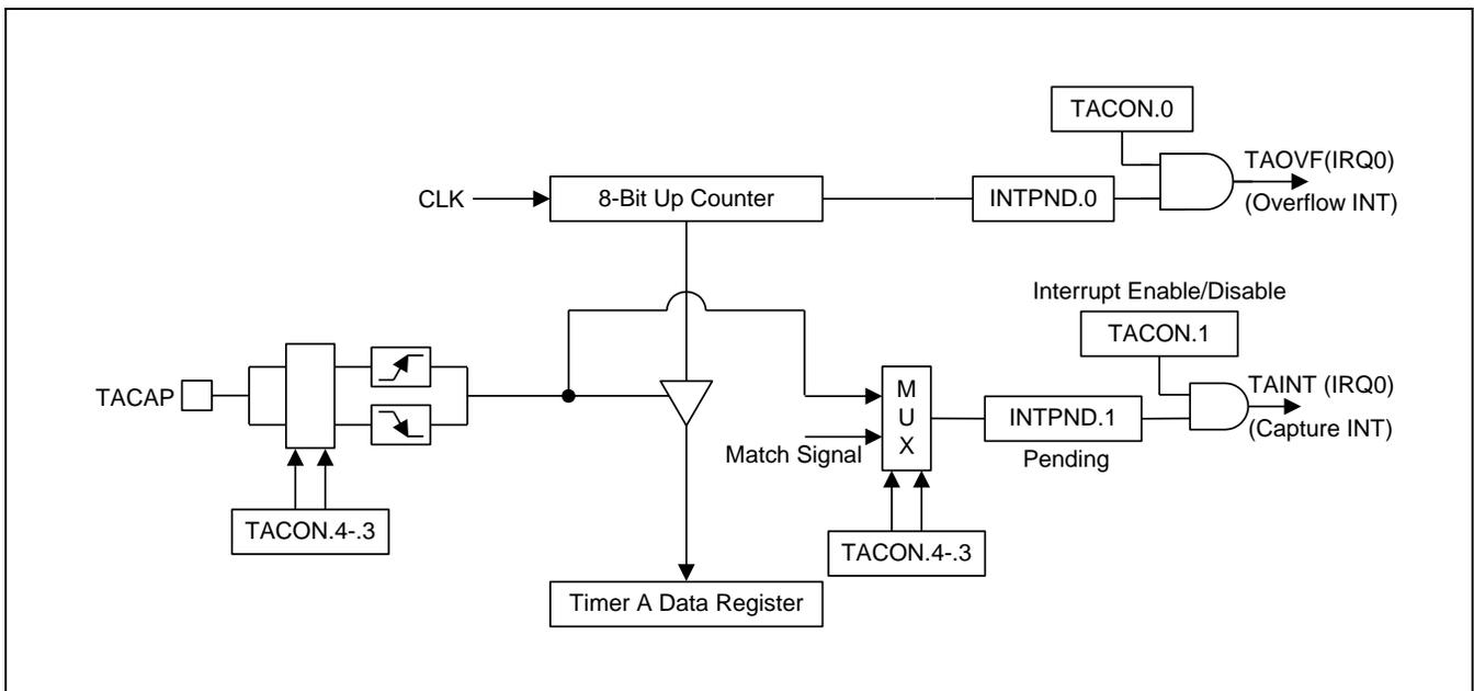
Figure 11-4 Simplified Timer A Function Diagram: Capture Mode
