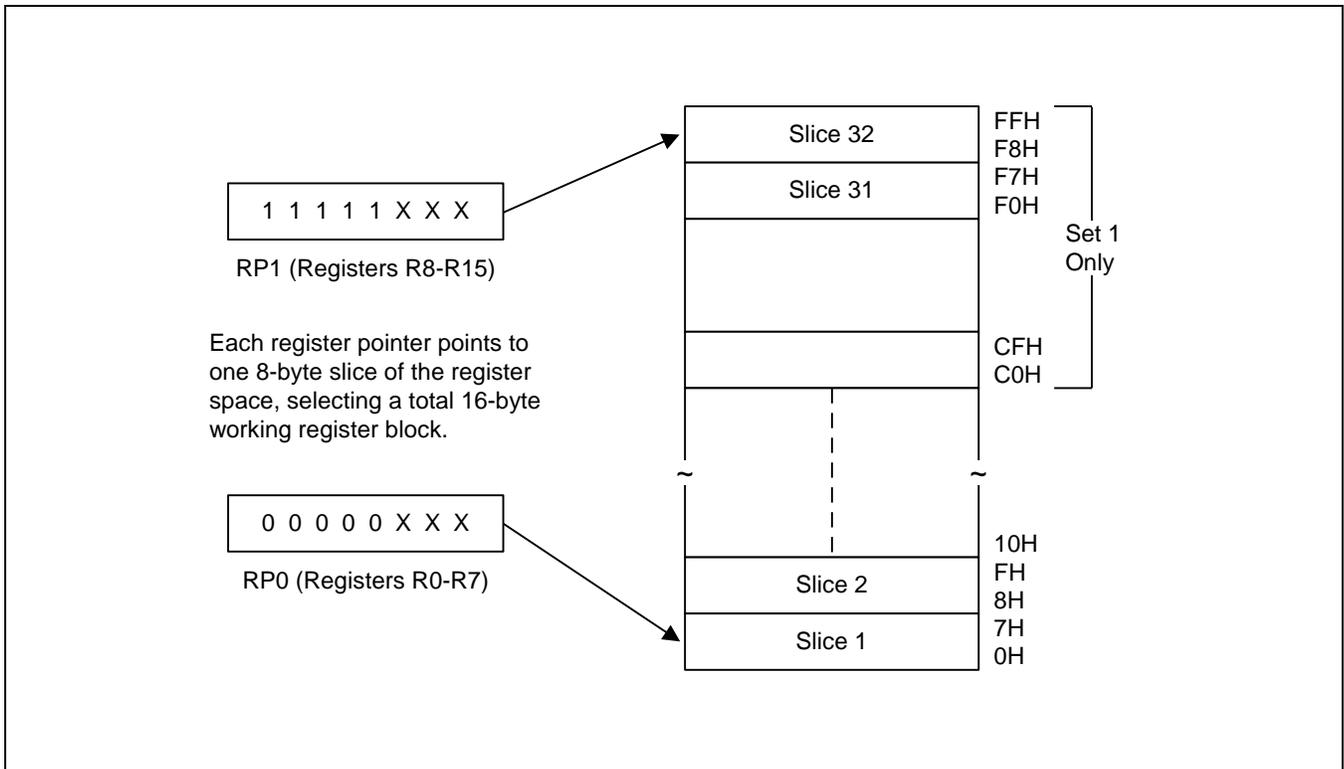
Figure 2-6 8 byte Working Register Areas (Slices)
