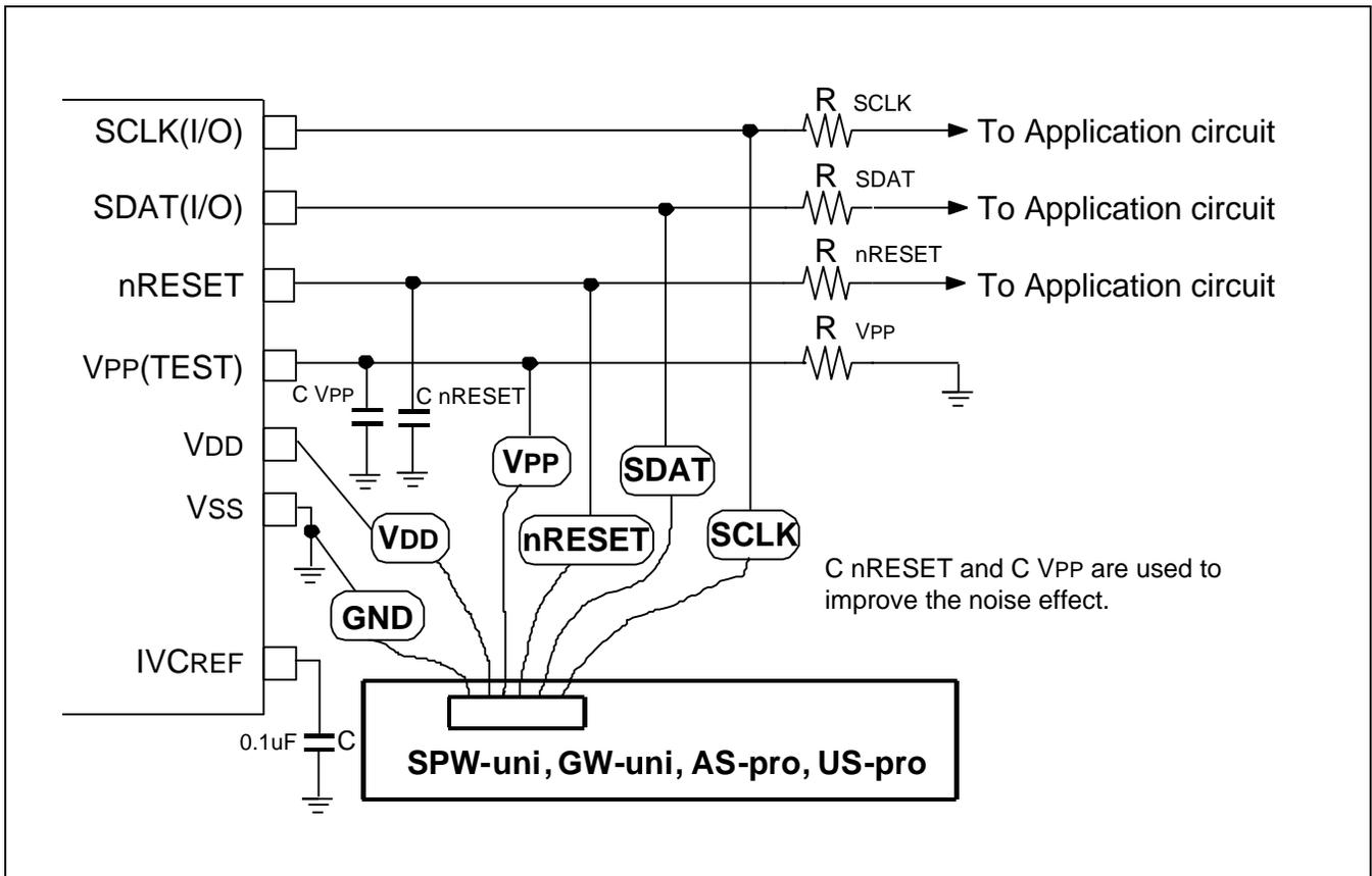
Figure 24-5 PCB Design Guide for on Board Programming
