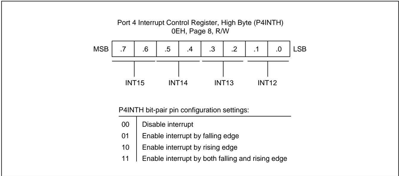
**Figure 9-20 Port 4 High-Byte Interrupt Control Register (P4INTH)**
