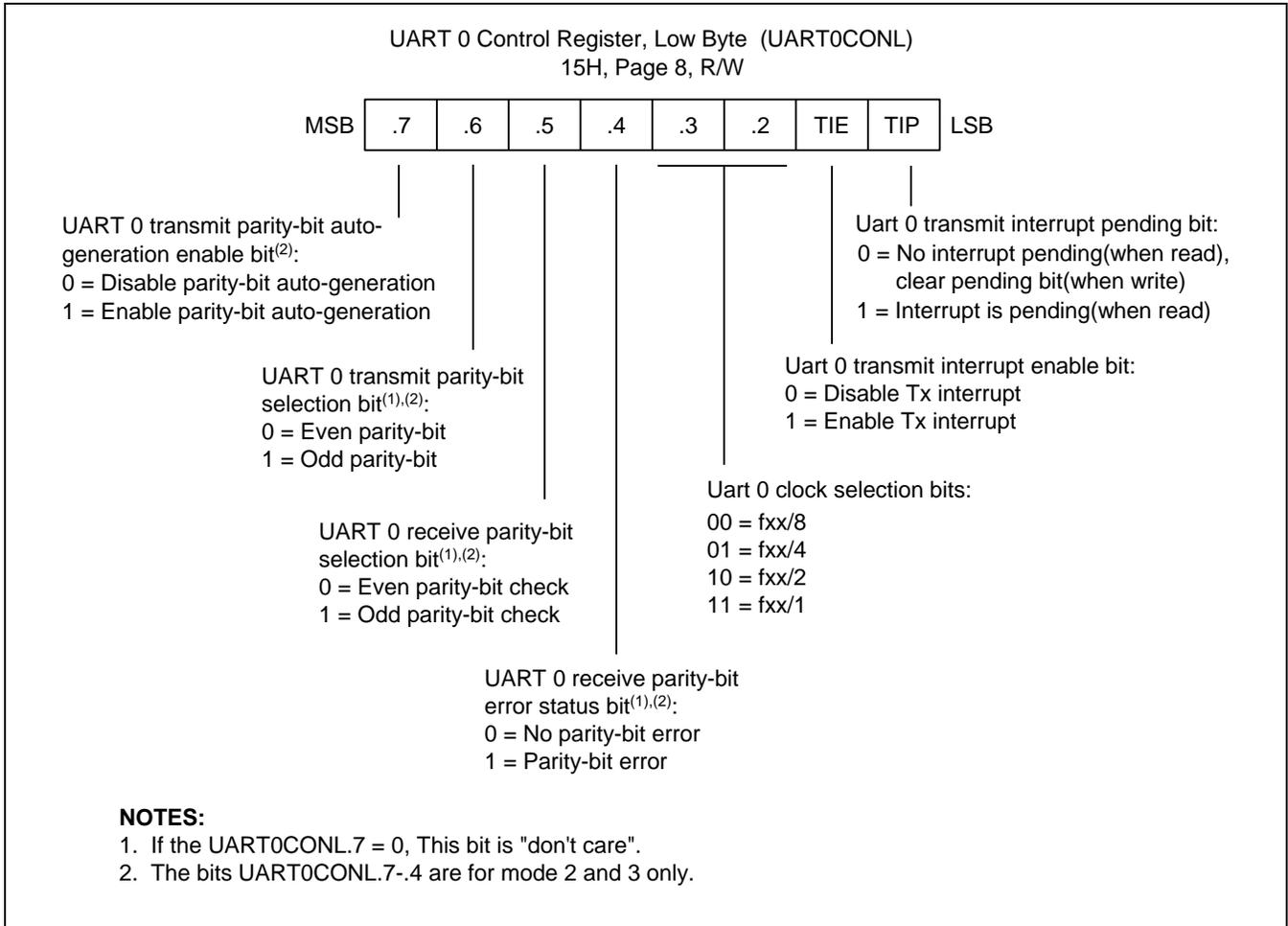
**Figure 18-2 UART 0 Low Byte Control Register (UART0CONL)**
