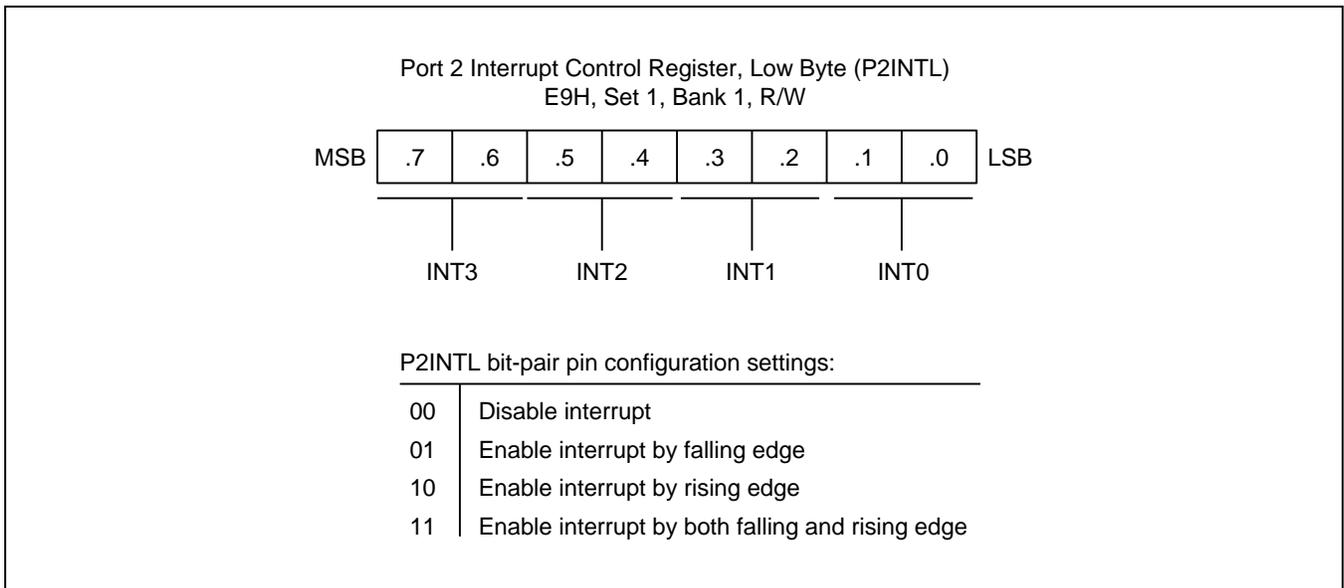
**Figure 9-11 Port 2 Low-Byte Interrupt Control Register (P2INTL)**
