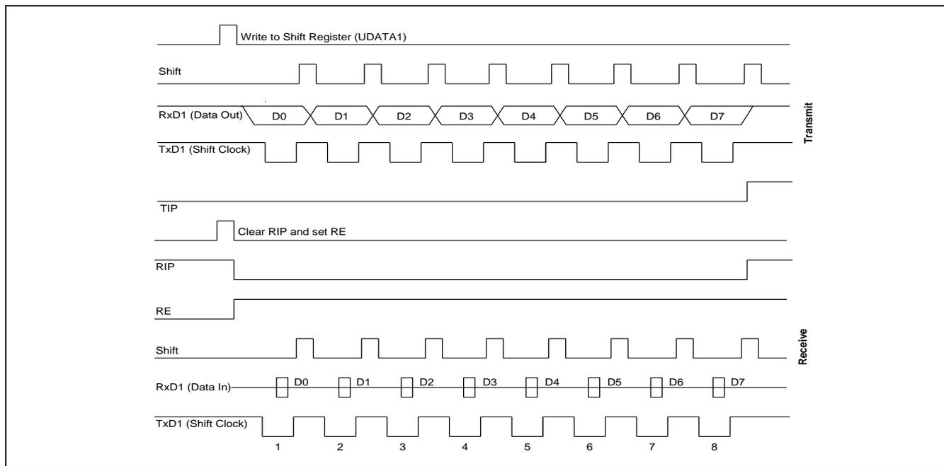
Figure 19-6 Timing Diagram for Serial Port Mode 0 Operation
