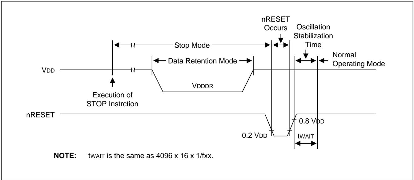
**Figure 22-3 Stop Mode Release Timing Initiated by nRESET**
