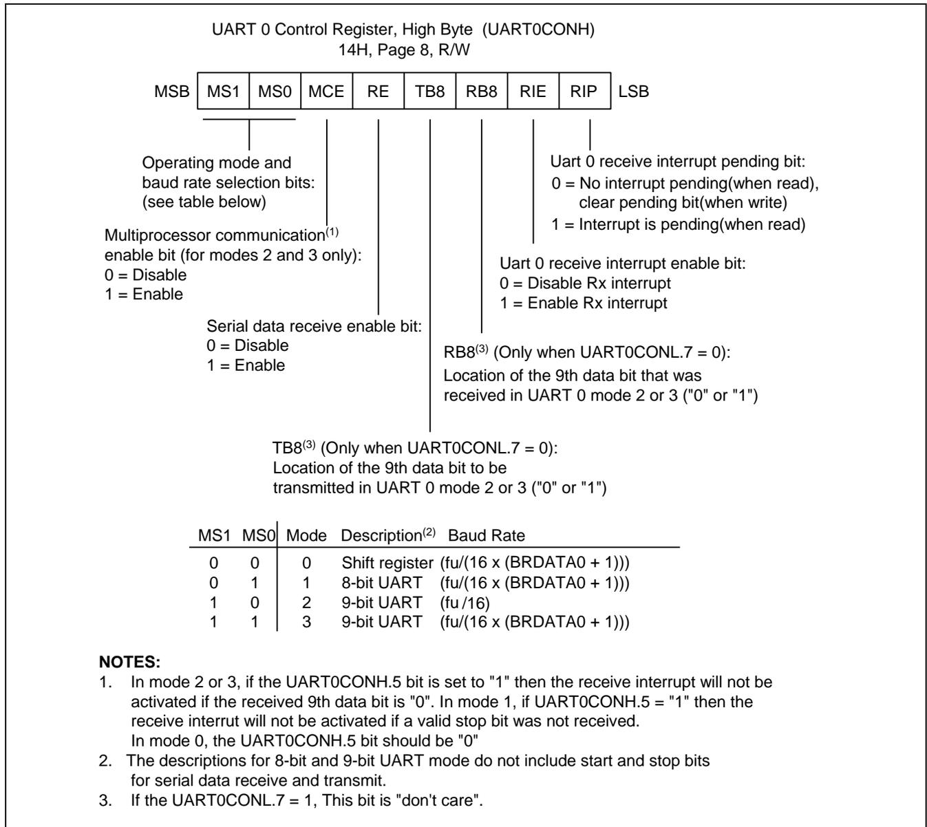
**Figure 18-1 UART 0 High Byte Control Register (UART0CONH)**
