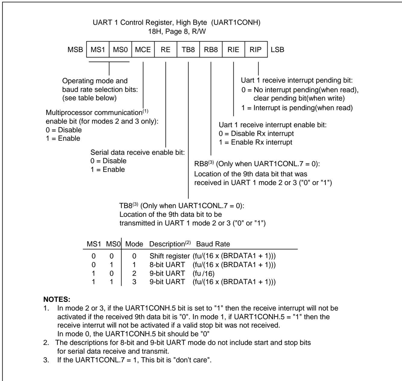
Figure 19-1 UART 1 High Byte Control Register (UART1CONH)
