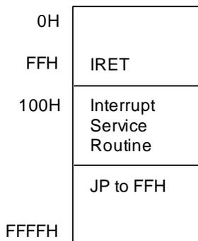
**NOTE:** In the fast interrupt example above, if the last instruction is not a jump to IRET, you must pay attention to the order of the last two instructions. The IRET cannot be immediately preceded by a clearing of the interrupt status (as with a reset of the IPR register).
