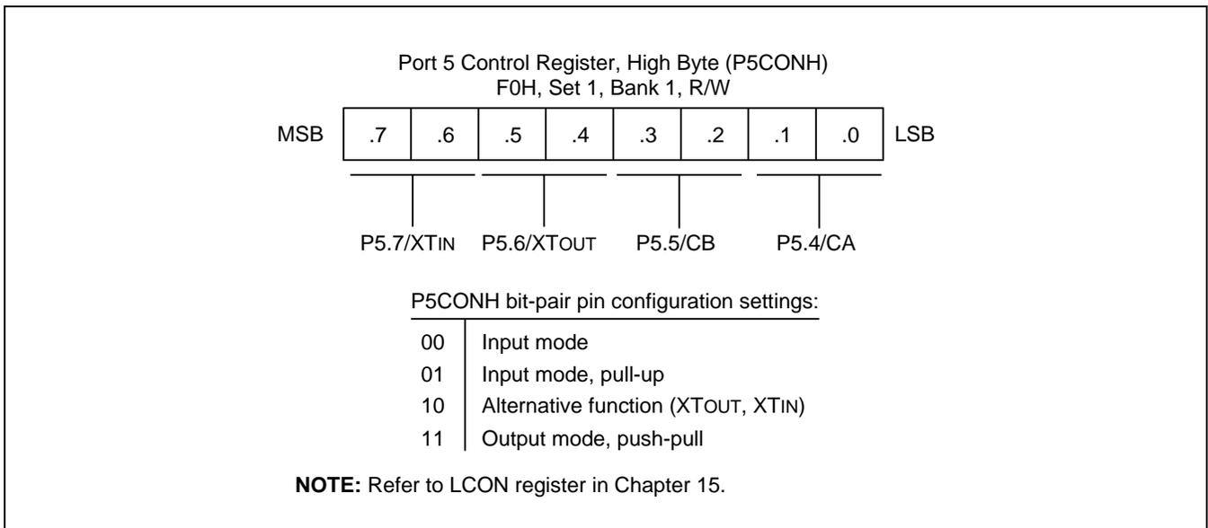
**Figure 9-23 Port 5 High-Byte Control Register (P5CONH)**
