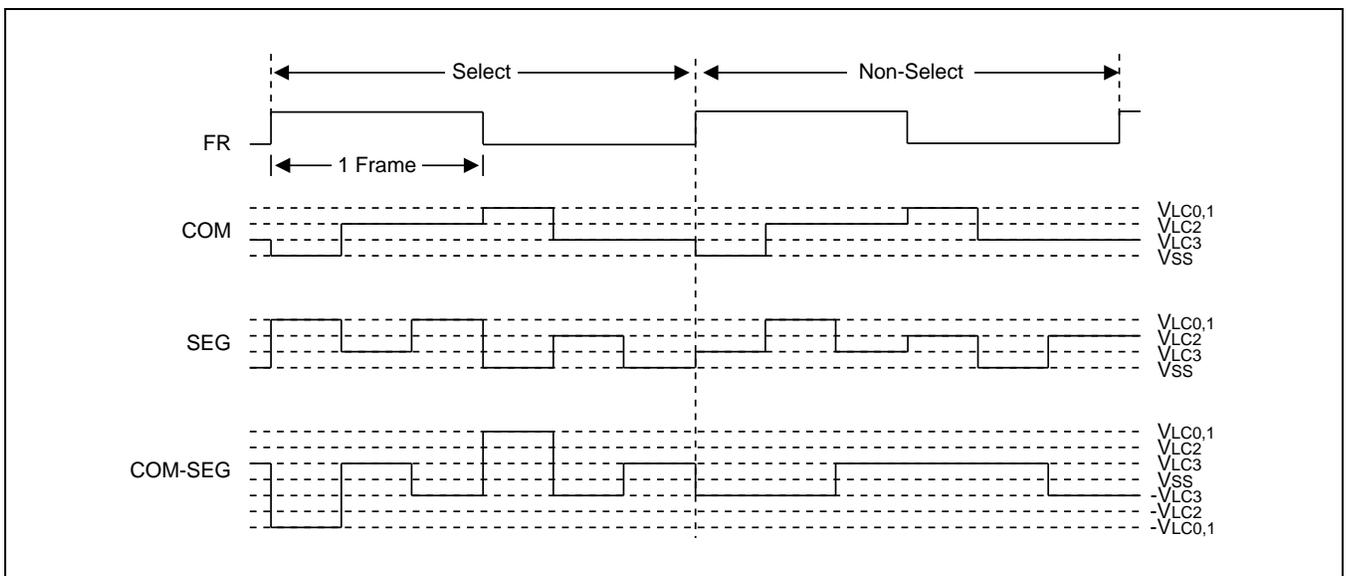
**Figure 15-10 Select/No-Select Signal in 1/3 Duty, 1/3 Bias Display Mode**
