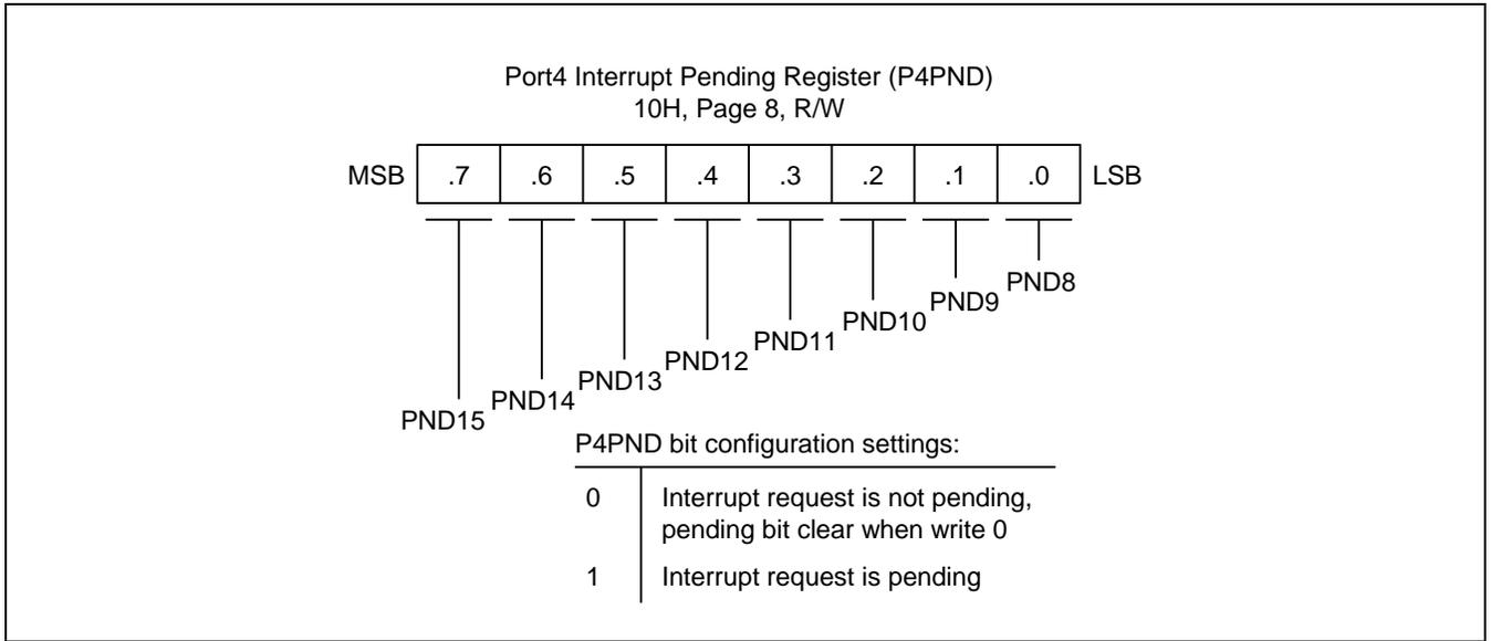
**Figure 9-22 Port 4 Interrupt Pending Register (P4PND)**
