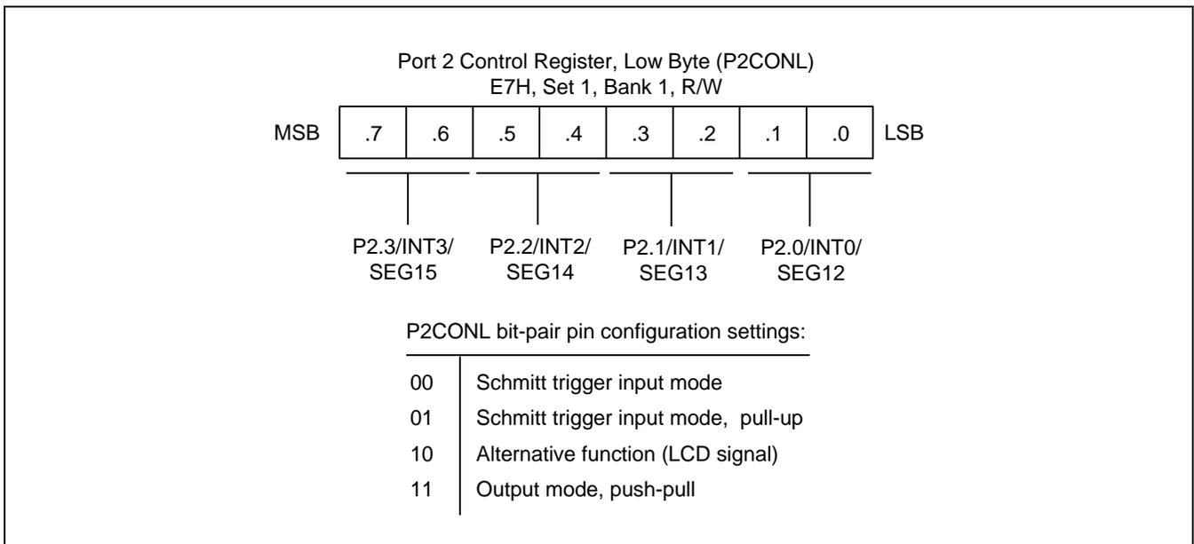
**Figure 9-9 Port 2 Low-Byte Control Register (P2CONL)**
