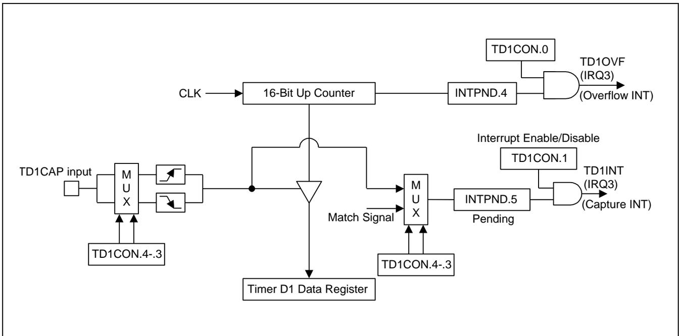
Figure 13-9 Simplified Timer D1 Function Diagram: Capture Mode
