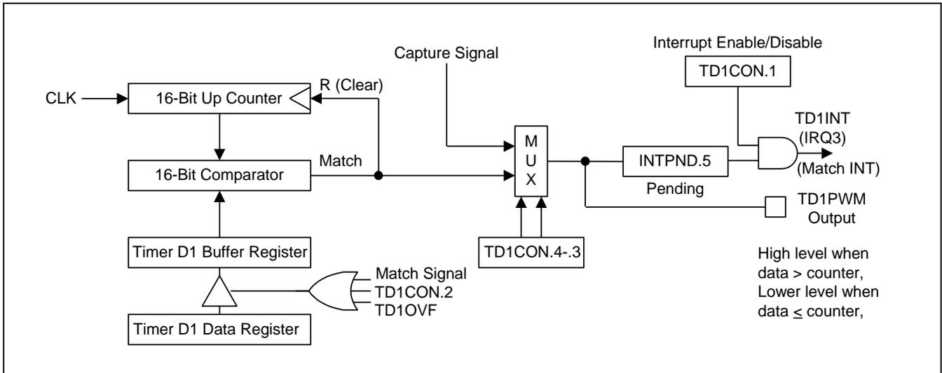
Figure 13-8 Simplified Timer D1 Function Diagram: PWM Mode
