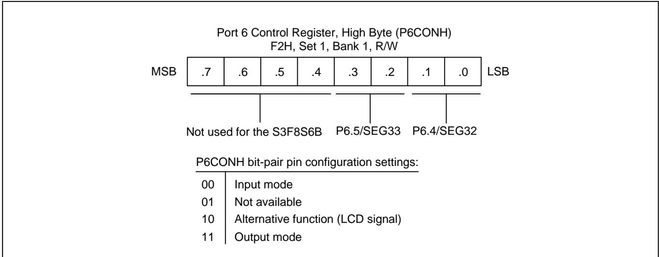
**Figure 9-25 Port 6 High-Byte Control Register (P6CONH)**
