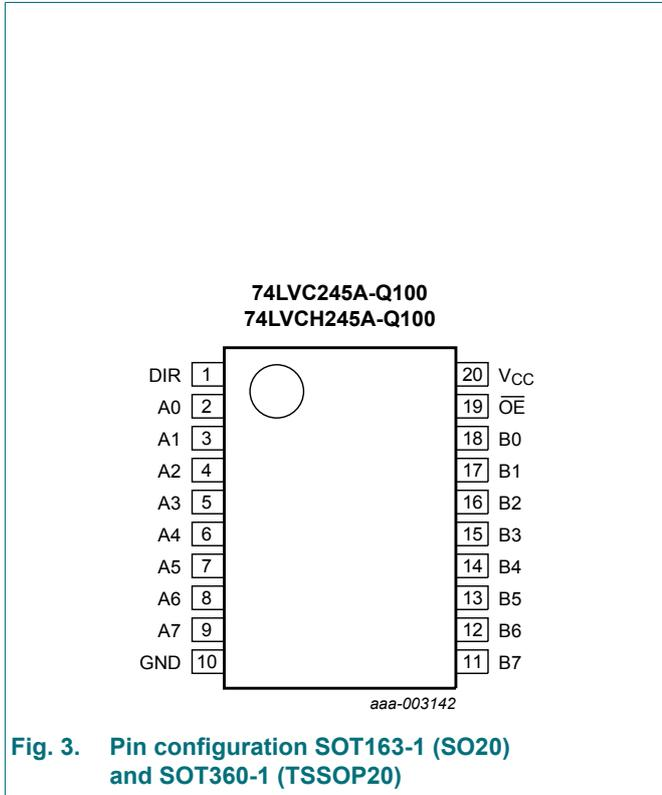
Fig. 3. Pin configuration SOT163-1 (SO20) and SOT360-1 (TSSOP20)
