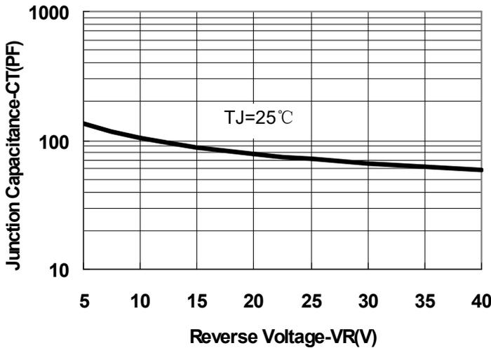
Fig.1-Typical Junction Capacitance
