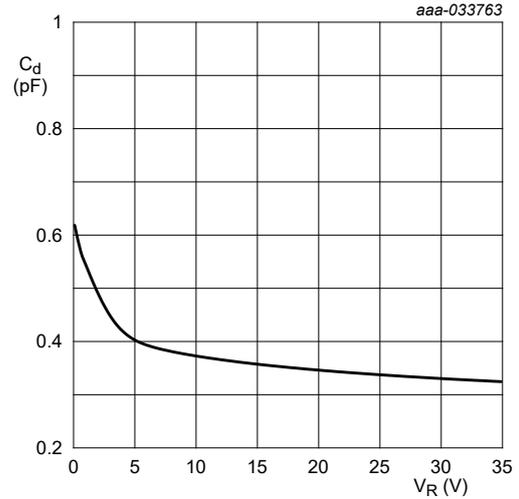
$f = 1\text{ MHz}; T_{\text{amb}} = 25^\circ\text{C}$
