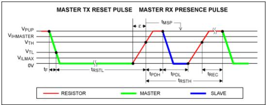
Figure 1. Reset and presence pulse.
