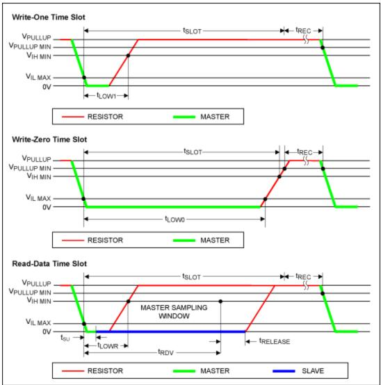
Figure 5. Legacy read/write timing diagram.
