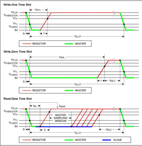
Figure 2. Read/write timing diagram.
