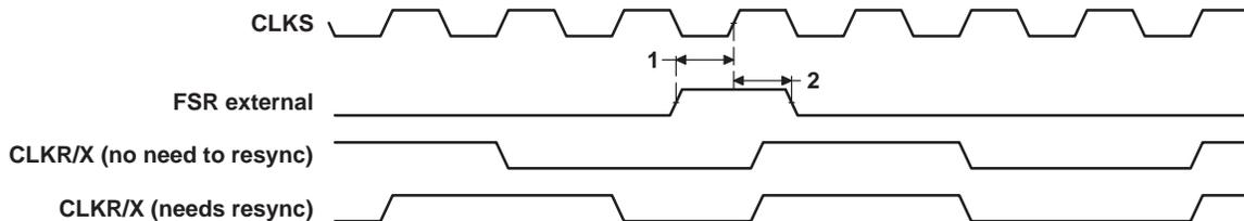
**Figure 52. FSR Timing When GSYNC = 1**
