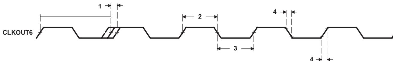
Figure 18. CLKOUT6 Timing
