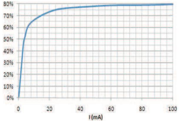
Figure 14. Efficiency Low Power Enabled
