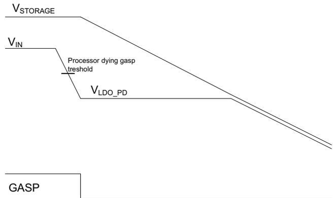
Figure 4. Pump and Dump Timing
