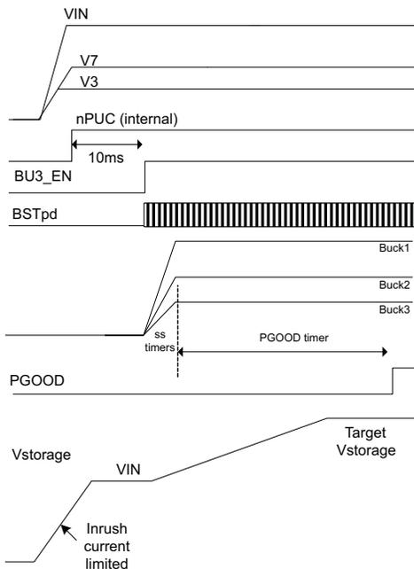
Figure 3. Power-Up Timing (Showing Automatic Start-Up)
