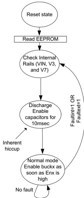
Faultint: Overtemperature, UVLO<sub>VIN</sub>, V7<sub>UVLO</sub>
