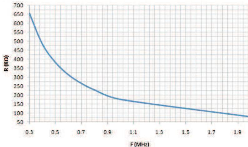
**Figure 30. ROSC vs Switching Frequency**
