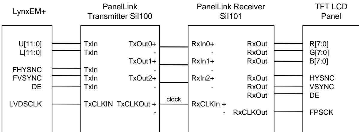
**Figure 22: PanelLink Interface with DSTN LCD Panel**
