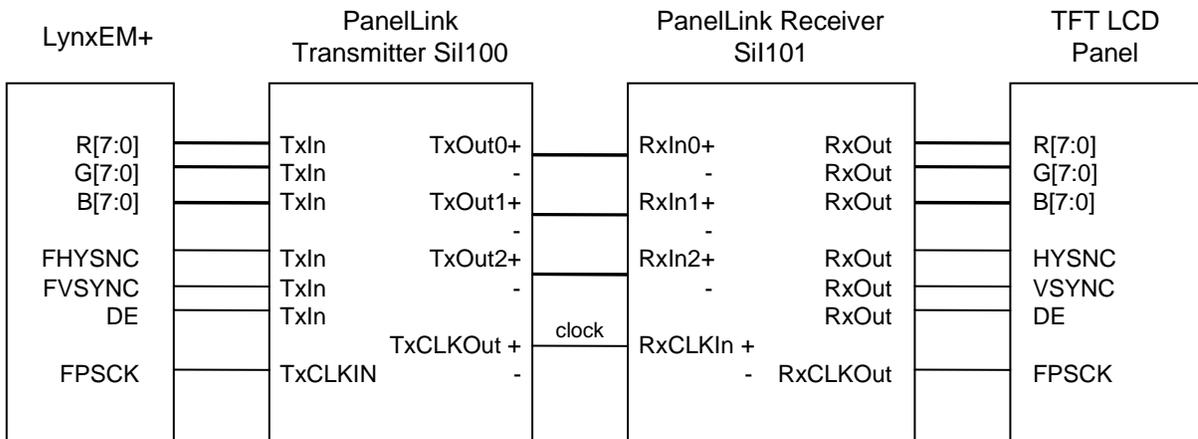
**Figure 21: PanelLink Interface with TFT LCD Panel**
