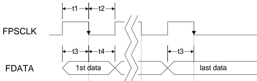
**Figure 32: DSTN Interface (Clock and Data) Timing**
