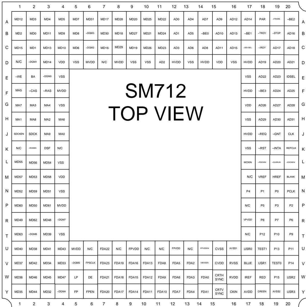
Figure 2: SM712 Pin Diagram for 256 BGA Package
