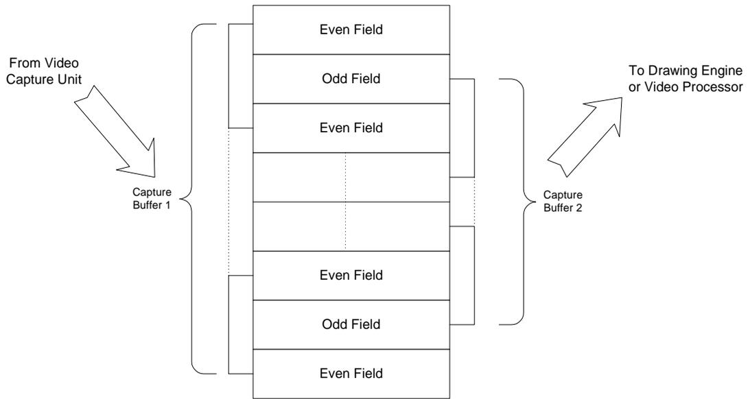
**Figure 10: Capture Buffer Structure in Interlaced Mode**
