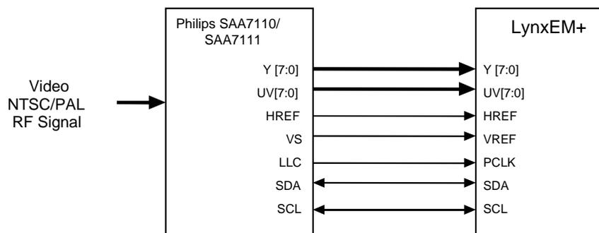
**Figure 7: Video Encoder Interface via Video Port**
