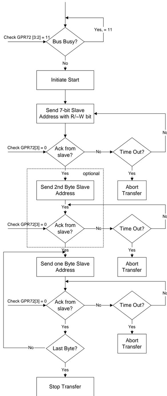
**Figure 24: LynxEM+ I<sup>2</sup>C Bus Protocol Flow Chart**
