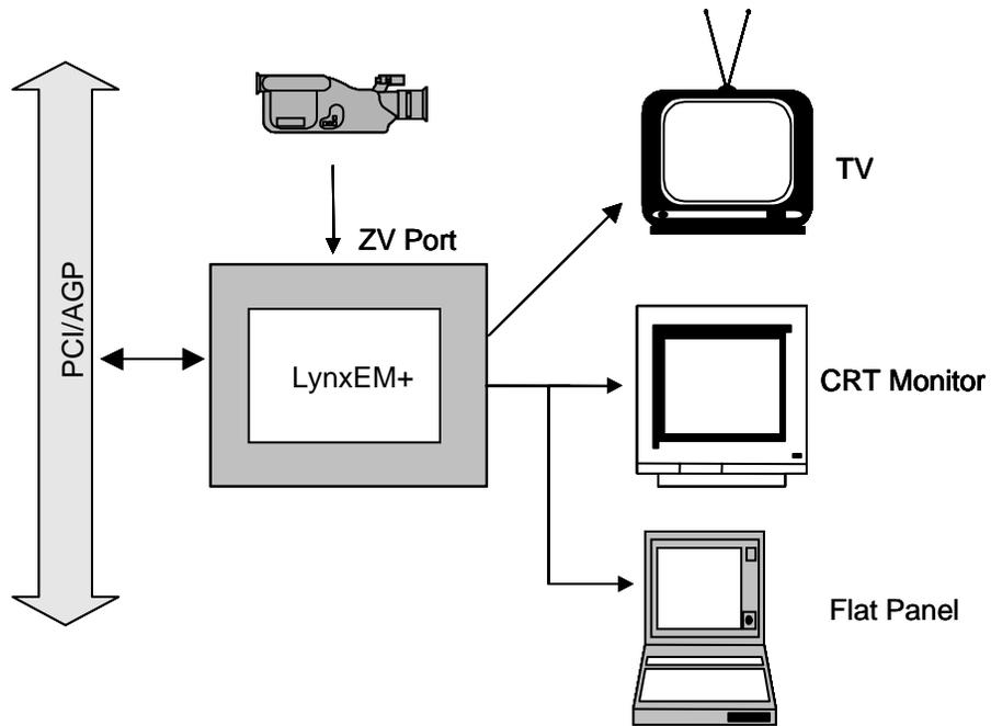
**Figure 1: System Block Diagram for the LynxEM+**
