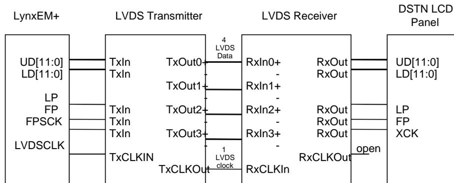
**Figure 19: LVDS Interface with DSTN LCD Panel**
