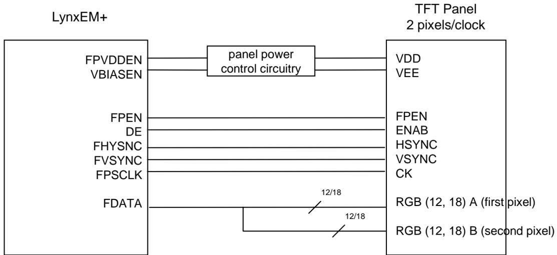
**Figure 13: TFT Panel (2 pixels/clock) Interface Diagram**
