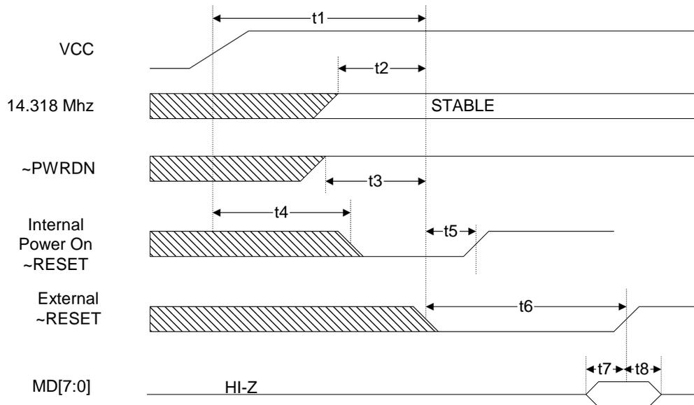
**Figure 29: Power-on Reset and Reset Configuration Timing**
