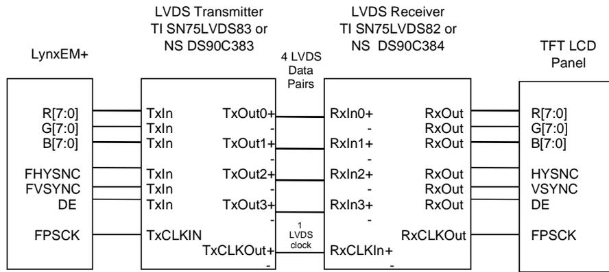
**Figure 18: LVDS Interface with TFT LCD Panel**
