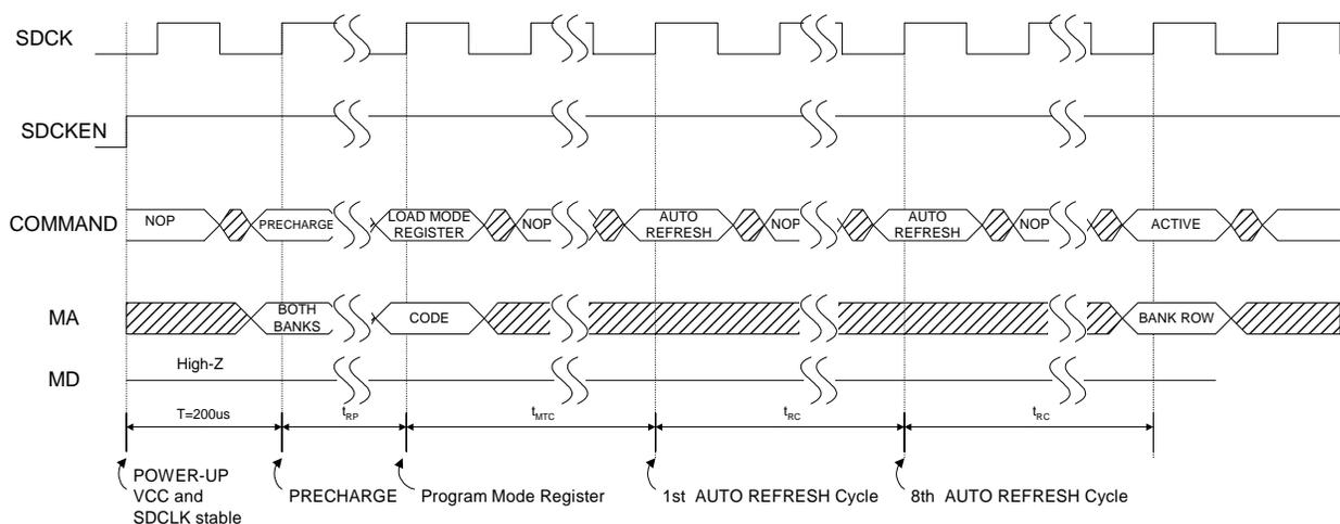
**Figure 4: External SGRAM Power-Up and Initialization Sequence**
