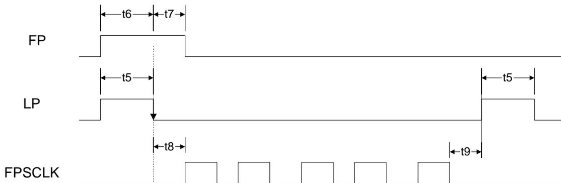
**Figure 33: DSTN Interface (Control and Clock) Timing**
