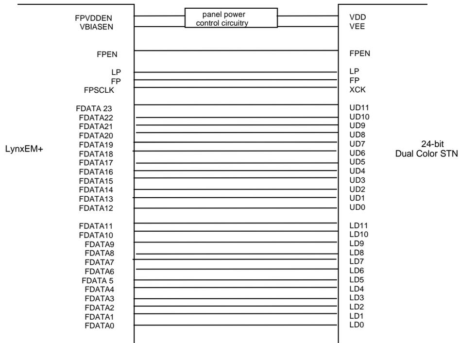
**Figure 15: 24-bit Dual Color STN Interface Diagram**
