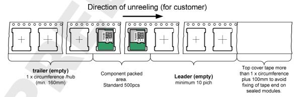
Empty hollow in component packed area shall be less than two per reel and those hollows shall not be consecutive.
