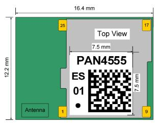
This label is suitable for reflow soldering and designed for the engineering sample status.
