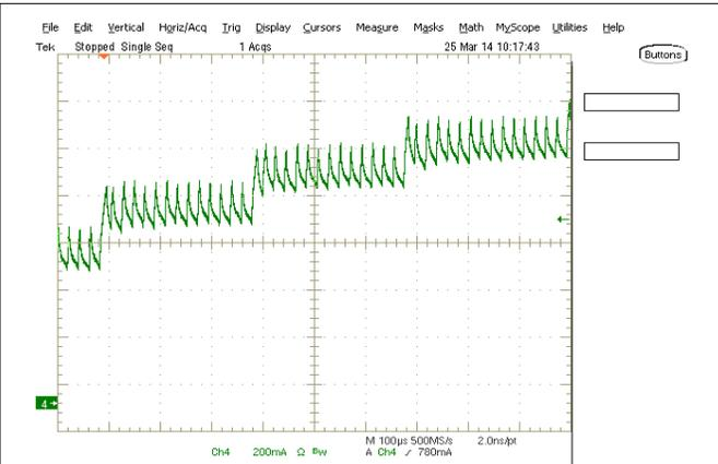
**Figure 8-3. Microstepping Waveform, Slow Decay on Increasing Steps**
