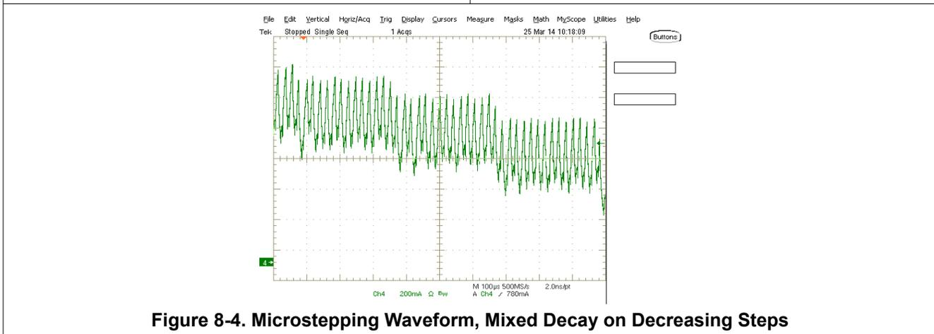
**Figure 8-4. Microstepping Waveform, Mixed Decay on Decreasing Steps**
