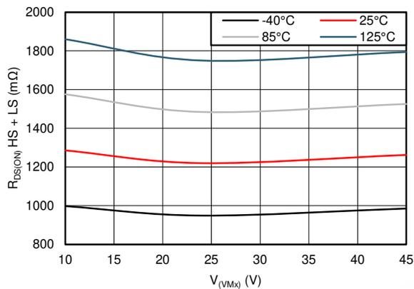
Figure 6-4.  $R_{DS(ON)}$  HS + LS vs  $V_{VMx}$
