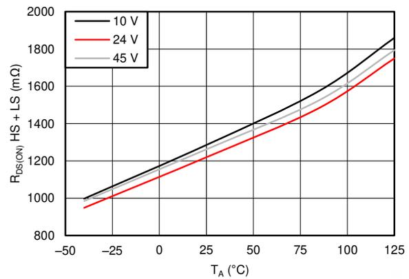
Figure 6-5.  $R_{DS(ON)}$  HS + LS vs Temperature
