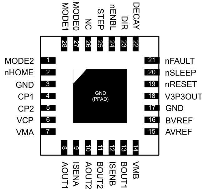
Figure 5-2. RHD Package 28-Pin VQFN Top View
