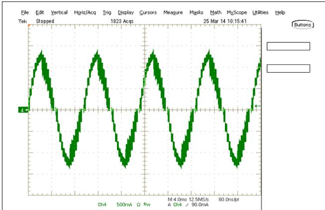
**Figure 8-2. Microstepping Waveform, Phase A, Mixed Decay**
