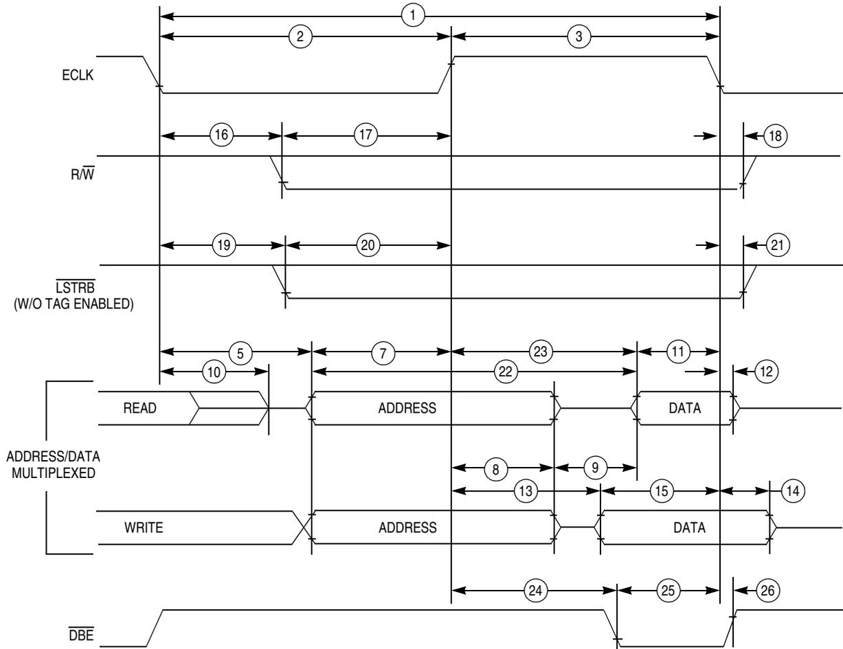
NOTE: Measurement points shown are 20% and 70% of  $V_{DD}$
