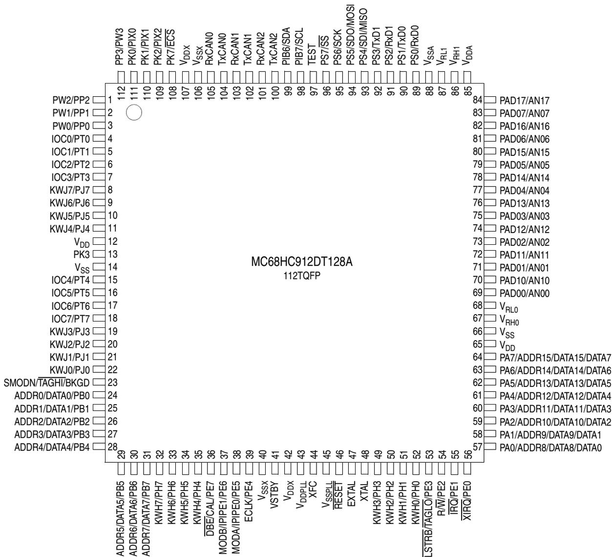
Note: TEST = This pin is used for factory test purposes. It is recommended that this pin is not connected in the application, but it may be bonded to 5.5 V max without issue. Never apply voltage higher than 5.5 V to this pin.
