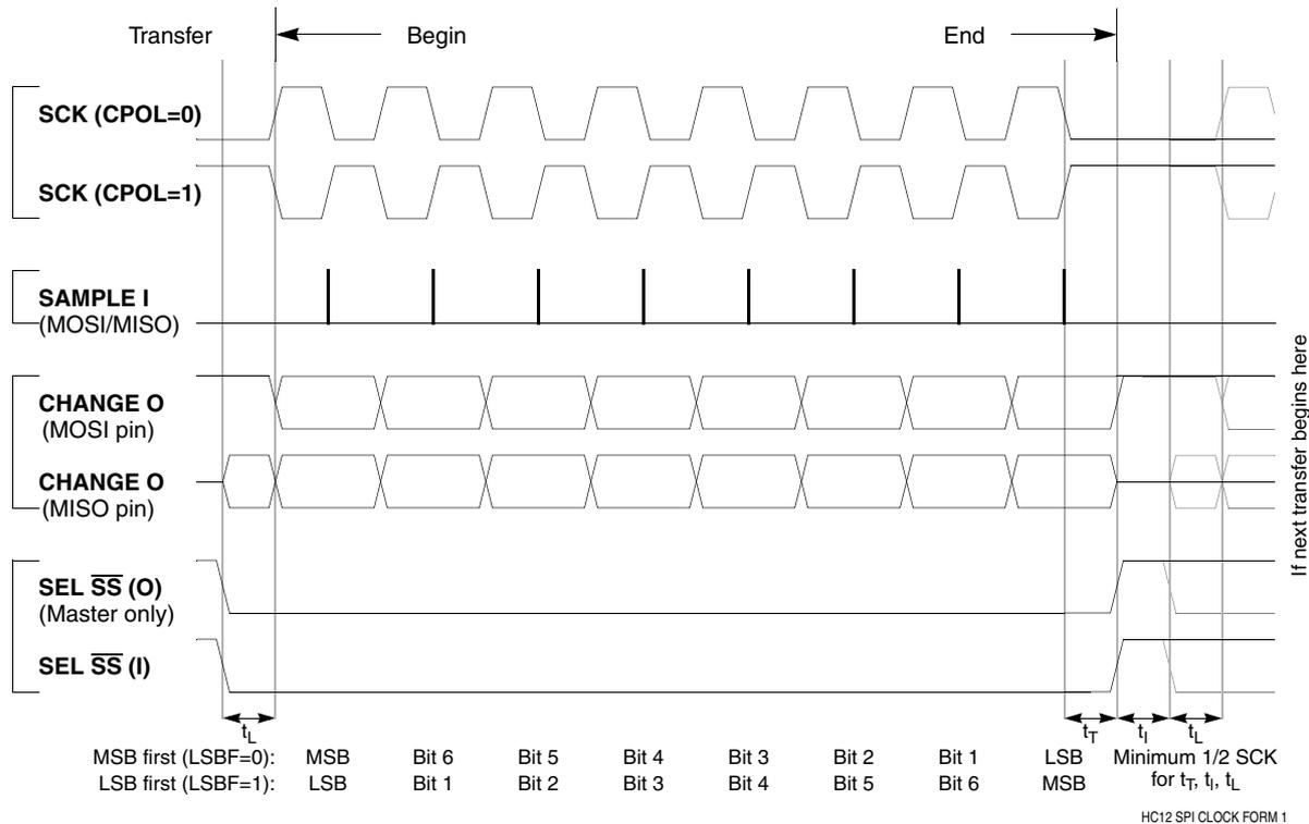
Figure 16-5. SPI Clock Format 1 (CPHA = 1)
