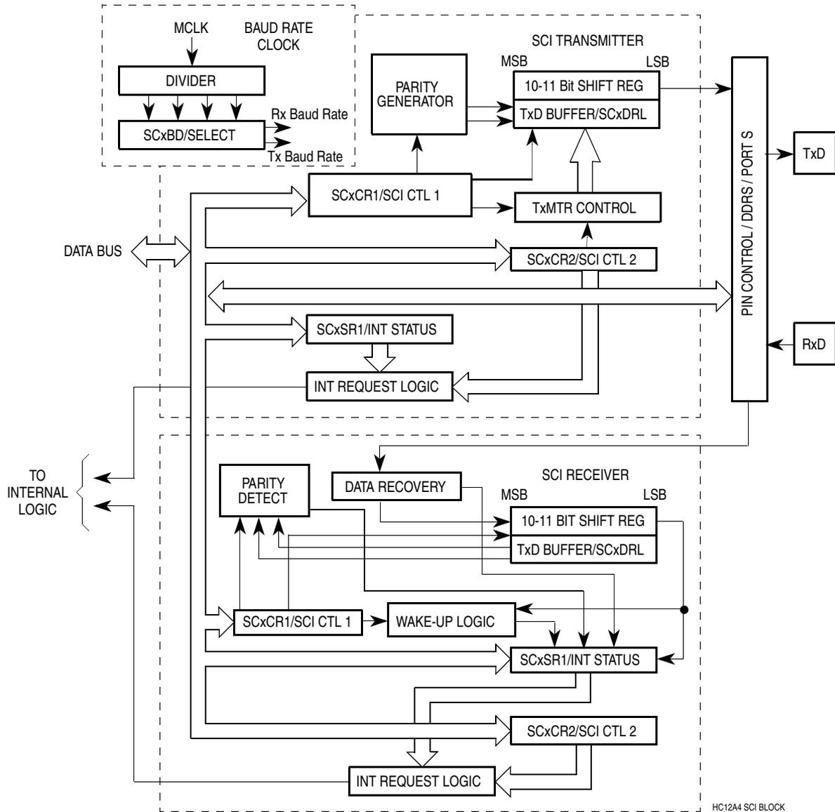
**Figure 16-2. Serial Communications Interface Block Diagram**
