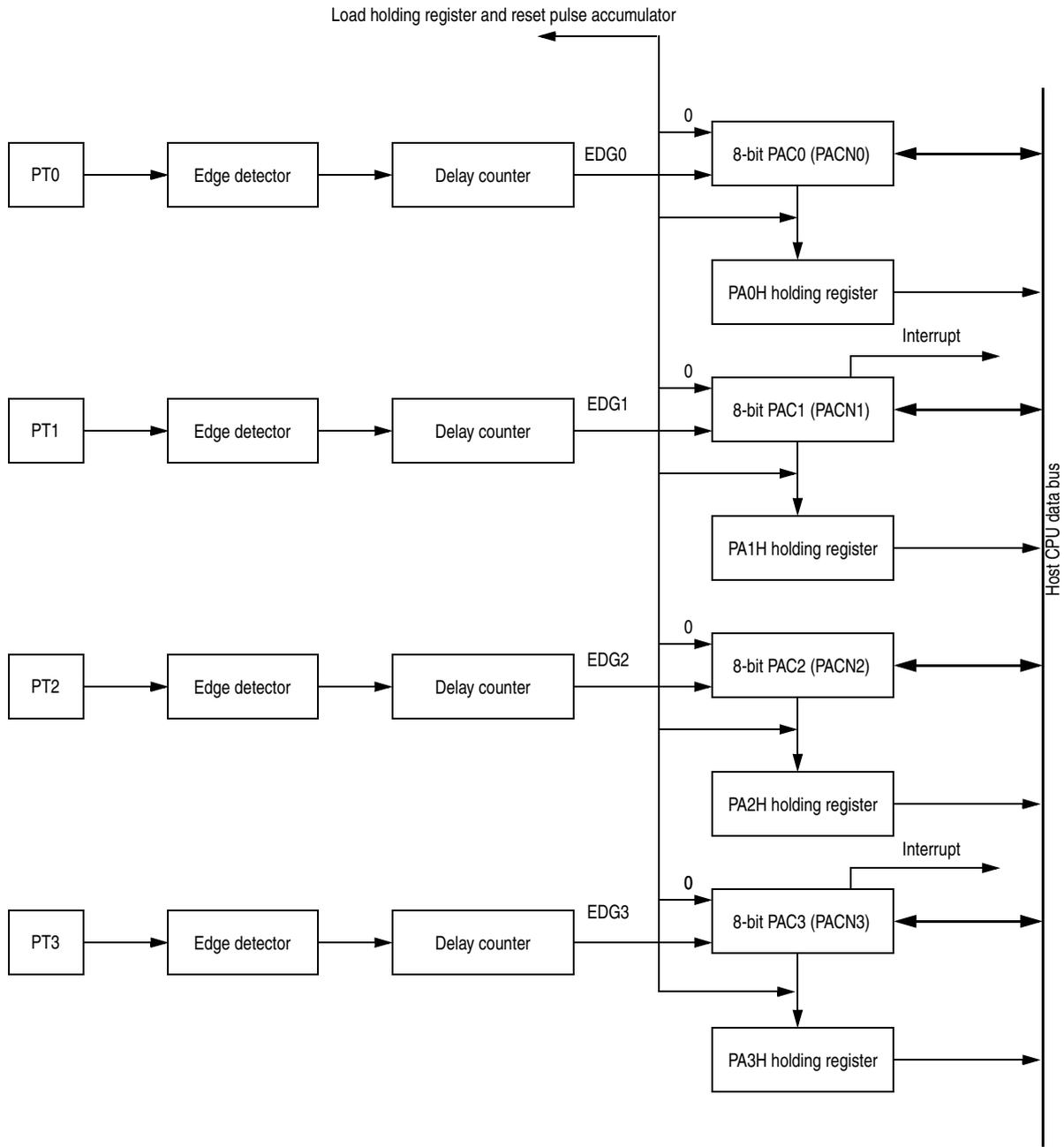
**Figure 15-3. 8-Bit Pulse Accumulators Block Diagram**
