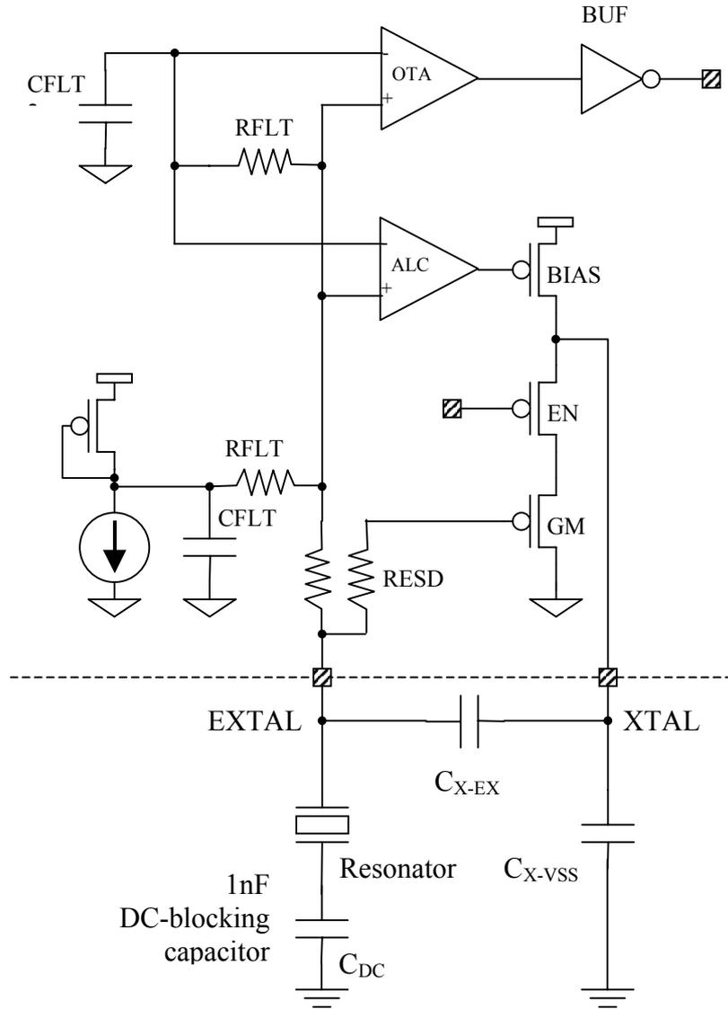
Figure 13-3. MC68HC912Dx128C Crystal with DC Blocking Capacitor
