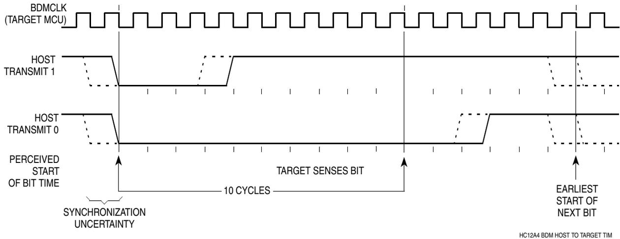
**Figure 20-1. BDM Host to Target Serial Bit Timing**
