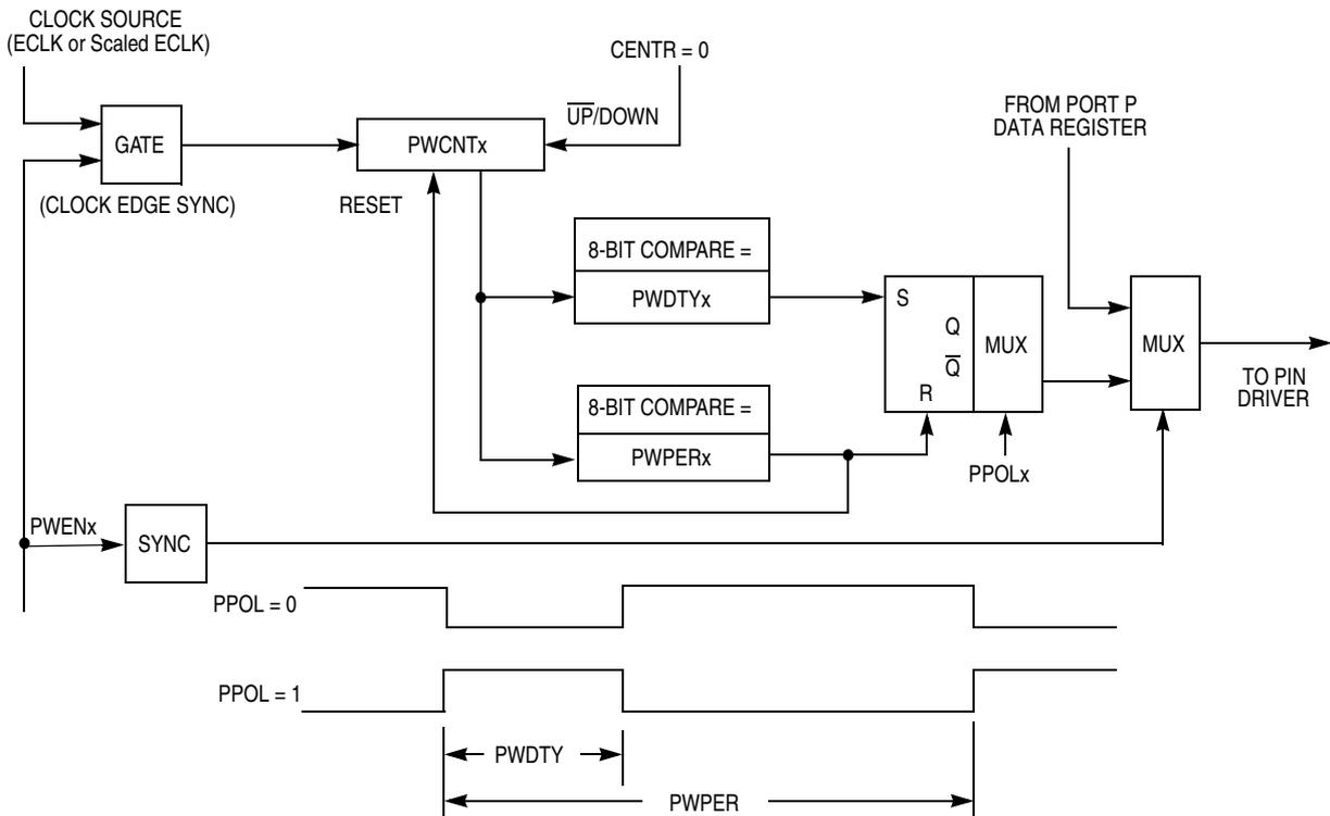
Figure 14-1. Block Diagram of PWM Left-Aligned Output Channel
