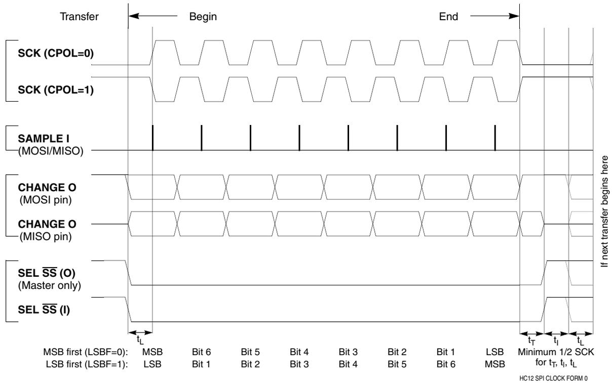
Figure 16-4. SPI Clock Format 0 (CPHA = 0)
