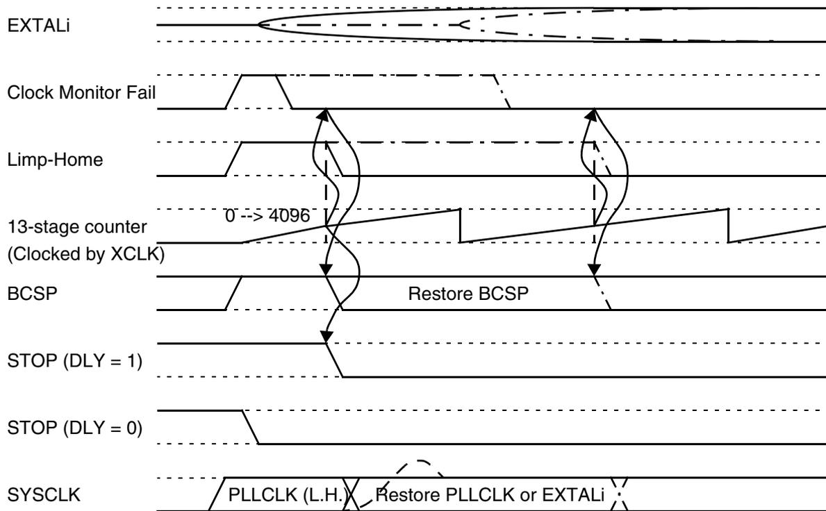
**Figure 12-5. STOP Exit and Fast STOP Recovery**
