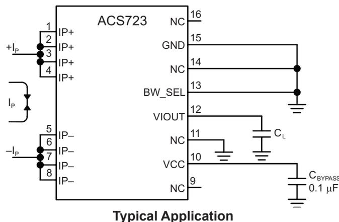
The ACS723 outputs an analog signal,  $V_{IOUT}$ , that changes, proportionally, with the bidirectional AC or DC primary sensed current,  $I_p$ , within the specified measurement range. The BW\_SEL pin can be used to select one of the two bandwidths to optimize the noise performance. Grounding the BW\_SEL pin puts the part in the high bandwidth (80 kHz) mode.
