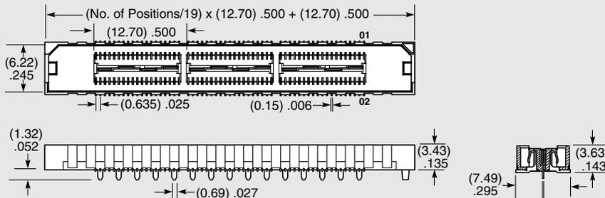
**Note:** Rugged through-hole ground plane soldered to board (requires paste-over-hole, not press-fit) for added retention to PCB.
