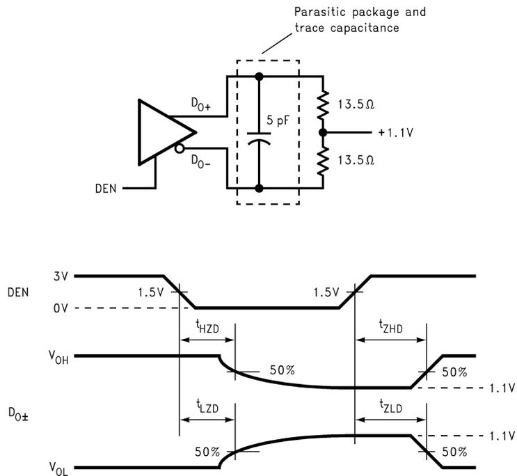
**Figure 8. Serializer TRI-STATE Test Circuit and Timing**
