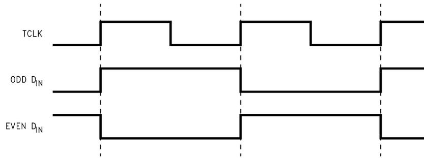
Figure 4. “Worst Case” Serializer ICC Test Pattern
