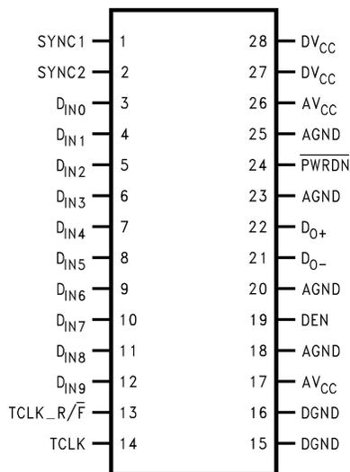
**Figure 14. DS92LV1023TMSA - Serializer SSOP Package**
