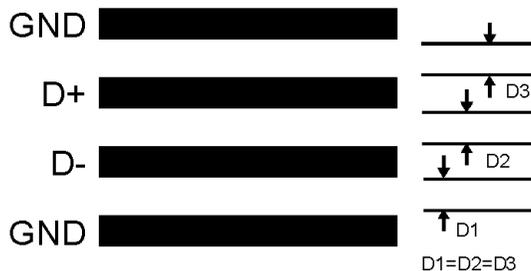
**Figure 19. Ideal Diode Trace Layout**
