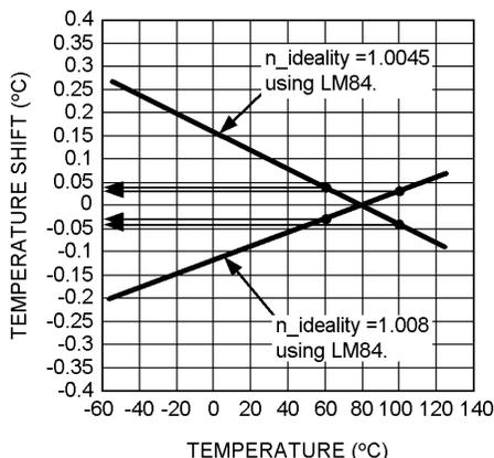
**Figure 18. Compensating for an Untargeted Non-Ideality Factor**
