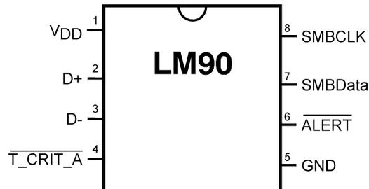
**Figure 1. 8-Lead VSSOP - TOP VIEW**
