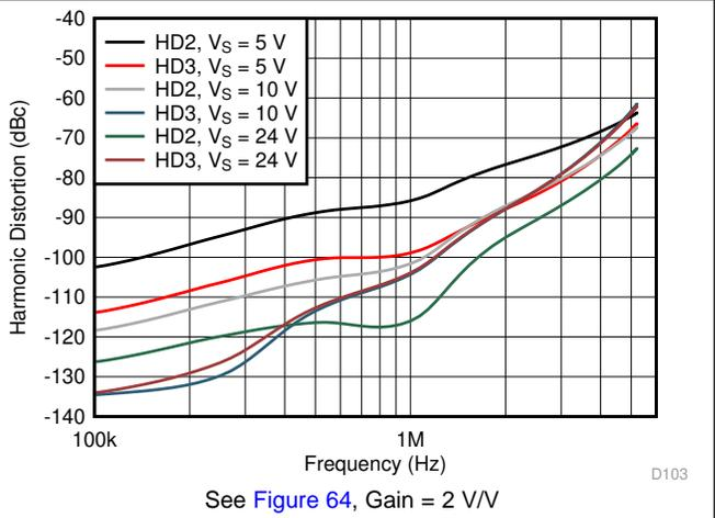
Figure 47. Harmonic Distortion vs Frequency vs Supply Voltage
