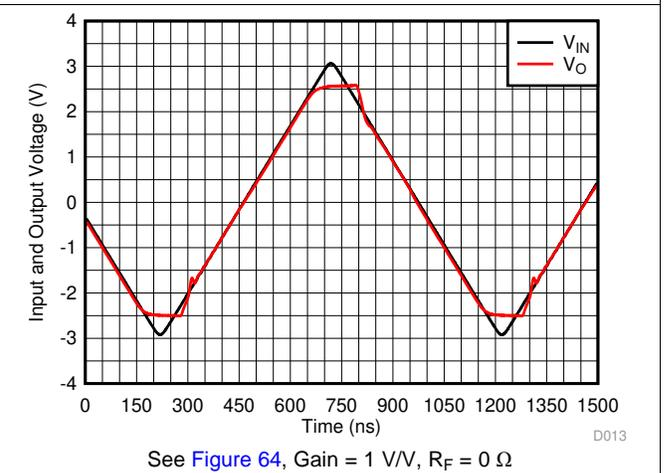
Figure 39. Input Overdrive Recovery
