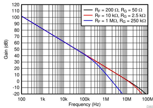
Figure 67. Loop-Gain vs. Frequency for Circuit of Figure 66
