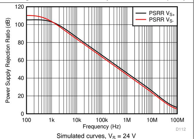
Figure 55. Power Supply Rejection Ratio vs Frequency
