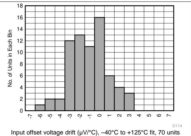
Figure 61. Input Offset Voltage Drift Distribution
