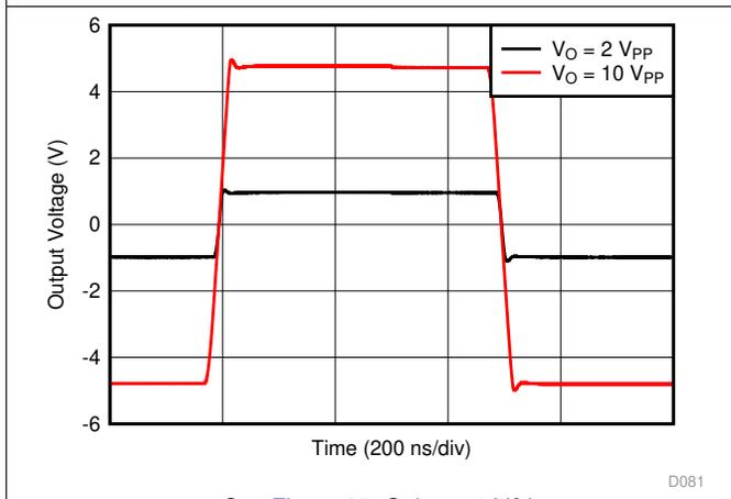
**Figure 29. Large-Signal Transient Response**
