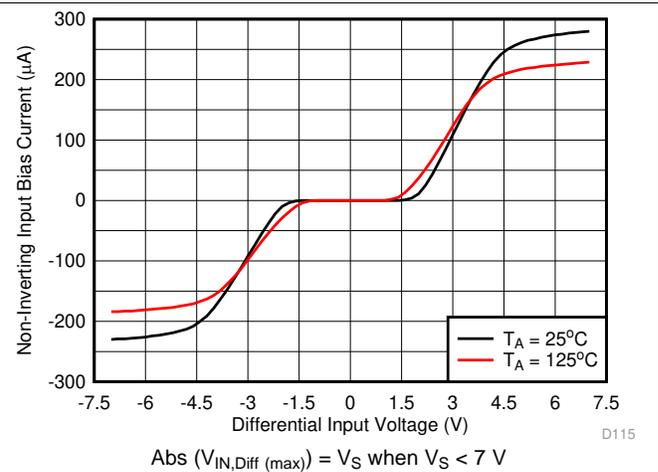
Figure 57. Input Bias Current vs Differential Input Voltage
