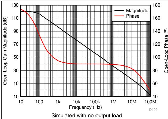
Figure 44. Open-Loop Gain and Phase vs Frequency
