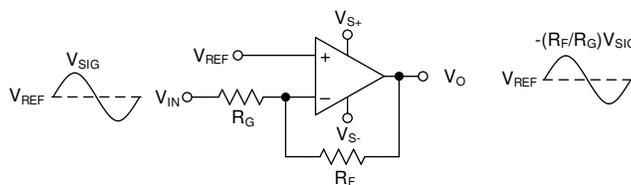
**Figure 65. Inverting Amplifier**
