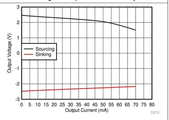
Figure 41. Output Voltage Range vs Output Current
