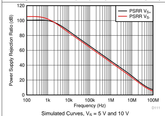
Figure 54. Power Supply Rejection Ratio vs Frequency
