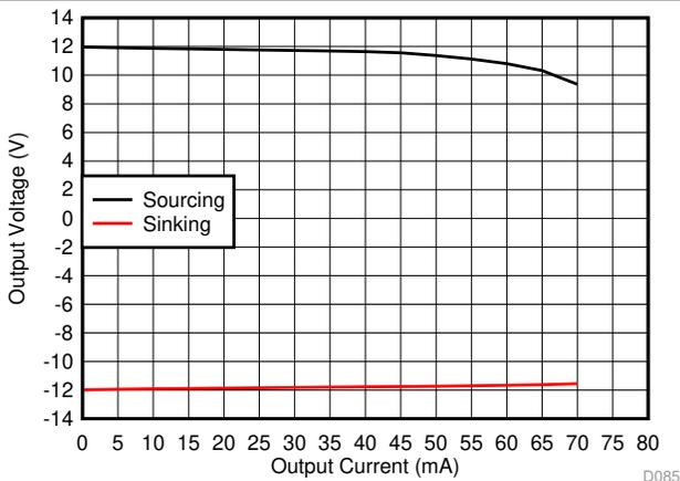
Figure 33. Output Voltage Range vs Load Current
