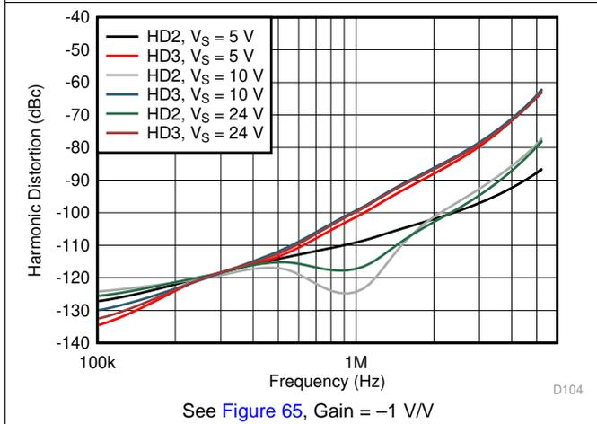
Figure 48. Harmonic Distortion vs Frequency vs Supply Voltage
