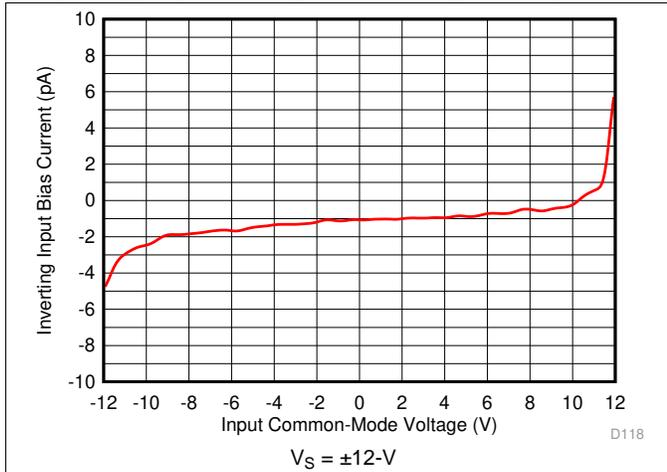
Figure 56. Input Bias Current vs Input Common-Mode Voltage
