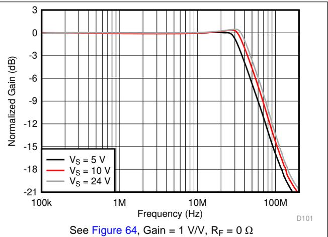
Figure 45. Large-Signal Response vs Supply Voltage
