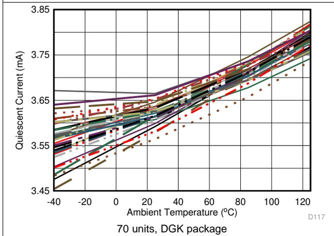
Figure 58. Quiescent Current vs Ambient Temperature
