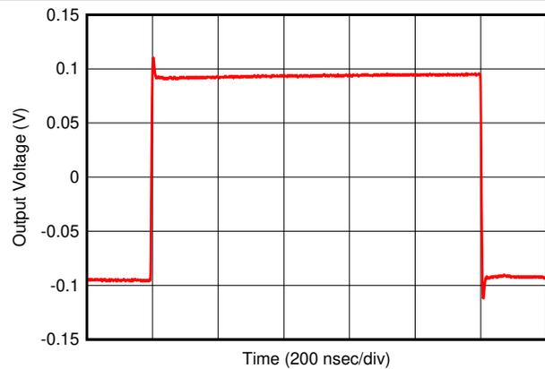
See Figure 64, Gain = 1 V/V,  $R_F = 0\ \Omega$
