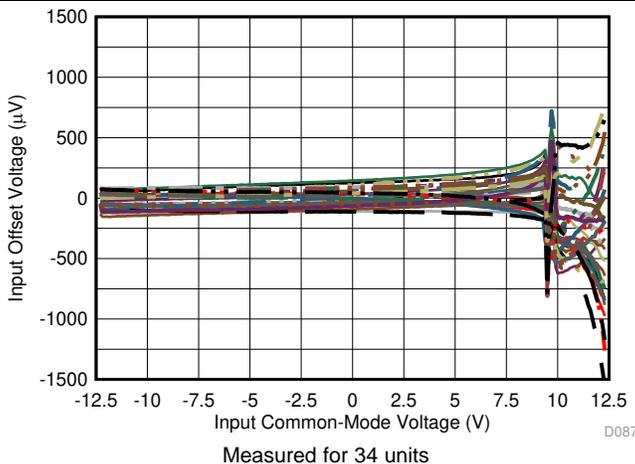
Figure 35. Input Offset Voltage vs Input Common-Mode Voltage
