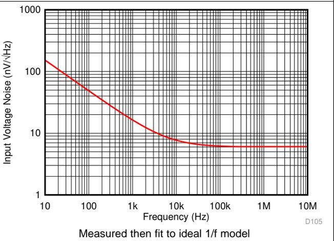
Figure 49. Input Voltage Noise Density vs Frequency
