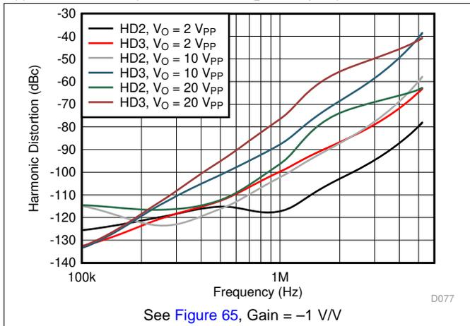
**Figure 25. Harmonic Distortion vs Frequency vs  $V_O$**
