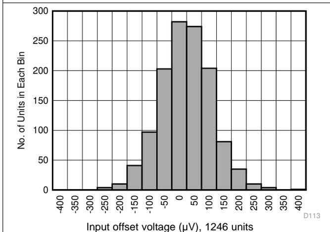
Figure 60. Input Offset Voltage Distribution
