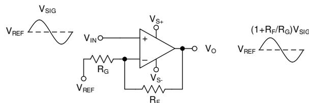
**Figure 64. Noninverting Amplifier**
