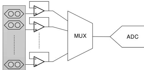
**Figure 76. Multichannel Sensor Interface Using Multiple Amplifiers**
