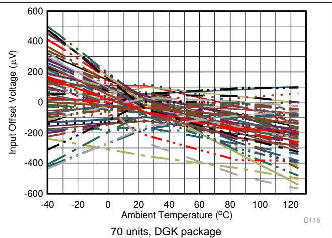
Figure 59. Input Offset Voltage vs Ambient Temperature
