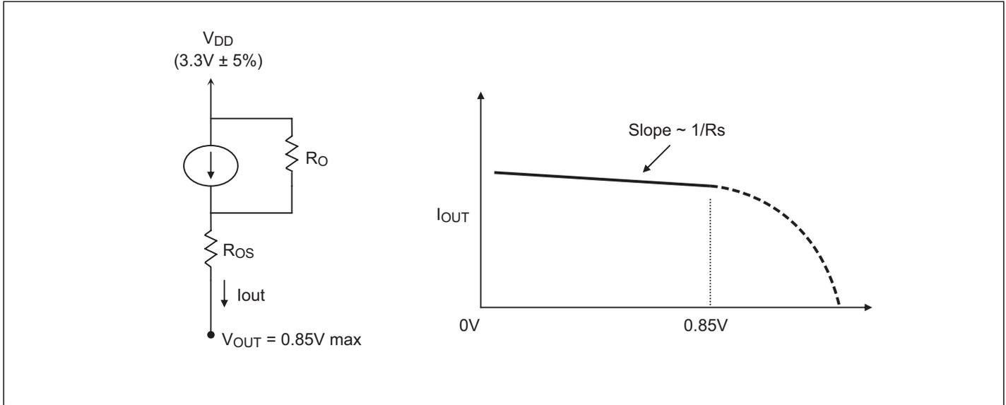
**Differential Clock Buffer characteristics**
