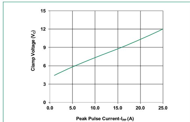
**Clamping Voltage vs.  $I_{pp}$  (Line-to-Line)**
