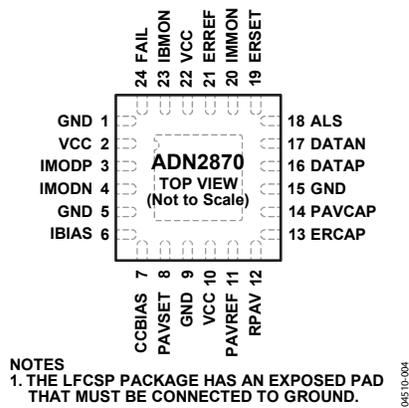
Figure 5. Pin Configuration
