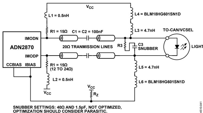
SNUBBER SETTINGS: 40Ω AND 1.5pF, NOT OPTIMIZED, OPTIMIZATION SHOULD CONSIDER PARASITIC.
