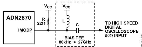
Figure 2. High Speed Electrical Test Output Circuit
