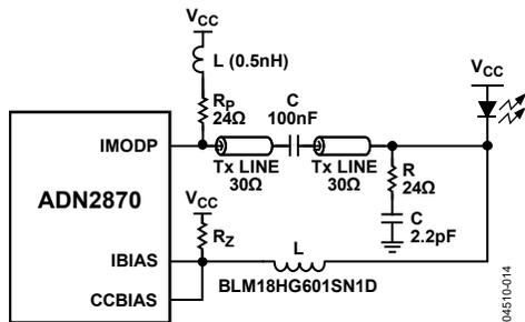
Figure 32. Recommended Interface for ADN2870 AC Coupling
