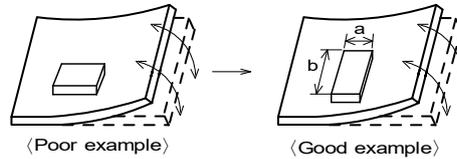
(2) Components location on PCB separation
