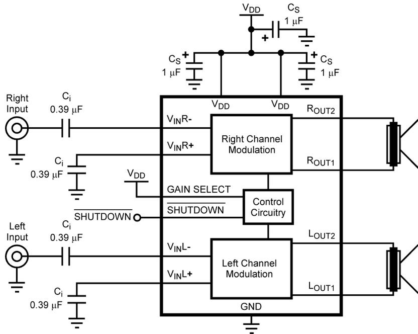
Figure 26. Single-Ended Input with Low Gain Selection Configuration
