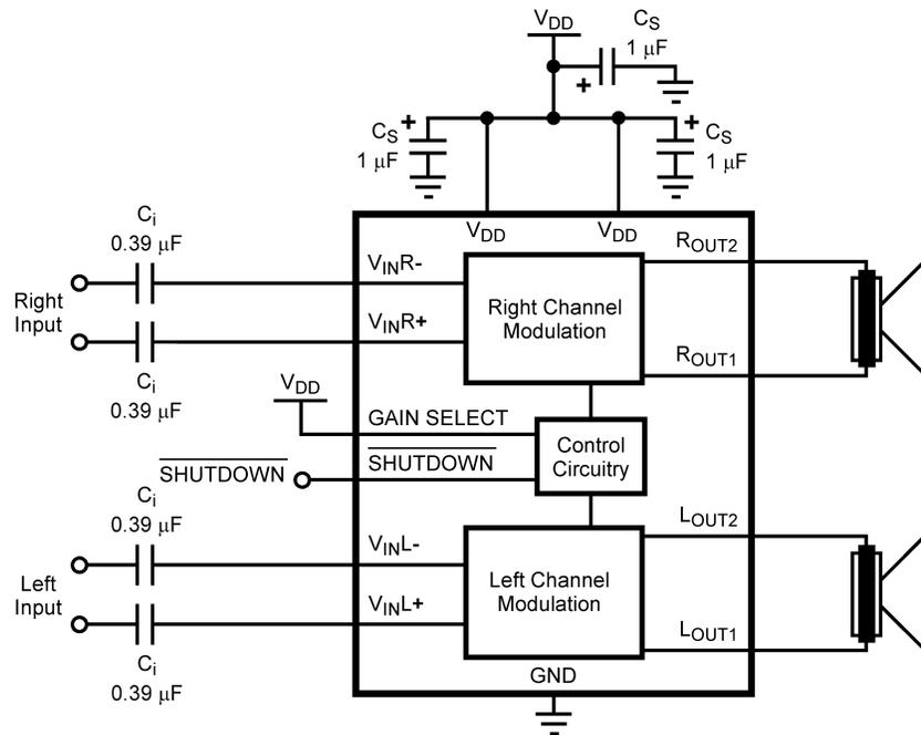
Figure 27. Differential Input with Low Gain Selection Configuration
