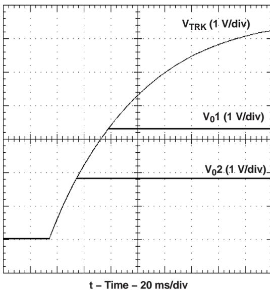
Figure 13. Simultaneous Power Up With Auto-Track Control
