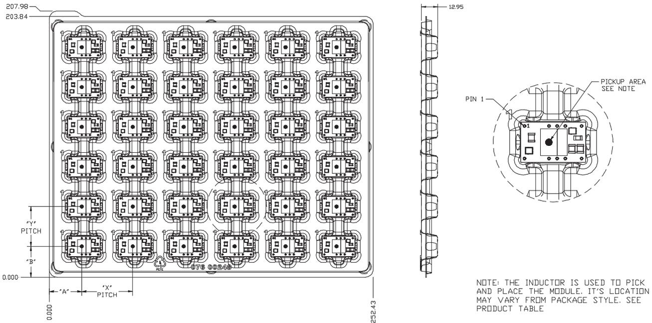
NOTE: THE INDUCTOR IS USED TO PICK AND PLACE THE MODULE. IT'S LOCATION MAY VARY FROM PACKAGE STYLE. SEE PRODUCT TABLE
