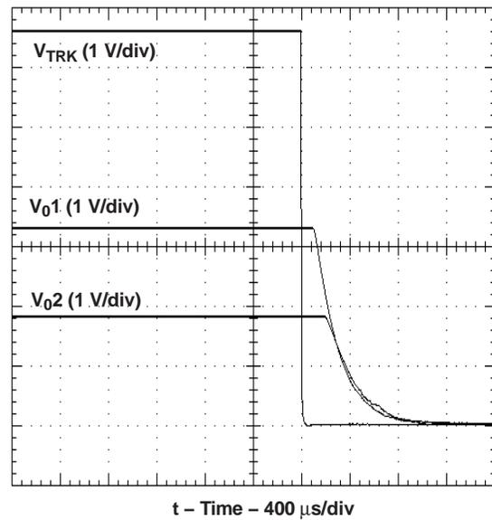
Figure 14. Simultaneous Power Down with Auto-Track Control
