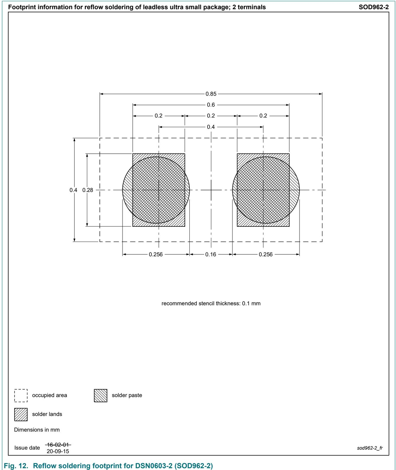
Fig. 12. Reflow soldering footprint for DSN0603-2 (SOD962-2)
