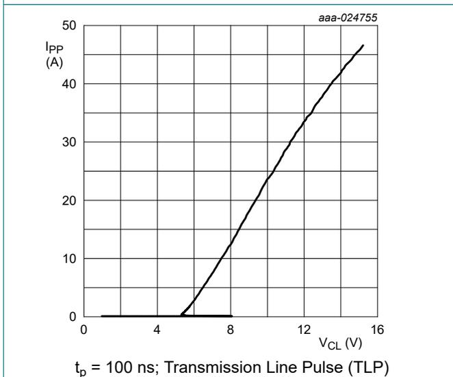
Fig. 5. Positive clamping voltage (TLP); typical values
