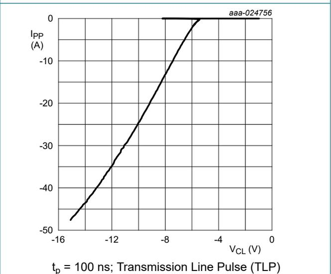
Fig. 6. Negative clamping voltage (TLP); typical values
