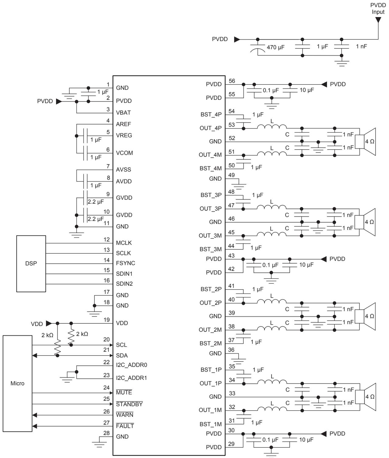
Figure 59. TAS6424L-Q1 Typical 4-Channel BTL Application Schematic
