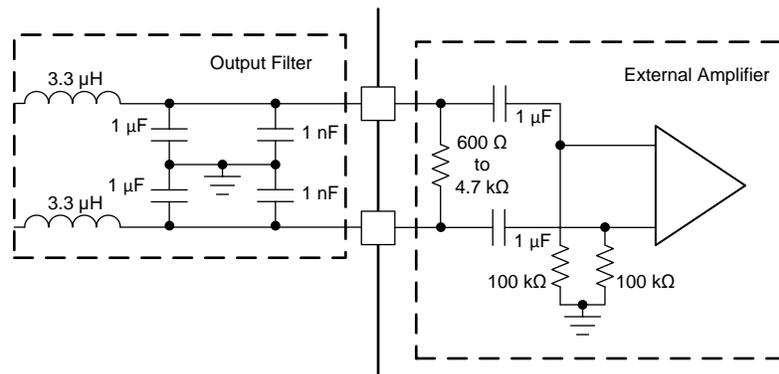
**Figure 58. External Amplifier Input Configuration for Line Driver**
