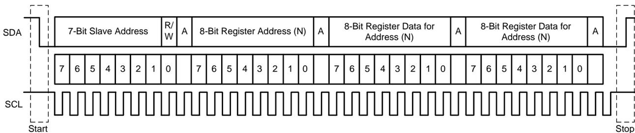
**Figure 21. Typical I<sup>2</sup>C Sequence**
