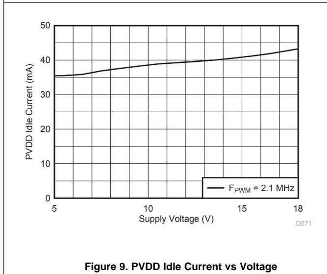
Figure 9. PVDD Idle Current vs Voltage
