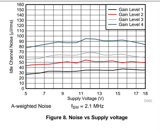
Figure 8. Noise vs Supply voltage
