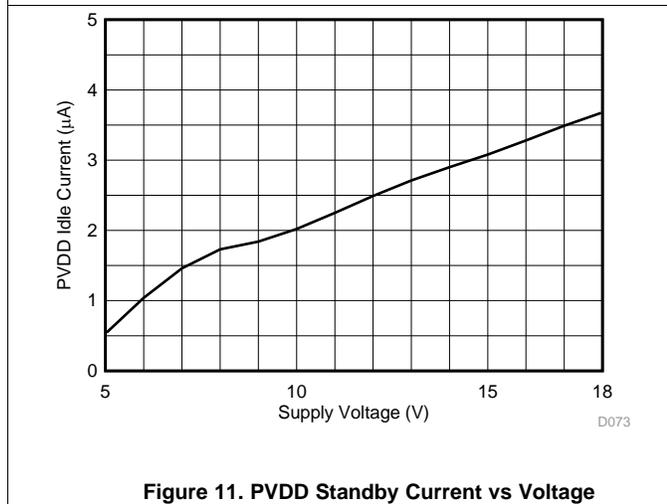
Figure 11. PVDD Standby Current vs Voltage
