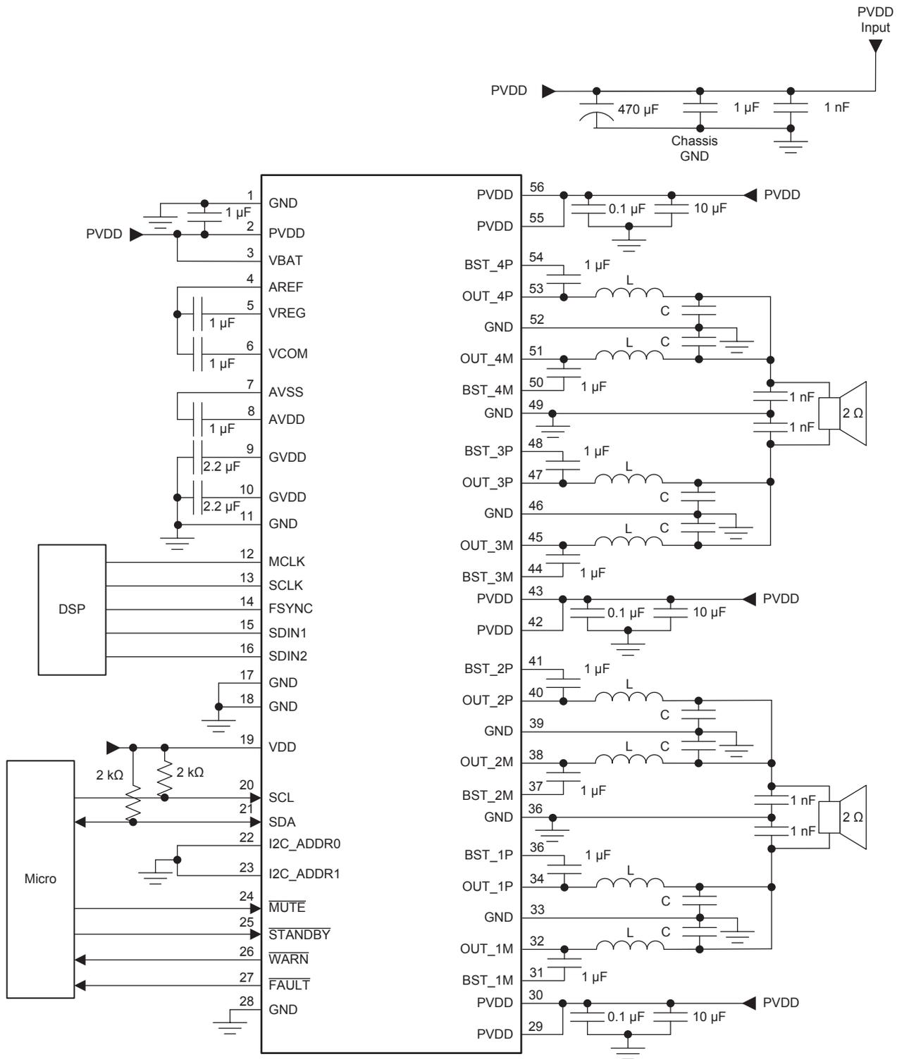
Figure 62. TAS6424L-Q1 Typical 2-Channel PBTL Application Schematic
