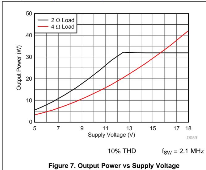
Figure 7. Output Power vs Supply Voltage
