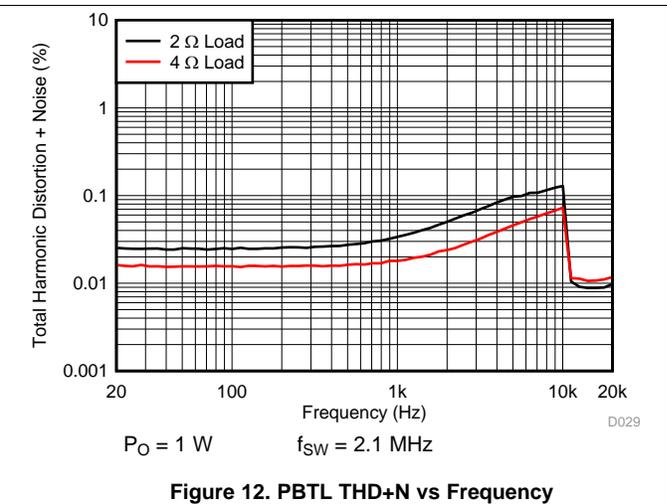
Figure 12. PBTLD THD+N vs Frequency
