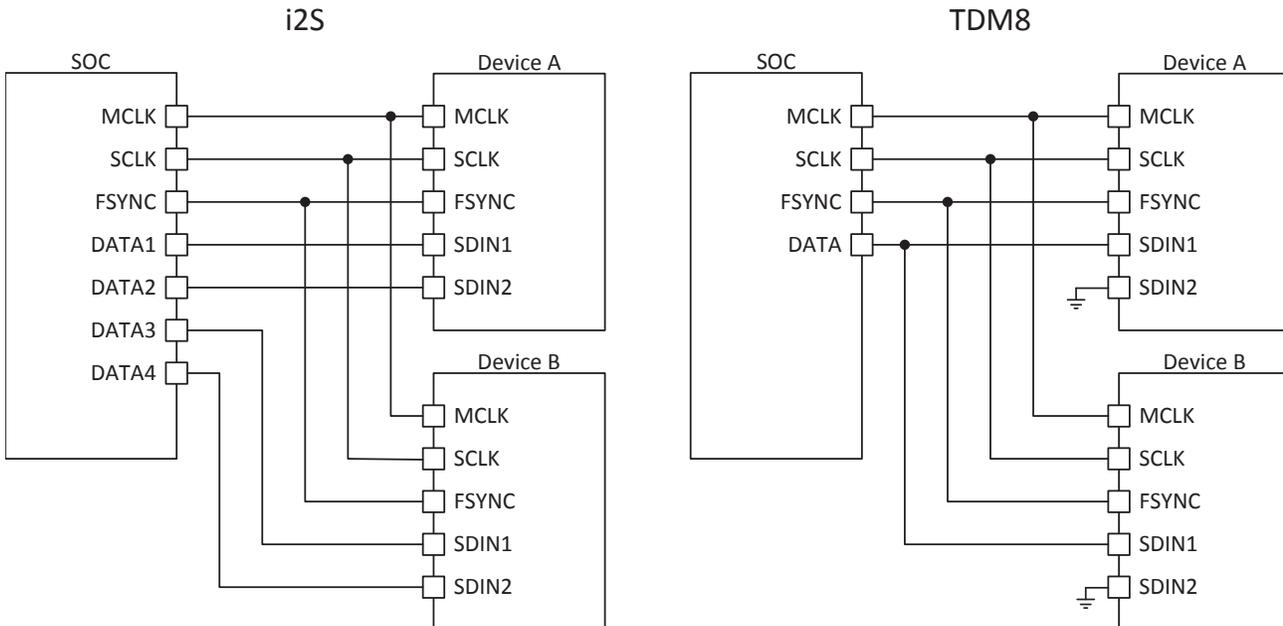
Figure 15. Digital-Audio Data Connection
