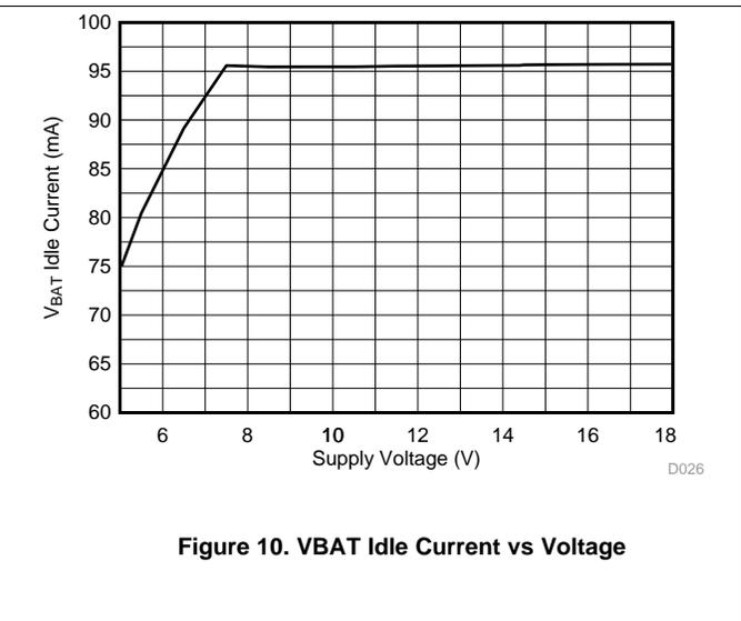
Figure 10. VBAT Idle Current vs Voltage
