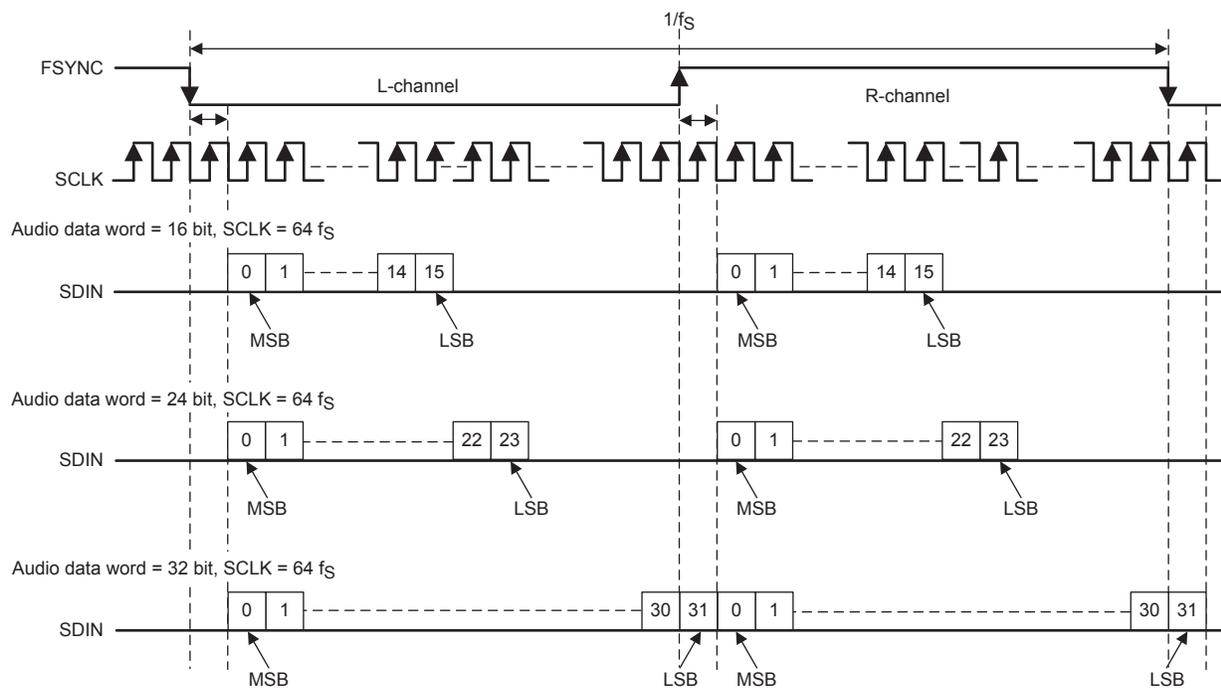
**Figure 18. I<sup>2</sup>S Audio Data Format**
