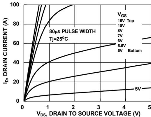
Figure 9. Saturation Characteristics
