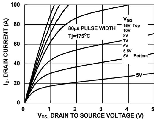
Figure 10. Saturation Characteristics
