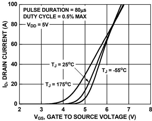
Figure 7. Transfer Characteristics
