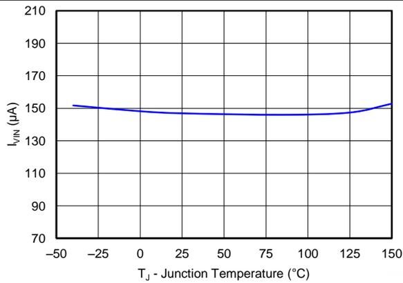
Figure 17. V<sub>IN</sub> Supply Current vs Junction Temperature
