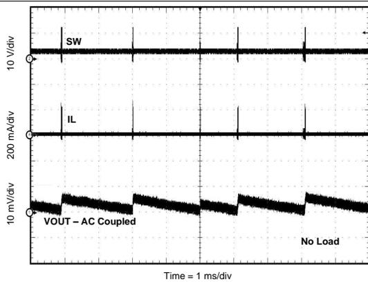
**Figure 42. Output Ripple PSM**
