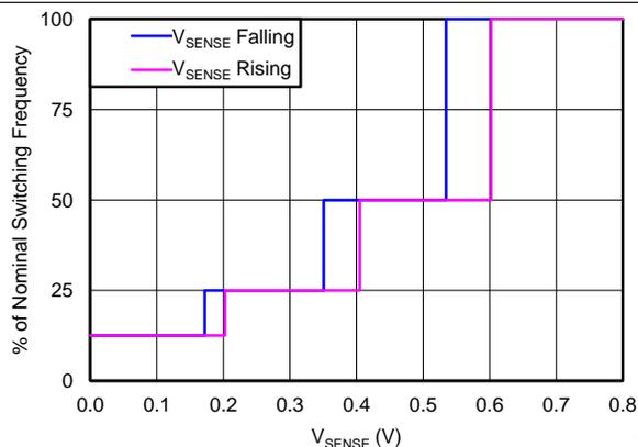
Figure 14. Switching Frequency vs V<sub>SENSE</sub>
