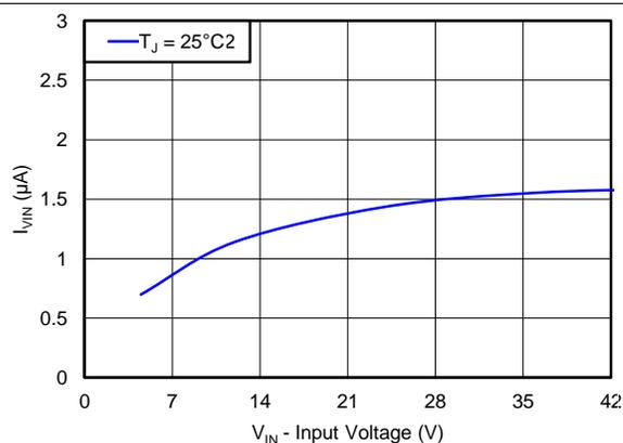
Figure 16. Shutdown Supply Current vs Input Voltage (V<sub>IN</sub>)
