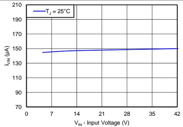
Figure 18. V<sub>IN</sub> Supply Current vs Input Voltage
