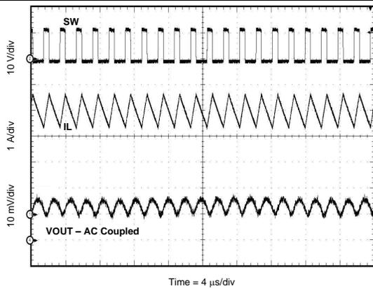
**Figure 40. Output Ripple CCM**
