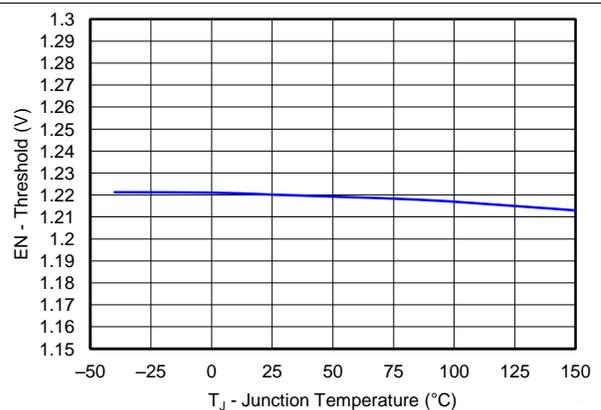
Figure 10. EN Terminal Voltage vs Junction Temperature
