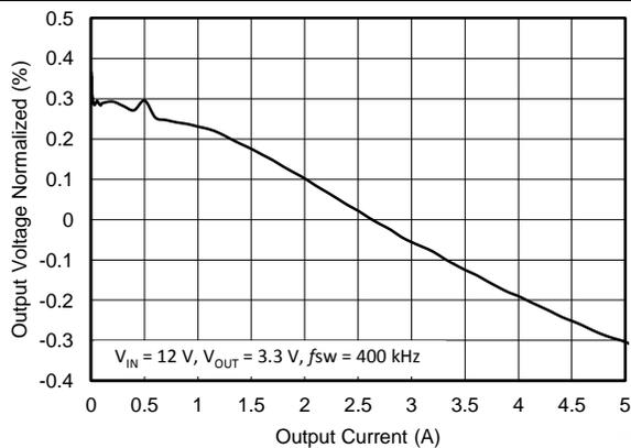
Figure 52. Regulation vs Load Current
