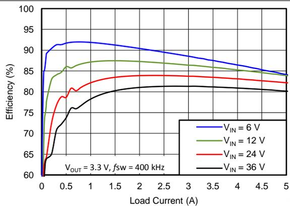
Figure 48. Efficiency vs Load Current
