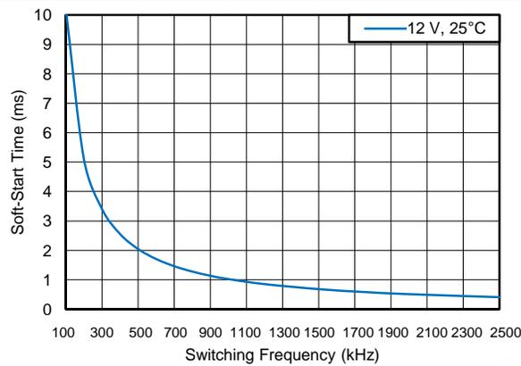
Figure 21. Soft-Start Time vs Switching Frequency
