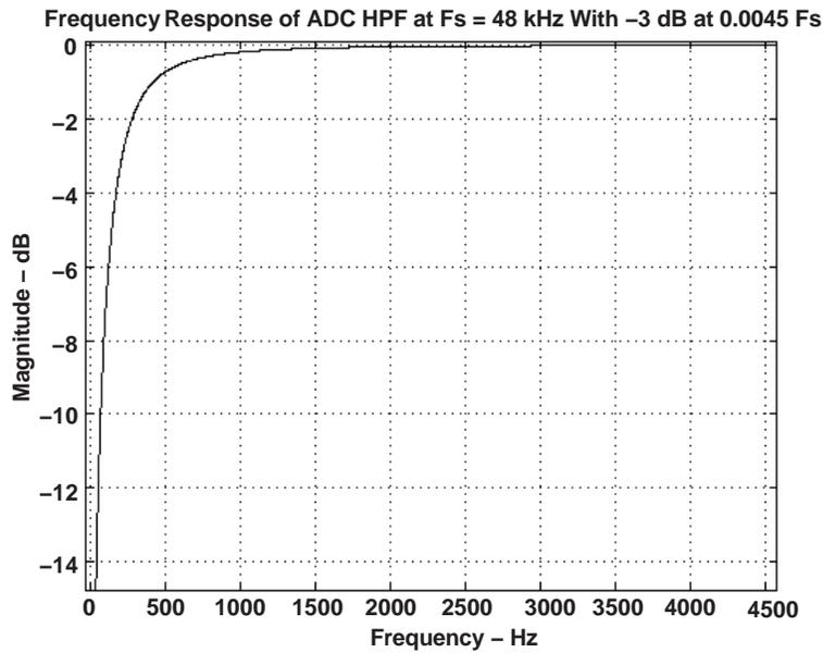
**Frequency Response of ADC High-Pass Filter (Fcut-off = 0.0125 Fs)**
