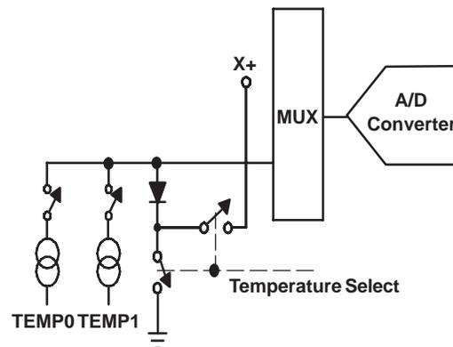
**Figure 25. Functional Block Diagram of Temperature Measurement Mode**
