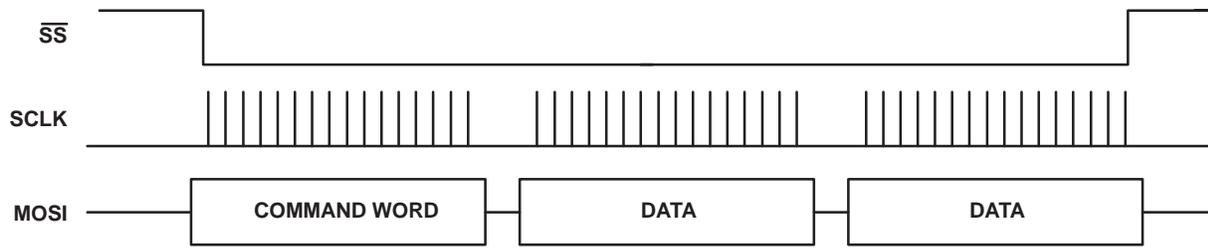
Figure 30. Write Operation for 'AIC26 SPI Interface
