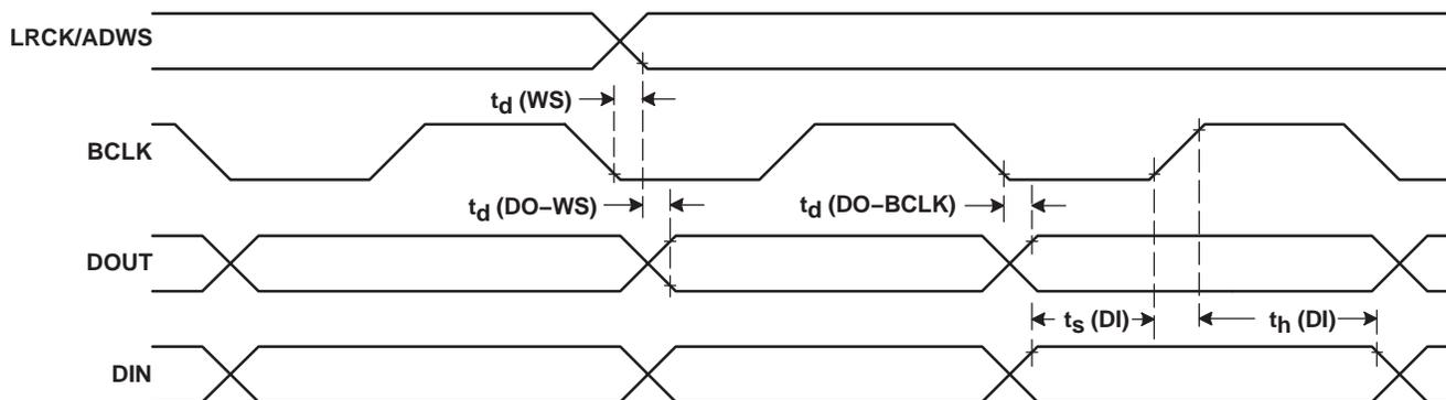
Figure 1. I<sup>2</sup>S/LJF/RJF Timing in Master Mode
