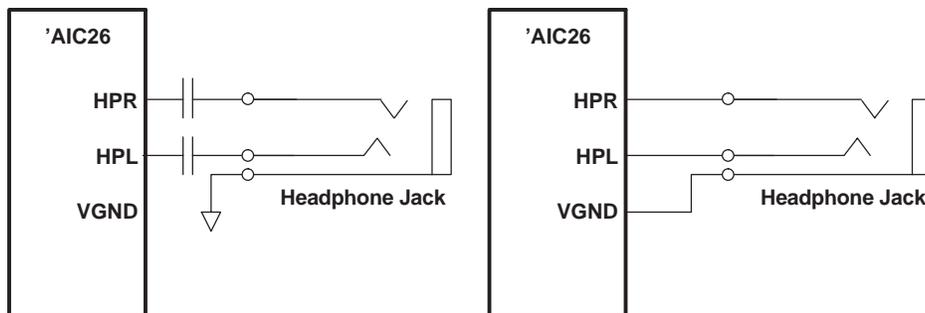
Figure 21. Headphone Configurations, AC-Coupled (left) and Capless (right)
