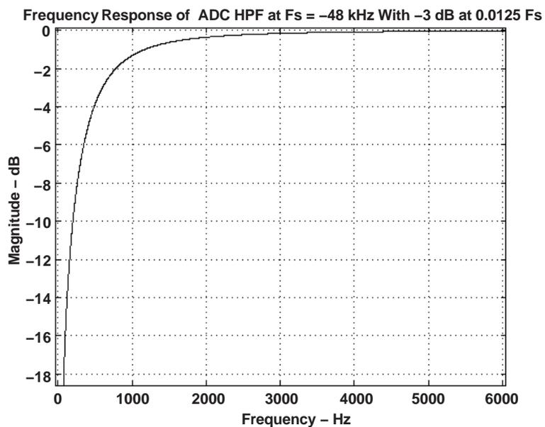
**Frequency Response of ADC High-Pass Filter (Fcut-off = 0.025 Fs)**
