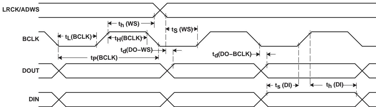
Figure 3. I<sup>2</sup>S/LJF/RJF Timing in Slave Mode
