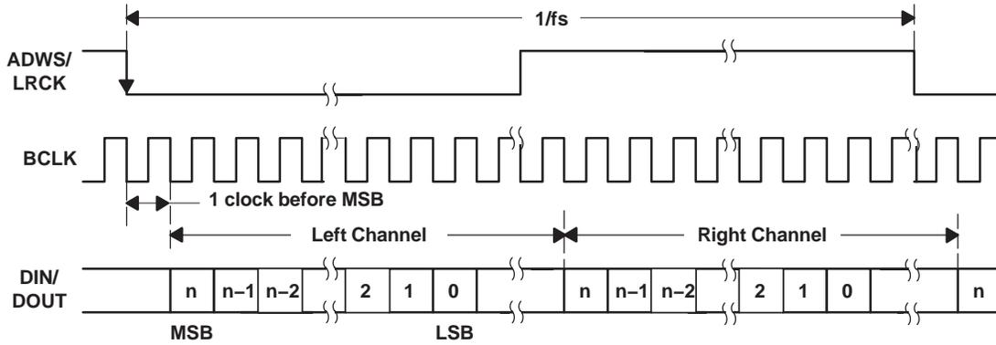
Figure 16. Timing Diagram for I<sup>2</sup>S Mode
