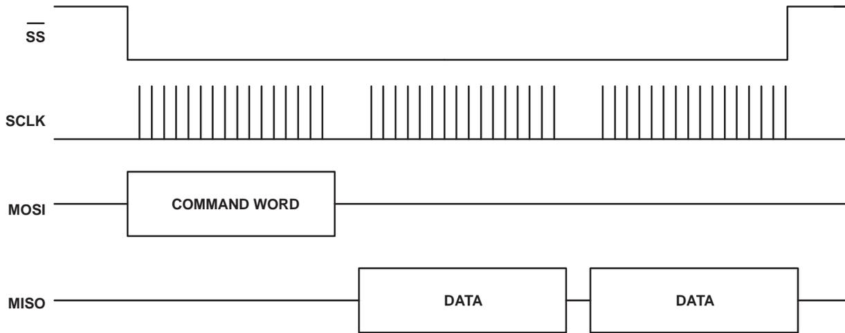
Figure 31. Read Operation for 'AIC26 SPI Interface
