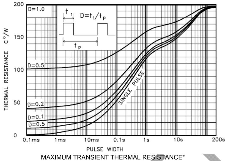
\* Reference above figure, devices were mounted on a 15mmx15mm ceramic substrate.
