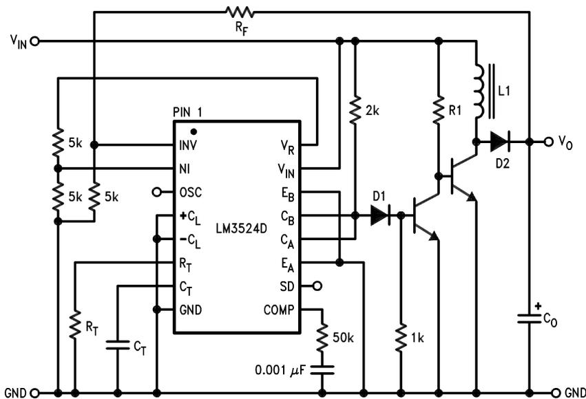
Figure 18. Positive Regulator, Step-Up Boosted Current Configuration
