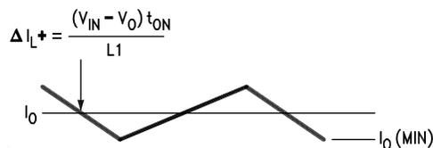
**Figure 24. Inductor Current Slope in Step-Down Regulator**
