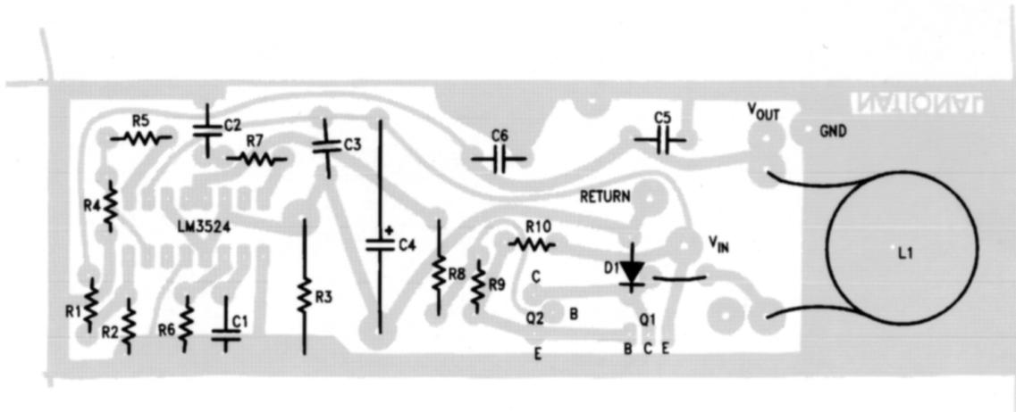
Figure 27. Stuffing Diagram, Component Side
