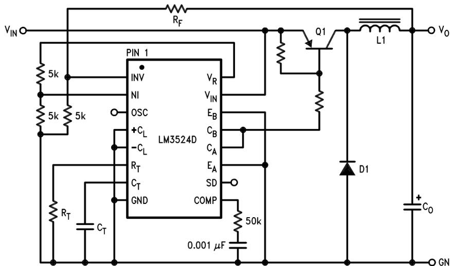
Figure 20. Positive Regulator, Step-Down Boosted Current Configuration
