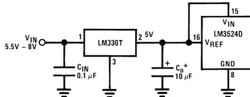
\*Minimum  $C_O$  of 10  $\mu\text{F}$  required for stability.
