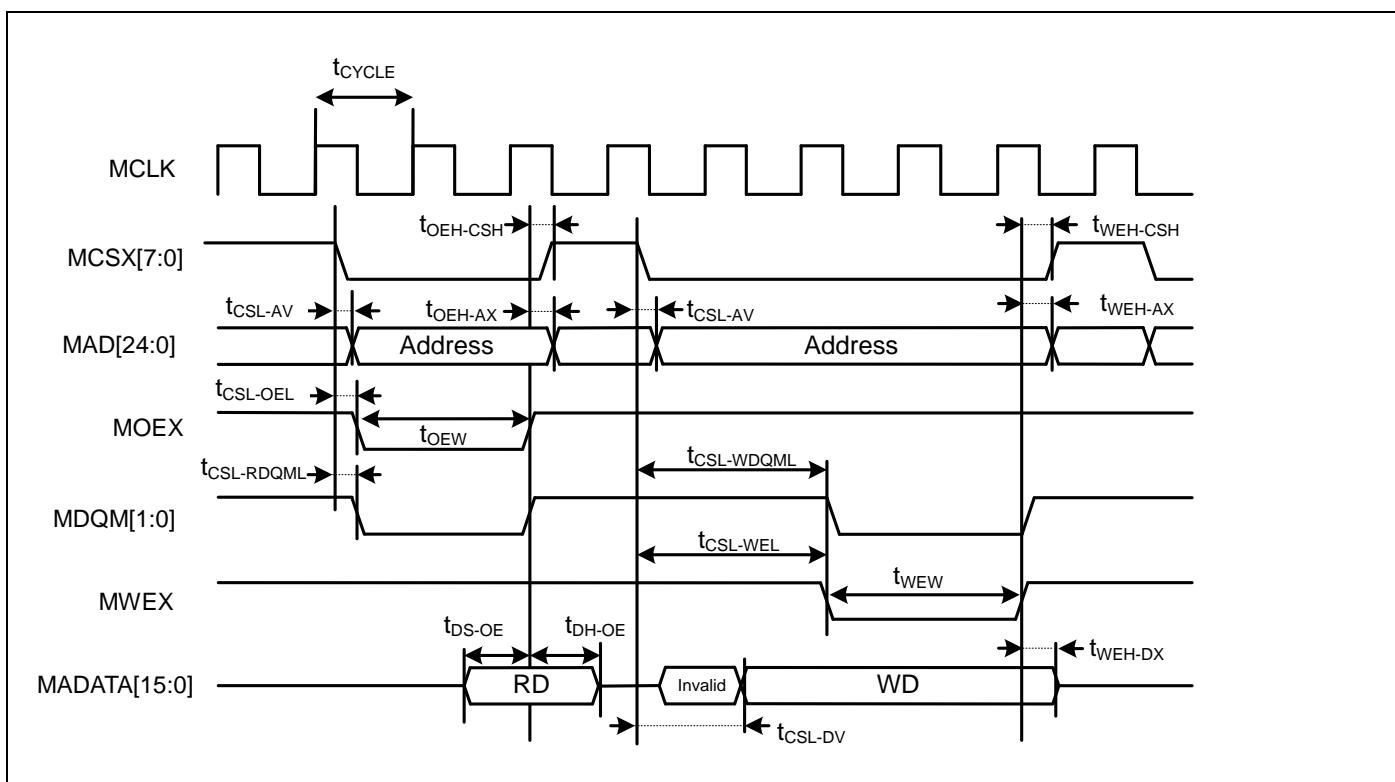
**Separate Bus Access Synchronous SRAM Mode**
