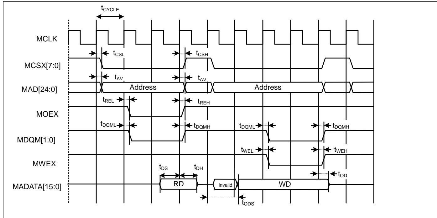
**Multiplexed Bus Access Asynchronous SRAM Mode**
