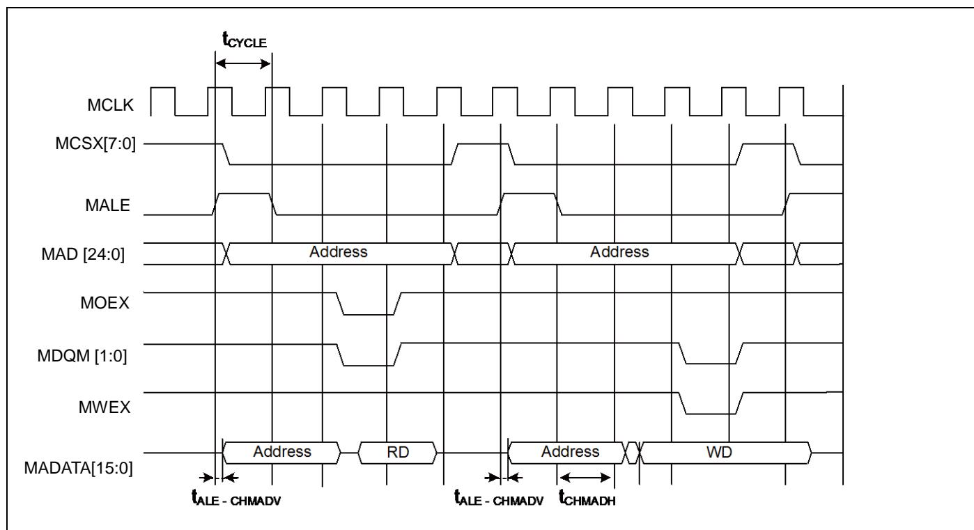
**Multiplexed Bus Access Synchronous SRAM Mode**
