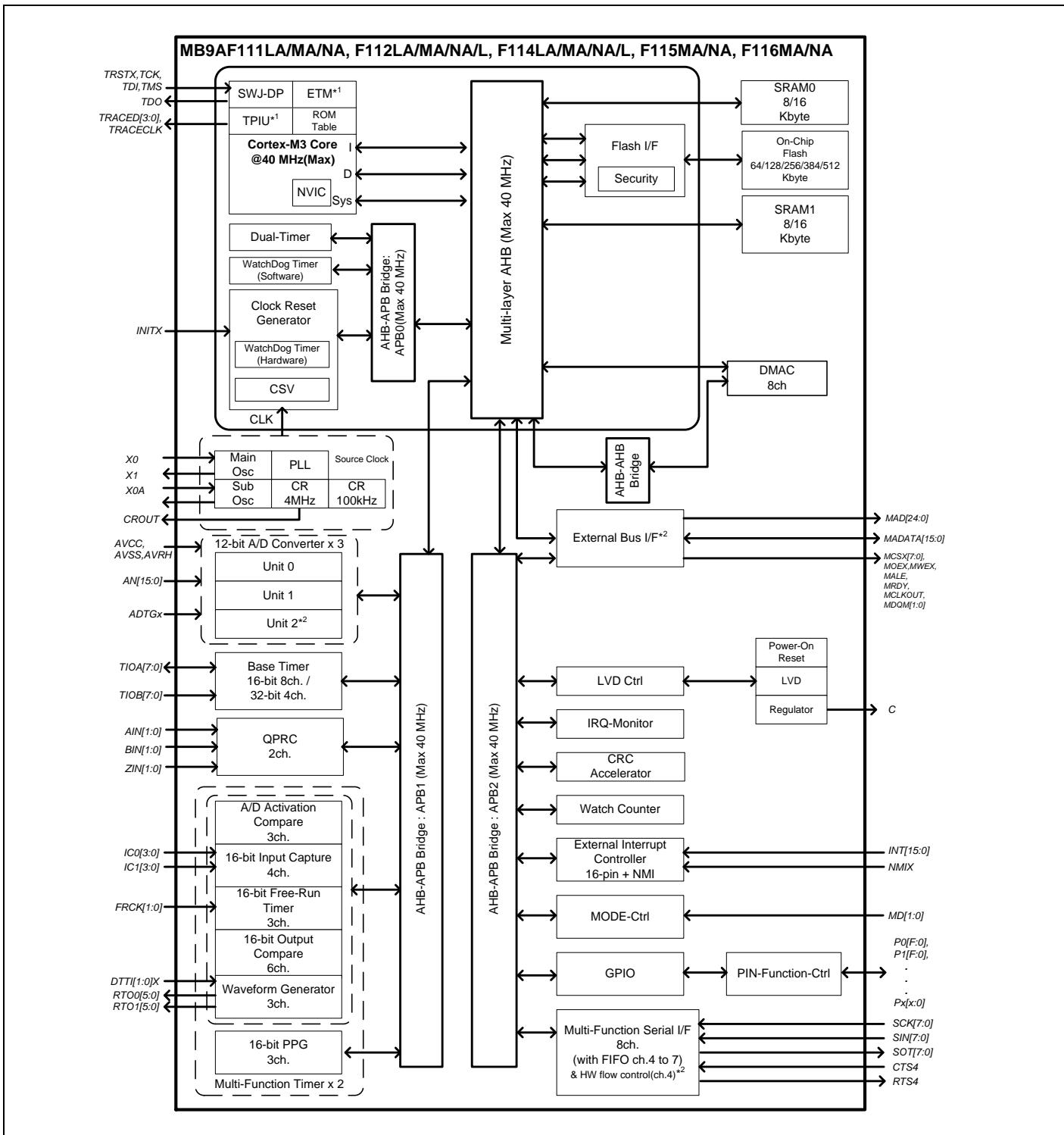
\*1: For the MB9AF111LA/MA, F112LA/MA, MB9AF114LA/MA, MB9AF115MA and MB9AF116MA, ETM is not available.
