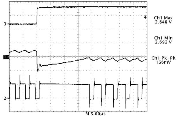
Trace 1– Regulator Output Voltage (100 mV/div.)
