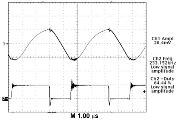
Trace 1– Regulator Output Voltage (10 mV/div.)
