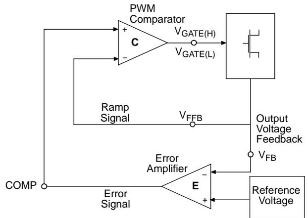
Figure 3. V<sup>2</sup> Control Diagram
