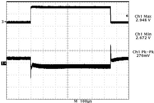
Trace 1– Regulator Output Voltage (100 mV/div.)
