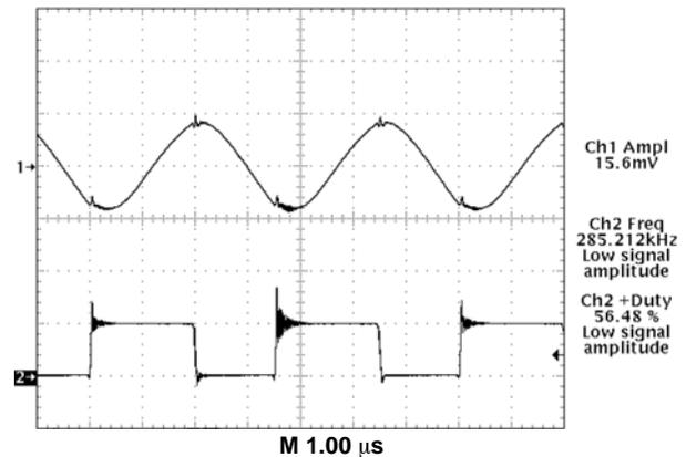
Trace 1– Regulator Output Voltage (10 mV/div.)
