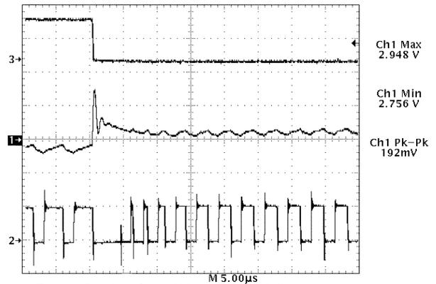
Trace 1– Regulator Output Voltage (100 mV/div.)
