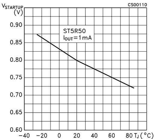
**Figure 21:** Start-up Voltage (V<sub>IN</sub> - V<sub>F</sub>) vs Temperature
