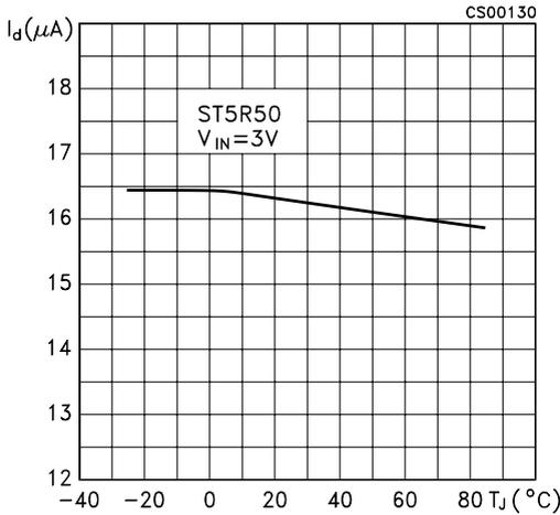
**Figure 31:** No Load Input Current vs Temperature
