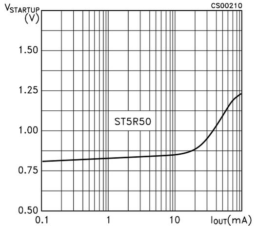
**Figure 23:** Start-up Voltage (V<sub>IN</sub> - V<sub>F</sub>) vs Output Current
