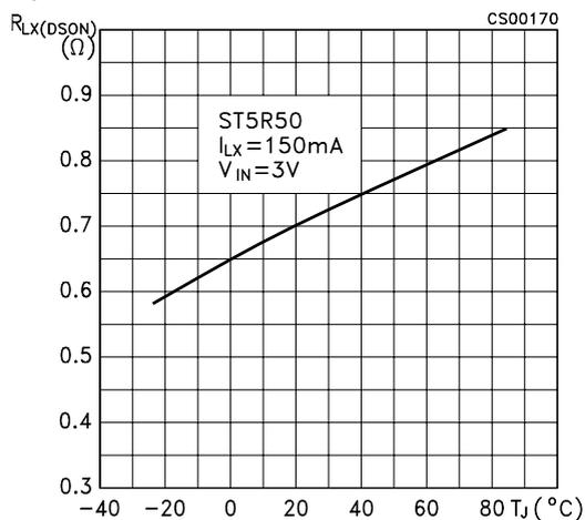
**Figure 27:** Internal Switch  $R_{DSON}$  vs Temperature
