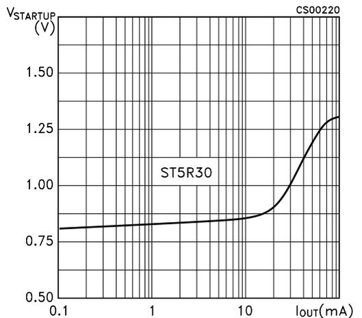
**Figure 24:** Minimum Input Voltage vs Output Current
