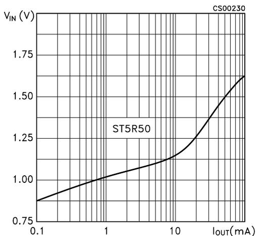
**Figure 25:** Minimum Input Voltage vs Output Current
