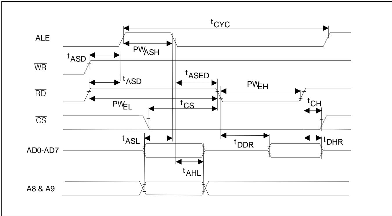
**Figure 38-2. Intel Bus Write Timing (BTS = 0 / MUX = 1)**
