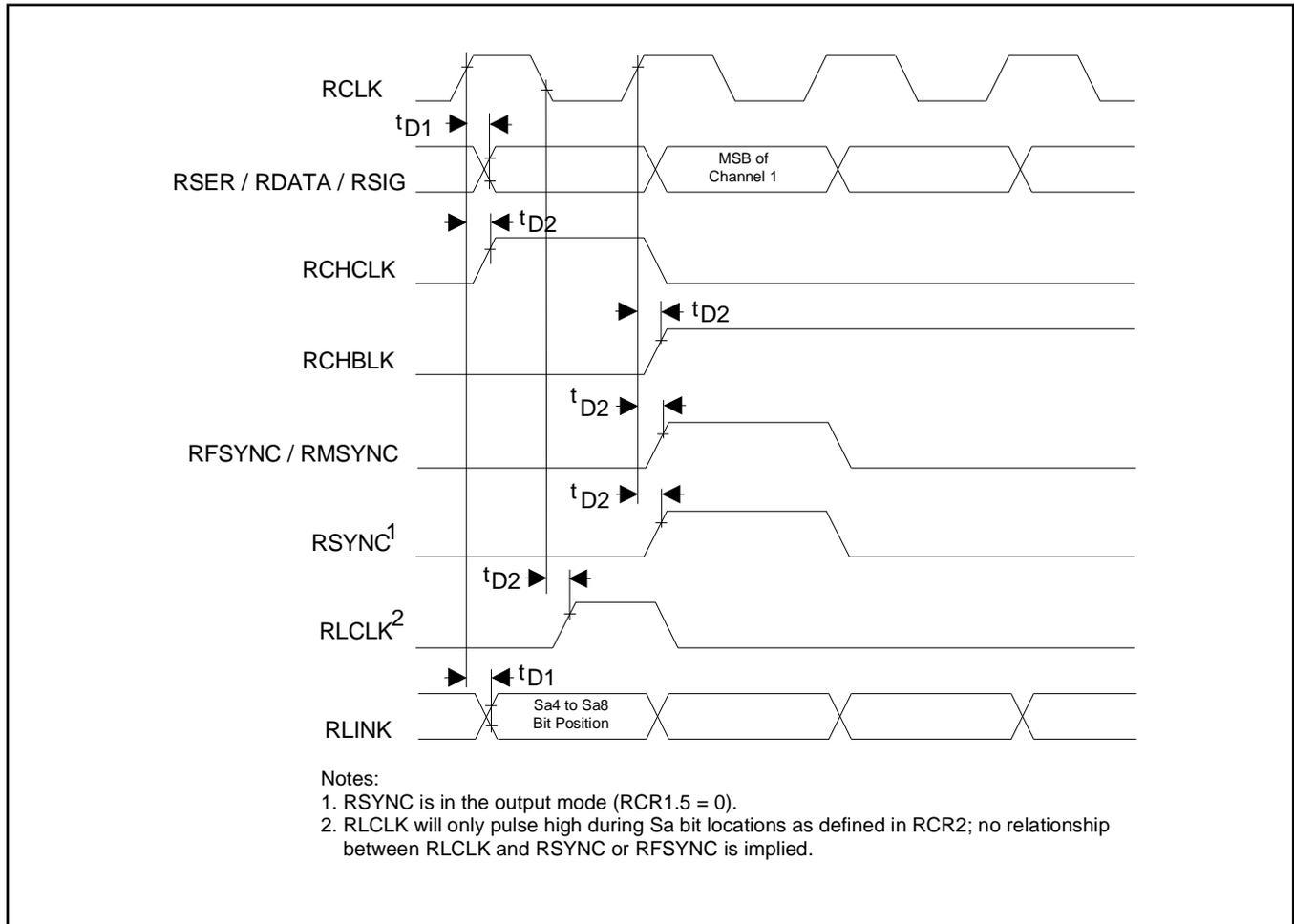
**Figure 38-10. Receive Side Timing, Elastic Store Enabled (T1 Mode)**
