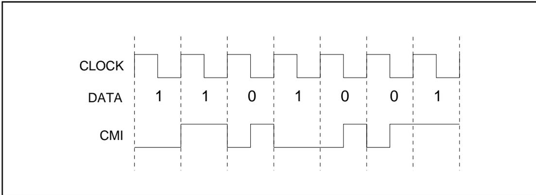
Transmit and receive CMI is enabled via LIC4.7. When this register bit is set, the TTIP pin will output CMI-coded data at normal levels. This signal can be used to directly drive an optical interface. When CMI is enabled, the user can also use HDB3/B8ZS coding. When this register bit is set, the RTIP pin will become a unipolar CMI input. The CMI signal will be processed to extract and align the clock with data.
