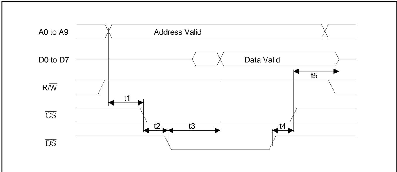
**Figure 38-7. Motorola Bus Write Timing (BTS = 1 / MUX = 0)**
