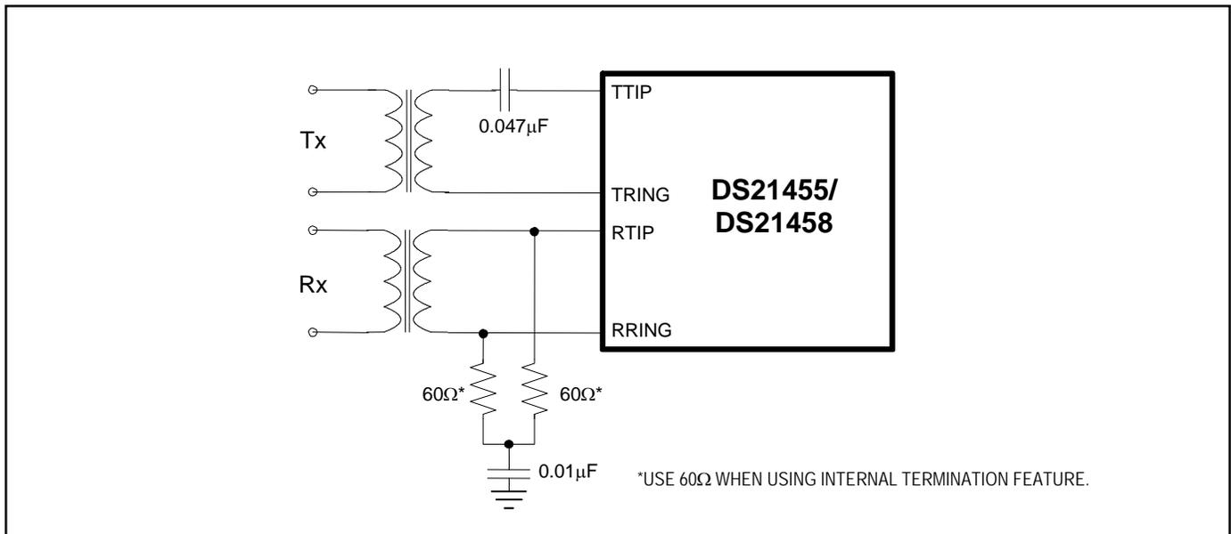
**Figure 25-2. Basic Unbalanced Network Connections**
