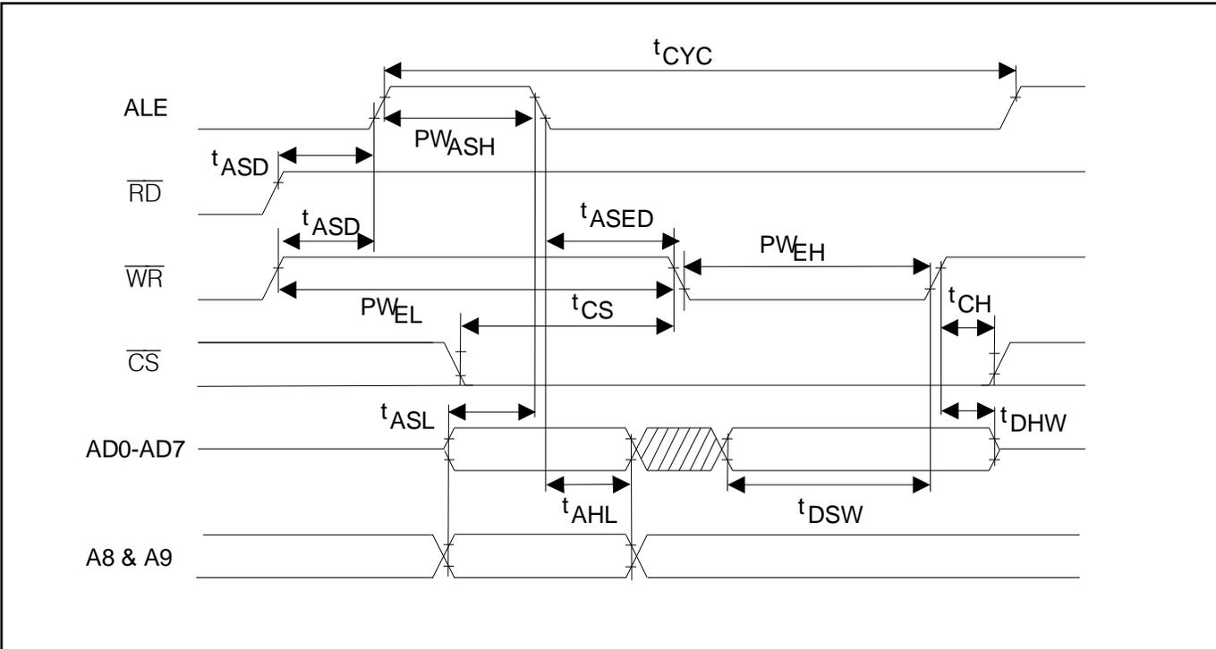
**Figure 38-3. Motorola Bus Timing (BTS = 1 / MUX = 1)**
