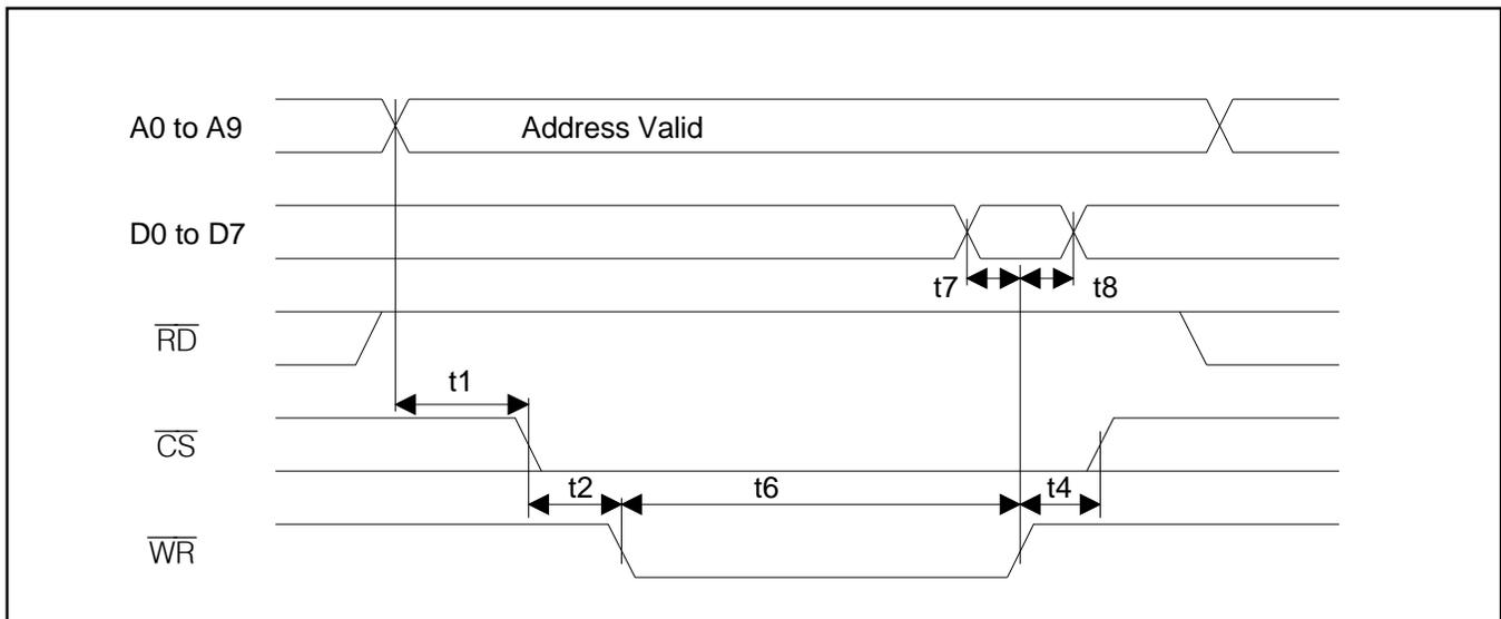
**Figure 38-6. Motorola Bus Read Timing (BTS = 1 / MUX = 0)**
