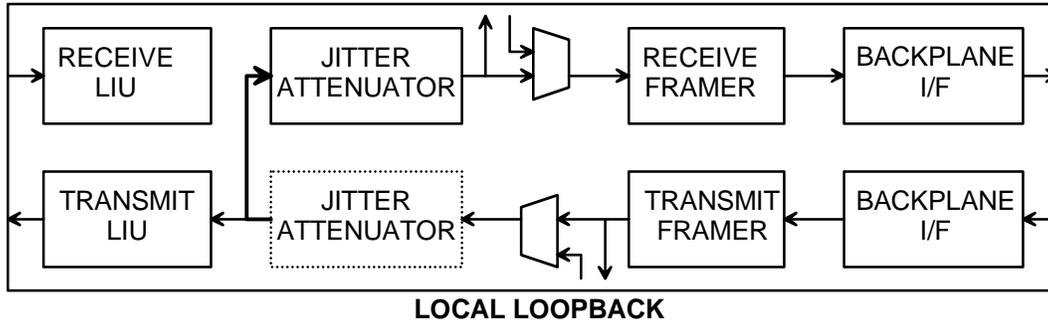
**Bit 4/Line Interface Unit Mux Control (LIUC).** This bit along with the LIUC/TPD pin and LBCR.7 controls the connection between the LIU and the Framer. See the LTS (LBCR.7) description below. When the LIUC/TPD pin is connected high or LBCR.7 = 1, the LIUC bit has control. When the LIUC/TPD pin is connected low the framer and LIU are separated and the LIUC bit has no effect. For the DS21458 this bit should always be set = 0.
