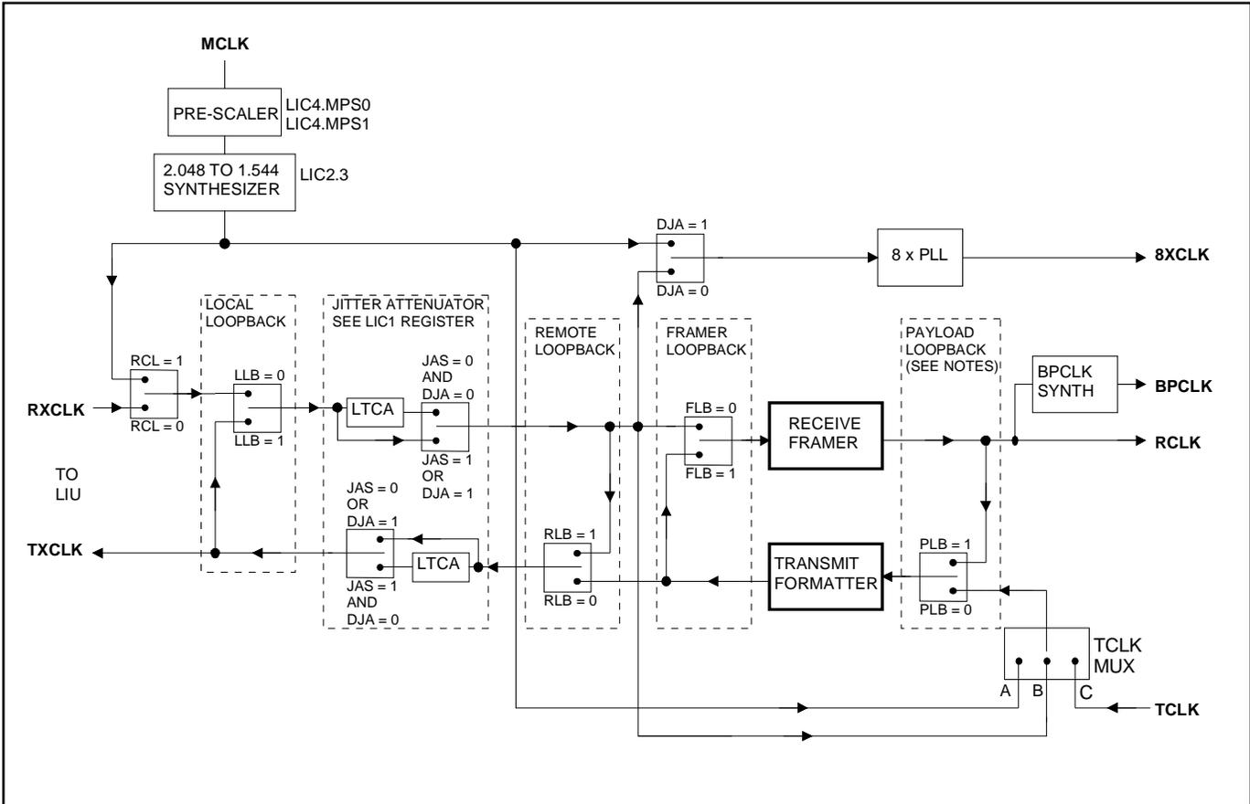
The TCLK MUX is dependent on the state of the TCSS0 and TCSS1 bits in the LIC1 register and the state of the TCLK pin.
