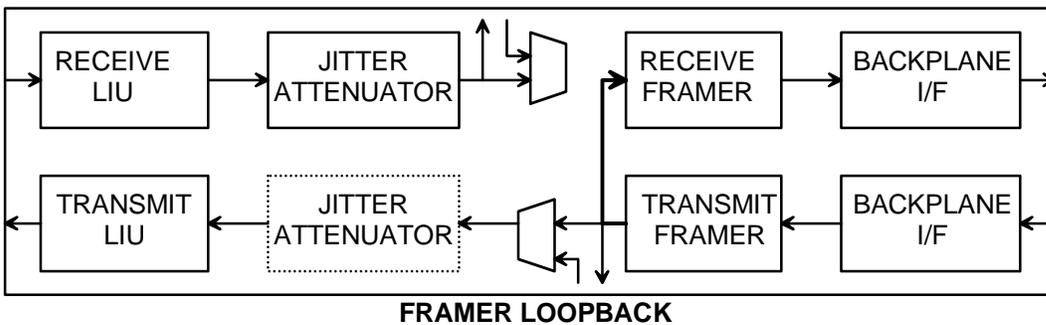
This loopback is useful in testing and debugging applications. In FLB, the device will loop data from the transmit side back to the receive side. When FLB is enabled, the following will occur:
