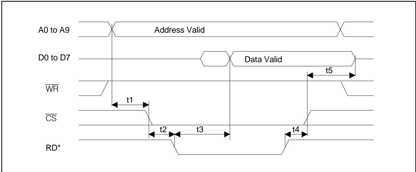
**Figure 38-5. Intel Bus Write Timing (BTS = 0 / MUX = 0)**
