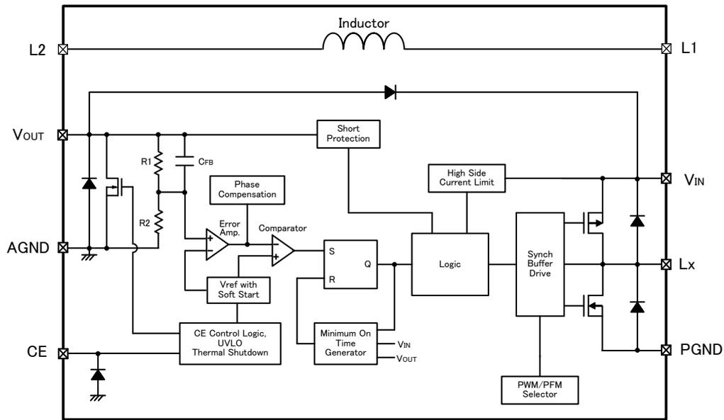
\* The XCL213 offers a fixed PWM control, a Control Logic of PWM/PFM Selector is fixed at "PWM" internally.
