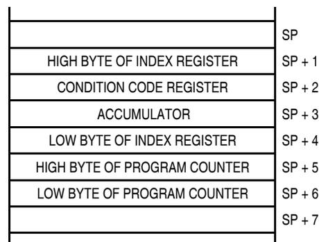
**Figure 18-16. Stack Pointer at Monitor Mode Entry**
