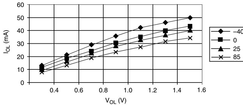
$V_{OL} < 1.0 \text{ V} @ I_{OL} = 15 \text{ mA}$
