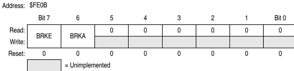
**Figure 18-4. Break Status and Control Register (BRKSCR)**
