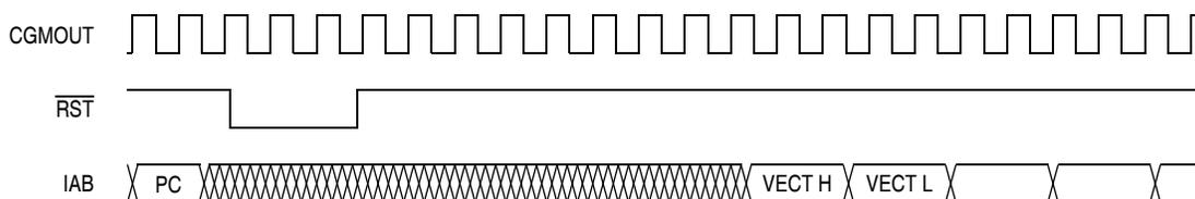
Figure 14-4. External Reset Timing
