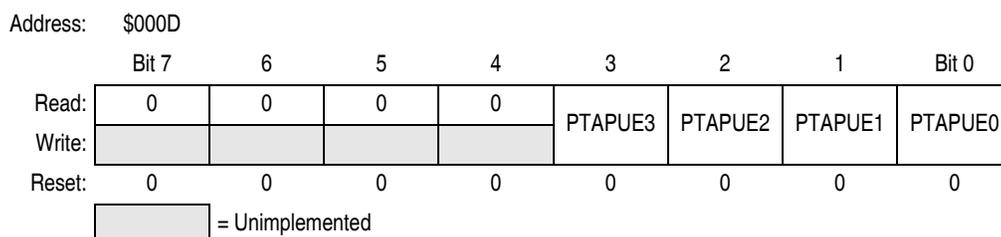
**Figure 12-5. Port A Input Pullup Enable Register (PTAPUE)**
