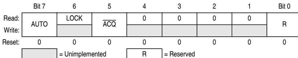
**Figure 4-5. PLL Bandwidth Control Register (PBWC)**
