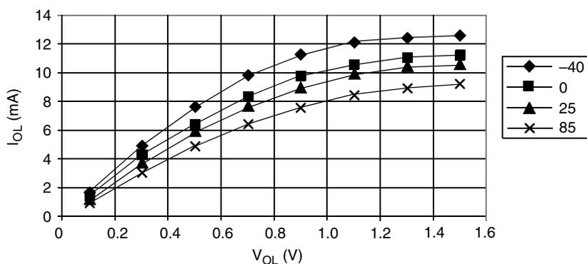
$V_{OL} < 0.3 \text{ V} @ I_{OL} = 0.5 \text{ mA}$
