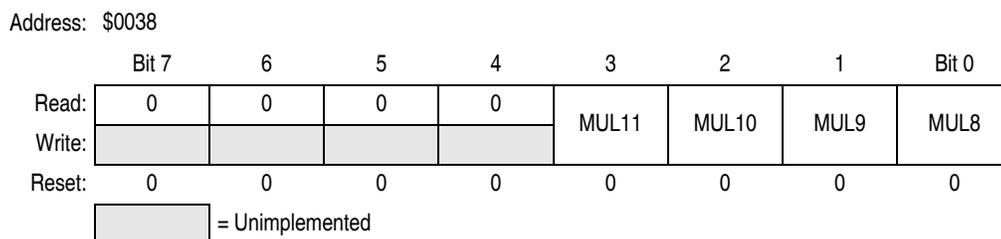
**Figure 4-6. PLL Multiplier Select Register High (PMSH)**
