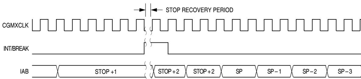
**Figure 14-19. Stop Mode Recovery from Interrupt**
