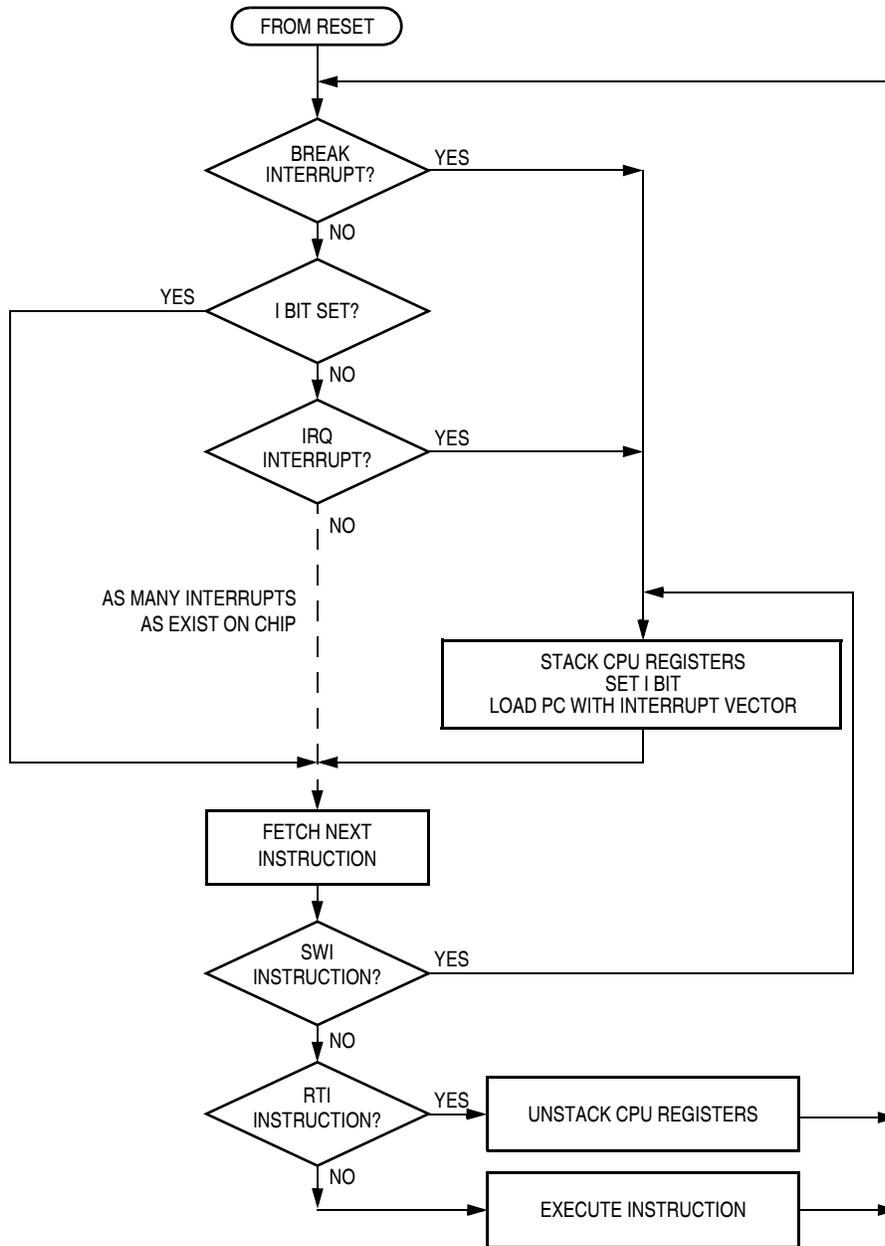
**Figure 14-10. Interrupt Processing**
