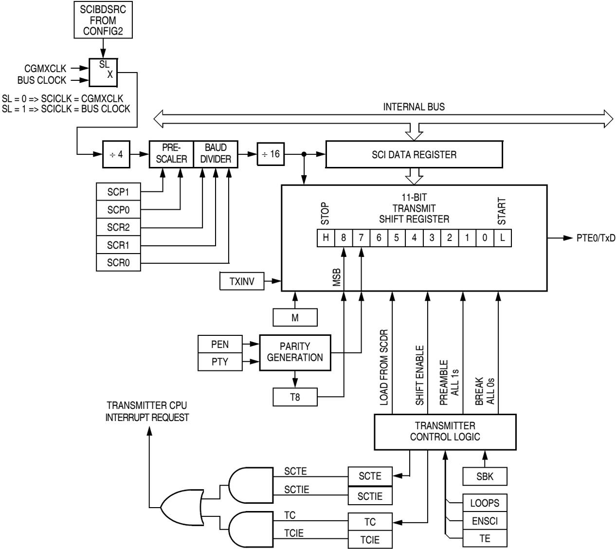
Figure 13-5. SCI Transmitter
