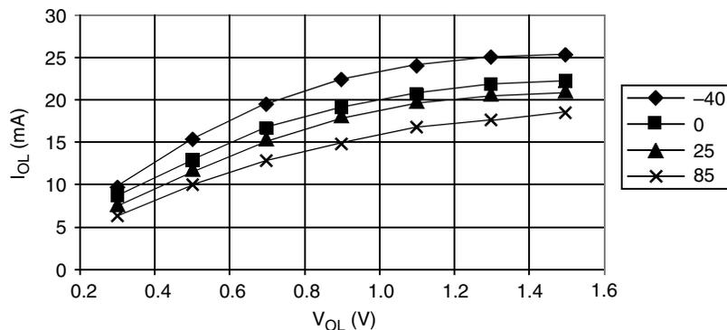
$V_{OL} < 0.8 \text{ V} @ I_{OL} = 10 \text{ mA}$
