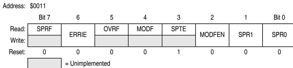
**Figure 15-15. SPI Status and Control Register (SPSCR)**
