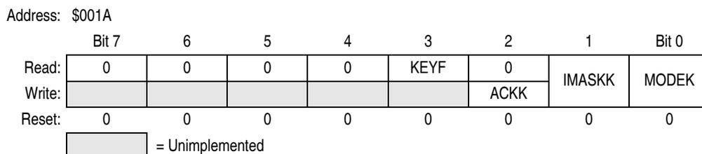
**Figure 9-4. Keyboard Status and Control Register (INTKBSCR)**
