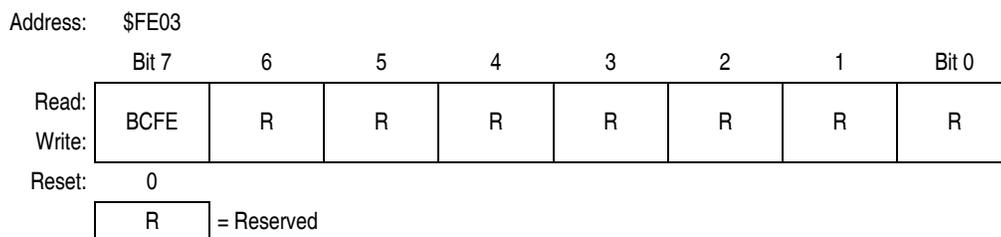
**Figure 14-22. SIM Break Flag Control Register (BFCR)**
