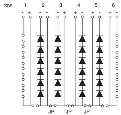
Assembled with all jumpers. Jumpers can be removed according driver design
