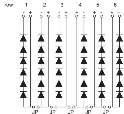
Assembled with all jumpers. Jumpers can be removed according driver design
