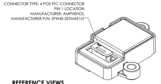
ALWAYS LIFT CONNECTOR SLIDER LATCH VERTICALLY TO THE OPEN POSITION WHEN INSERTING OR EXTRACTING A CABLE TO AVOID CONNECTOR AND CABLE CONTACT DAMAGE. MUST CLOSE THE SLIDER LATCH TO MAKE A PERMANENT CONNECTION TO THE CABLE. AVOID LATERAL LOADING OF THE CONNECTOR.
