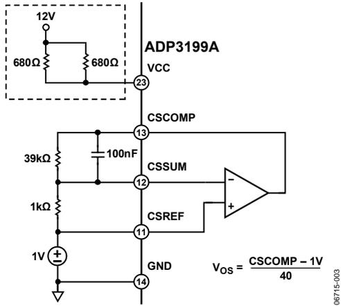
Figure 5. Current Sense Amplifier Offset Voltage ( $V_{OS}$ )
