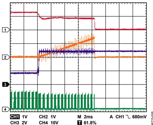
Figure 9. Overcurrent Latch-Off Waveforms
