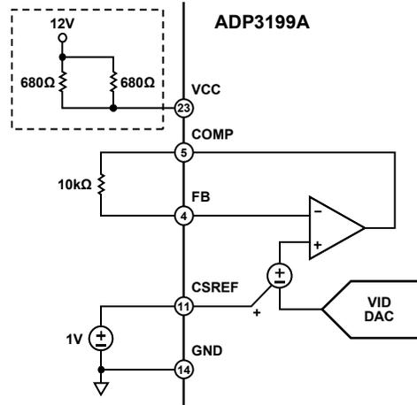
Figure 6. Positioning Voltage
