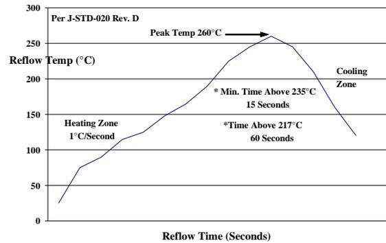
**Figure 37. Recommended linear reflow profile using Sn/Ag/Cu solder.**
