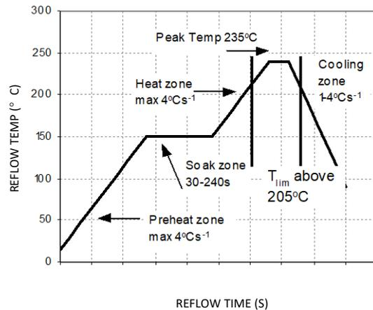
Figure 35. Reflow Profile for Tin/Lead (Sn/Pb) process.
