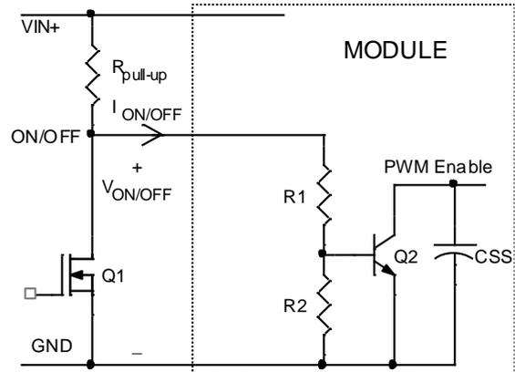
Figure 29. Circuit configuration for using negative logic On/Off.
