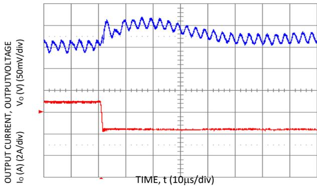
**Figure 13. Transient Response to Dynamic Load Change from 100% of full load (Vo = 3.3Vdc, Cext = 2x150 µF Polymer Capacitors).**
