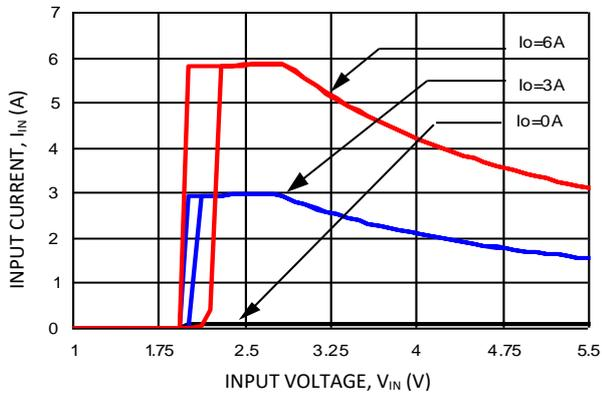
**Figure 7. Input voltage vs. Input Current**
