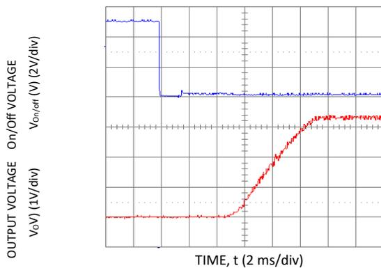
**Figure 15. Typical Start-Up Using Remote On/Off with Low-ESR external capacitors (7x150uF Polymer) (Vin = 5.0Vdc, Vo = 3.3Vdc, Io = 6A, Co = 1050µF).**
