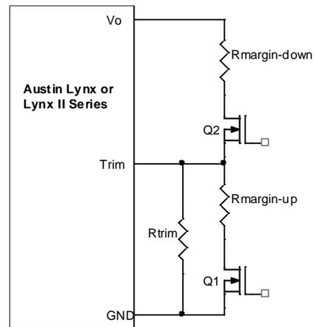
Figure 31. Circuit Configuration for margining Output voltage.
