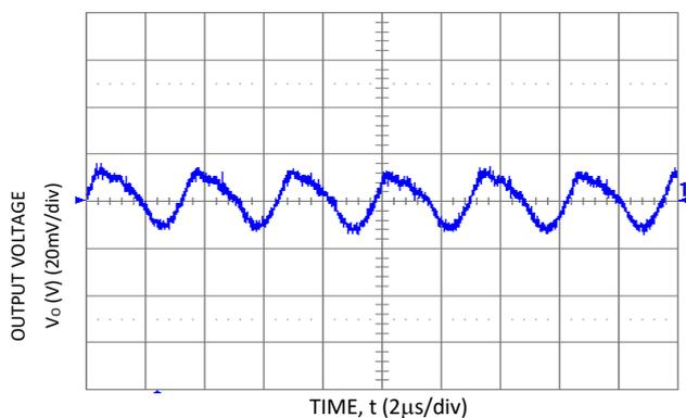
**Figure 9. Typical Output Ripple and Noise**
