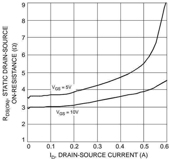
Fig. 3 On-Resistance vs. Drain Current & Gate Voltage
