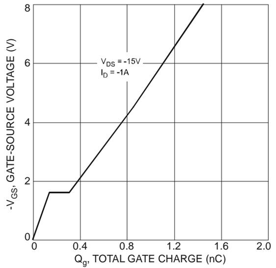
Fig. 14 Gate-Charge Characteristics
