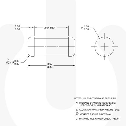
Figure 11. 2-TERMINAL, SOD-80, JEDEC DO-213AC, MINI-MELF
