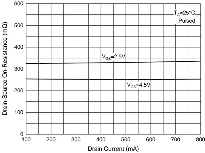
Fig. 4 -  $R_{DS(ON)} - V_{GS}$
