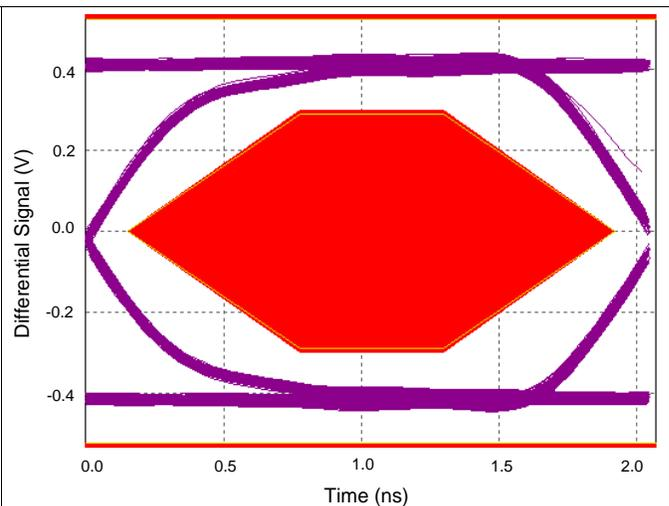
Figure 19. High Speed Eye Diagram Without TS5USBC400
