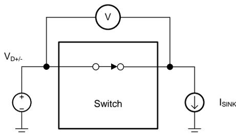
Channel ON,  $R_{ON} = V/I_{SINK}$
