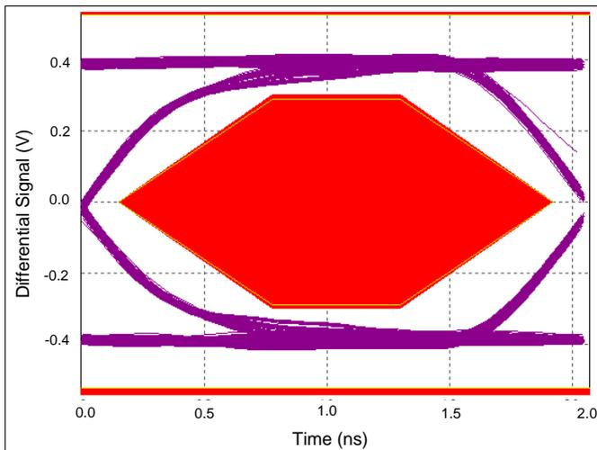
Figure 18. High Speed Eye Diagram With TS5USBC400
