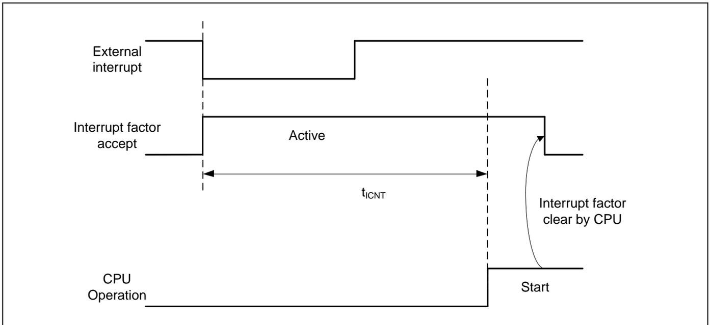
\*: External interrupt is set to detecting fall edge.
