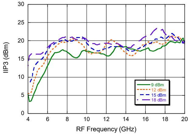
**IIP3 over Temperature @  $P_{LO} = 15$  dBm,  $I_F = 100$  MHz**
