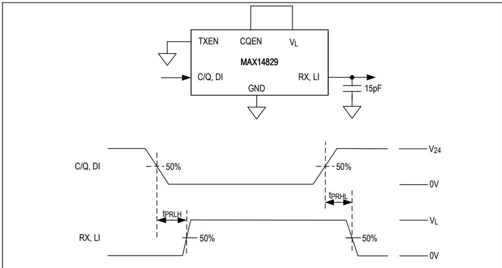
Figure 4. C/Q and DI Receiver Propagation Delays
