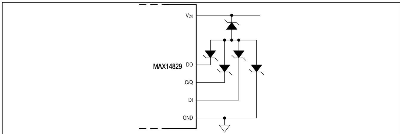
Figure 6. MAX14829 Operating Circuit with TVS Protection
