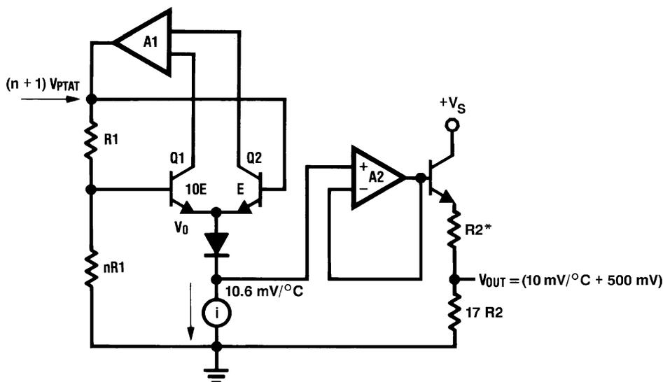
\*R2  $\approx$  2k with a typical 1300-ppm/ $^{\circ}\text{C}$  drift.
