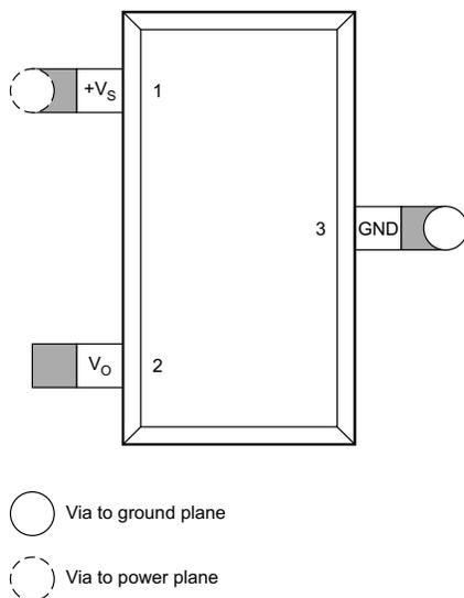
**Figure 19. PCB Layout**
