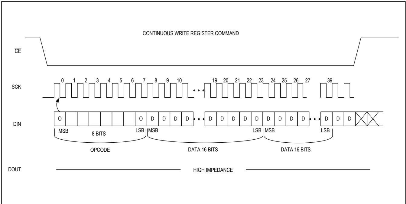
Figure 21. Continuous Write Register Opcode Command Protocol
