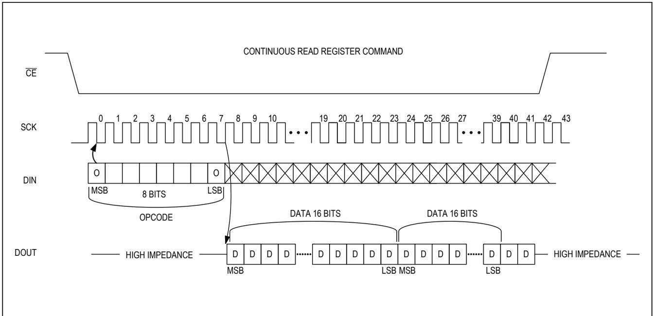
Figure 19. Continuous Read Register Opcode Command Protocol
