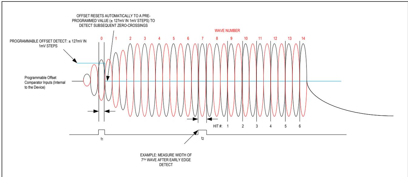
Figure 5B. Early Edge Detect Received Wave Example
